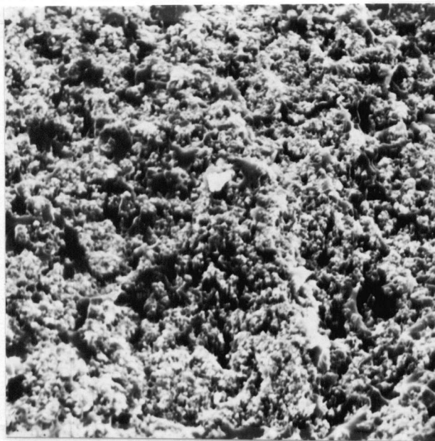
( d ). 20.0 vol% fine nickel magnification = 800
