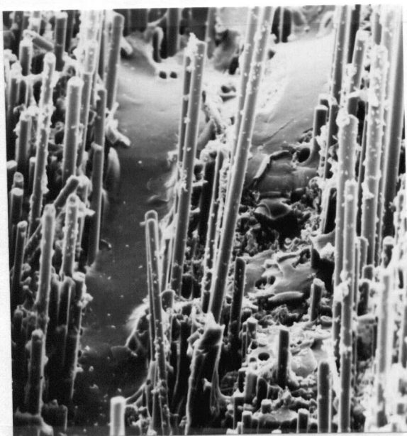
( b ). 2.5 vol% iron plus 24.2 vol% Glass magnification = 200
