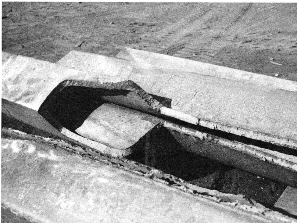
Fig. (50). Bulged strand from Western Canada Steel (Weybridge mold), showing the part of the web that has separated.
