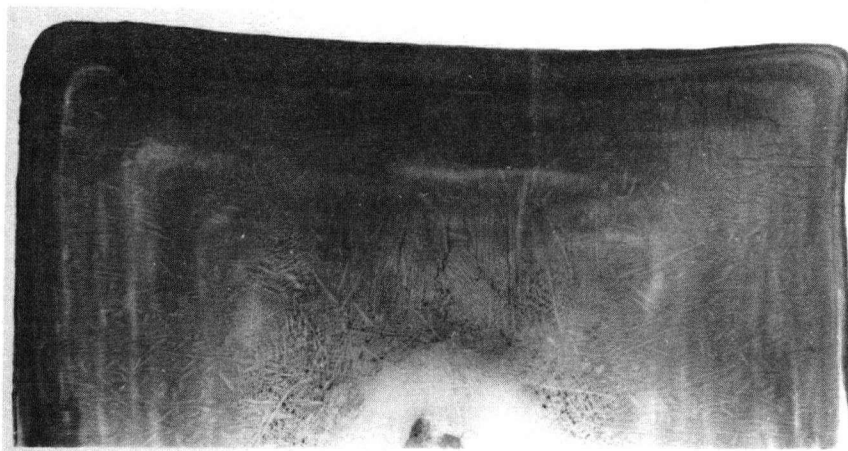
Fig. (34). Transverse section from billet section 2 1 . 0.75 x
