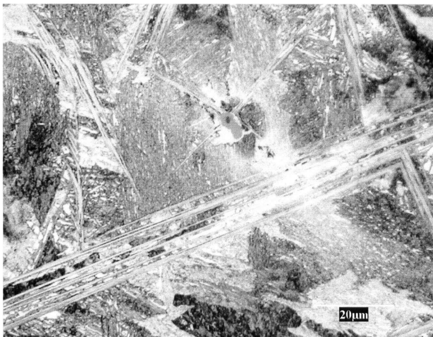
Figure 4.33 Nucleation of carbide plates at an inclusion in DSC sample 13
