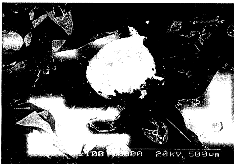
Fig. 6 — Another white bead in Cominco tail slag (SEM, magnification 100, accelerating voltage 20kV)
