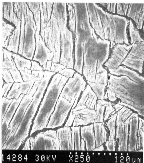
Figure 8.14 Electron back-scatter micrographs of an iron-doped (4.4wt% iron) synthetic copper matte and of a pure synthetic copper matte obtained after total-bed polarization showing particle fracturing.
