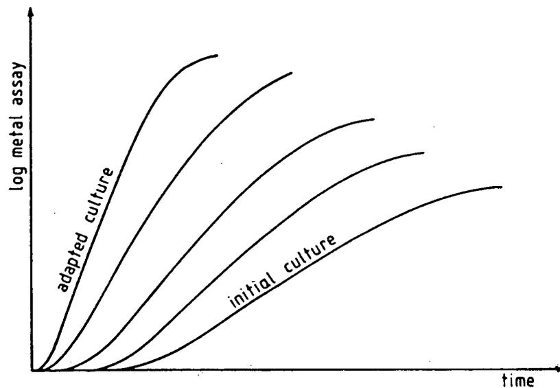
Figure 3.8 : Effect of repeated inoculation of initially non-acclimatized bacteria into the same environment (after Rossi [16]).
