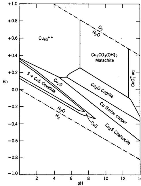
Figure 3.2 : Standard E<sub>h</sub>-pH diagram of system Cu-H<sub>2</sub>O-O<sub>2</sub>-S-CO<sub>2</sub>, 25°C and 1 atm. total pressure, presenting the stability of some copper minerals in supergene enrichment deposits (after Klein & Hurlbut [27]).
