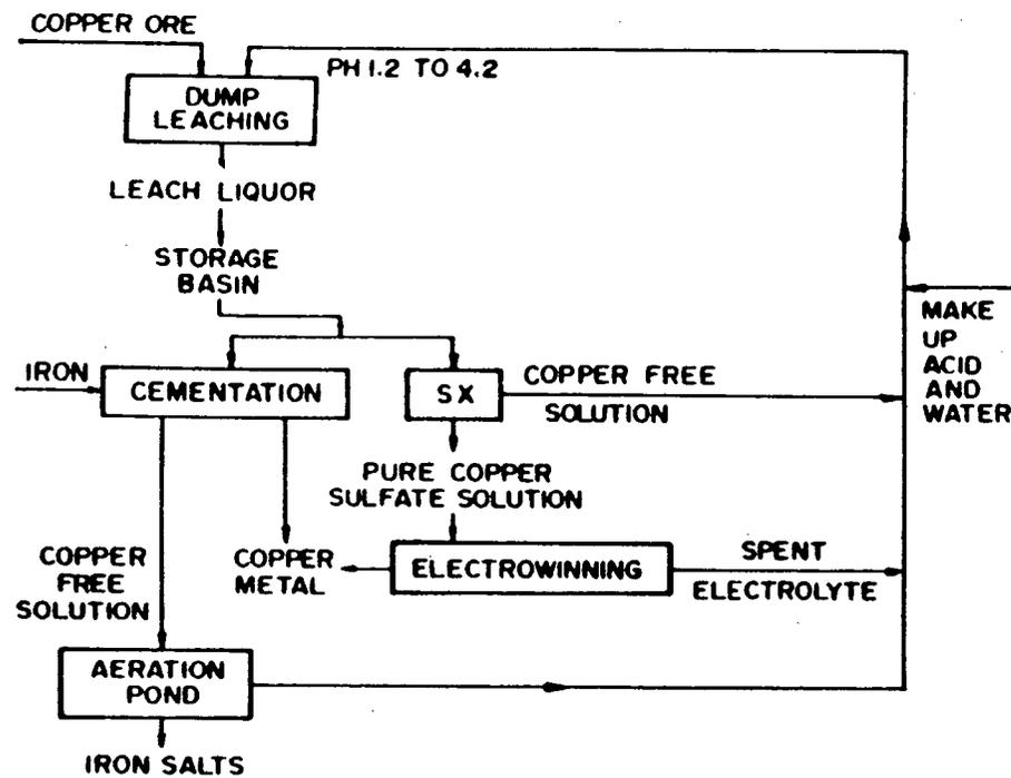
Figure 3.3 : Generalized flowsheet illustrating dump, heap, thin-layer, or *in-situ* leaching (after Gupta & Mukherjee [10]).
