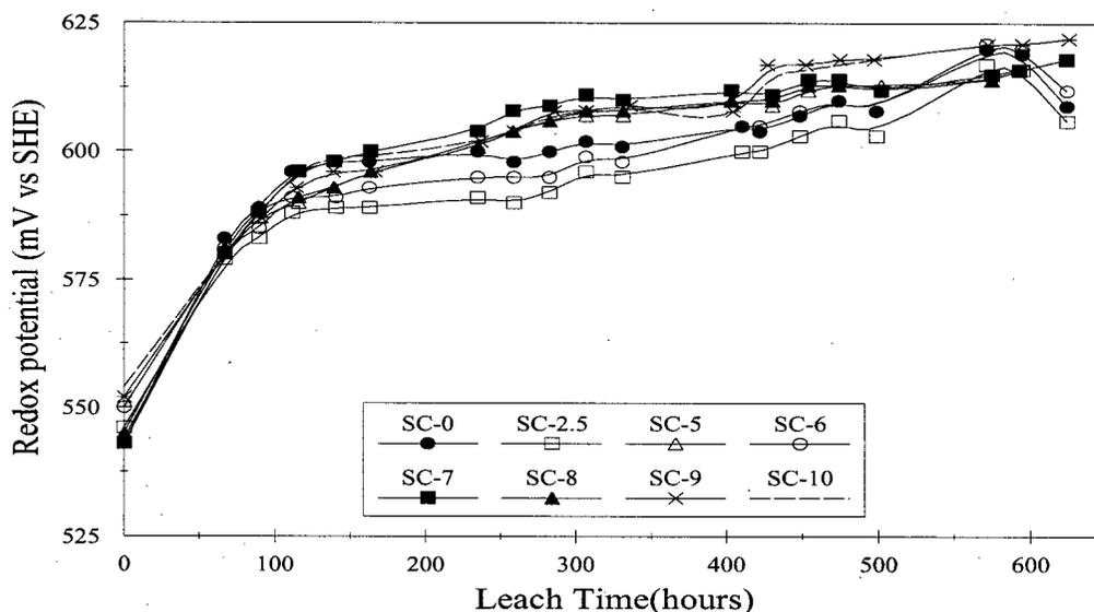
Figure 5.12 : Redox potential ( $E_h$ ) vs. time plots for all sterile tests, Zaldívar (Cl) series (Zaldívar ore, 9 g/L  $Fe^{2+}$ , variable  $Cl^-$  level).
