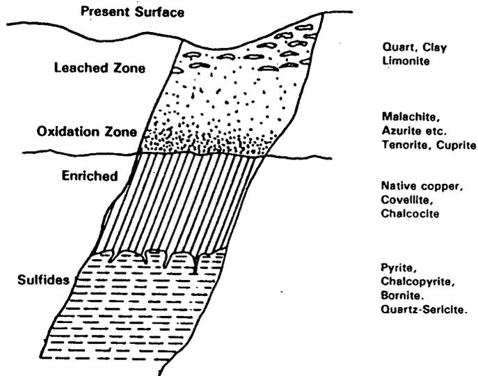
Figure 3.1 : Vertical section of upper portion of copper ore deposit illustrating zonation, water table, and typical copper minerals (after Bartlett [26]).
