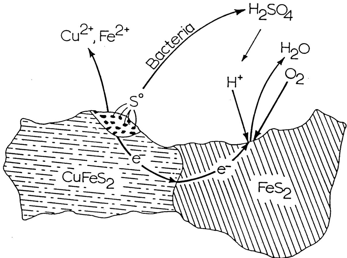
Figure 3.16 : Illustration of bacterially enhanced galvanic leaching mechanism between pyrite and chalcopyrite (after Murr [11]).
