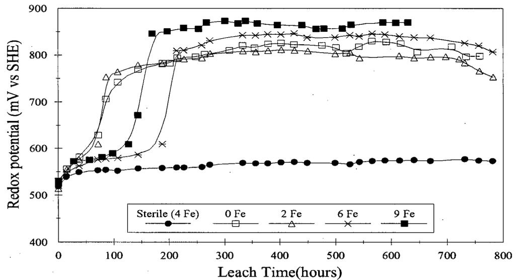
Figure 5.3 : Redox potential ( $E_h$ ) vs time plots of selected bioleach tests and a sterile test (4 g/L Fe<sup>2+</sup>) from Set 1, Lower (Fe) series (Lower ore, 2.5 g/L Cl<sup>-</sup>, variable Fe<sup>2+</sup> level).
