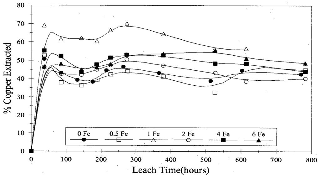
Figure 5.4 : Copper extraction vs. time plots for all sterile tests, Lower (Fe) series (Lower ore, 2.5 g/L Cl<sup>-</sup>, variable Fe<sup>2+</sup> level).
