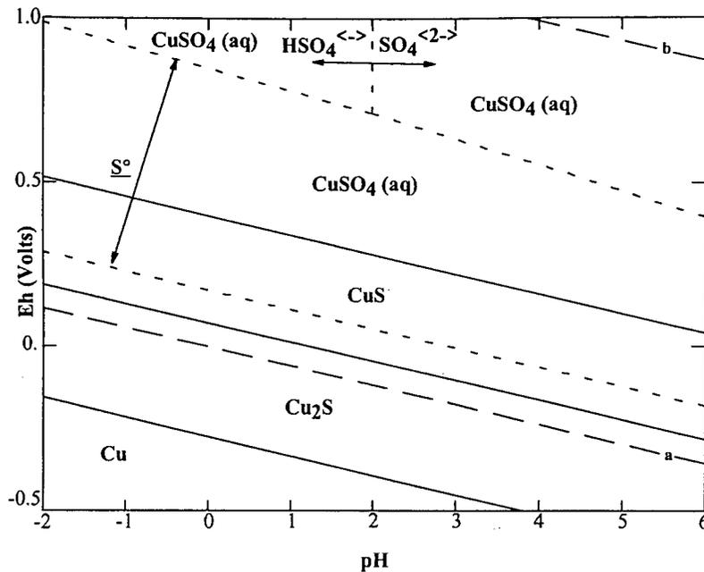
Figure 3.13 :  $E_h$ -pH diagram for the Cu-S-Cl- $H_2O$  system at 25°C, [S, Cu, Cl] solute species = 1 M,  $P(H_2S(g))=1$  atm. with extended sulfur stability realized by destabilizing the sulfate/sulfur equilibrium line by 300 kJ/mol.
