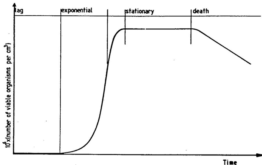
Figure 3.7 : Characteristic bacterial growth curve under laboratory (batch) conditions (after Rossi [16]).
