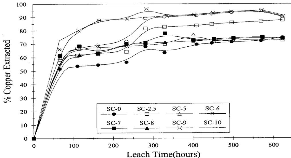
Figure 5.14 : Copper extraction vs. time plots for all sterile tests, Zaldívar (Cl) series (Zaldívar ore, 9 g/L  $\text{Fe}^{2+}$ , variable  $\text{Cl}^-$  level). (Legend: SC means sterile control, # is chloride concentration in g/L).
