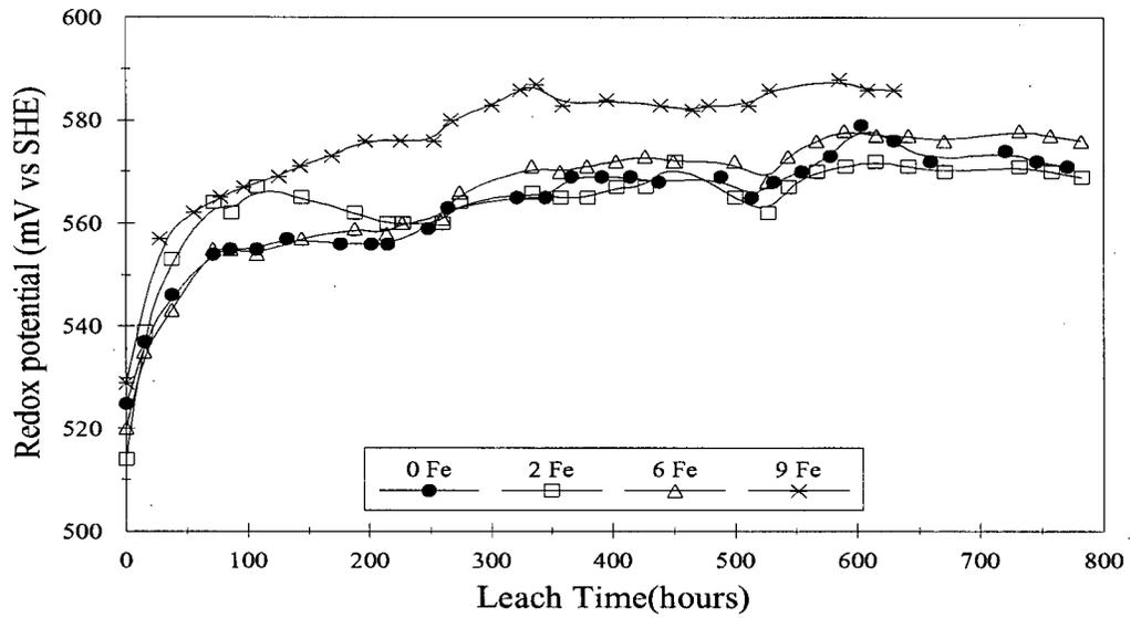
Figure 5.2: Redox potential ( $E_h$ ) vs. time plots of selected sterile leaches of Lower (Fe) series (Lower ore, 2.5 g/L Cl<sup>-</sup>, variable Fe<sup>2+</sup> level).
