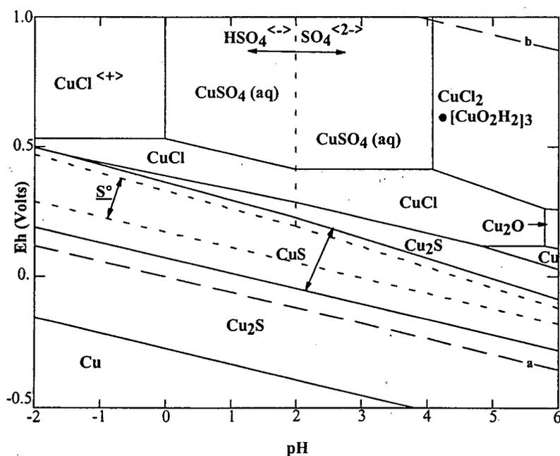
Figure 3.12 : E<sub>h</sub>-pH diagram for the Cu-S-Cl-H<sub>2</sub>O system at 25°C, [S, Cu, Cl] solute species = 1 M, P(H<sub>2</sub>S(g))=1 atm. under standard conditions.
