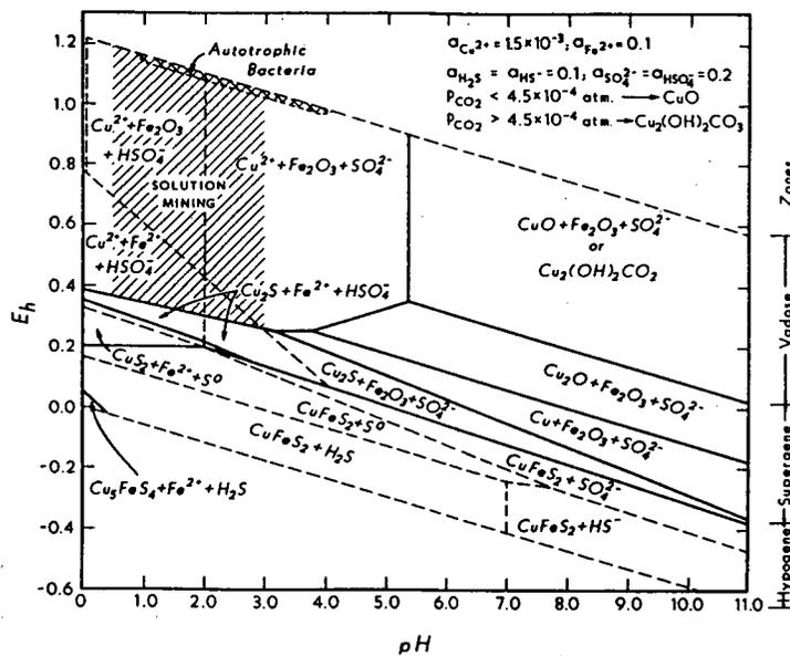
Figure 3.15 : E<sub>h</sub>-pH diagram for the Cu-Fe-S-H<sub>2</sub>O system illustrating zoning, solution mining region, and regime of bacterial activity (after Wadsworth and Miller [107]).
