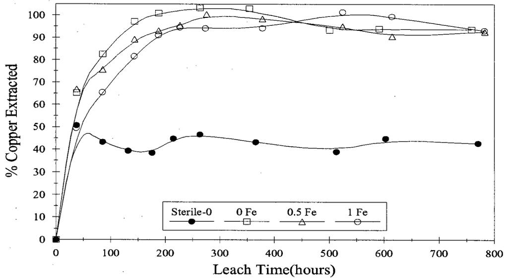
Figure 5.5 : Copper extraction vs. time plots for selected bioleach tests and a sterile test (0 g/L Fe<sup>2+</sup>), set 1, Lower (Fe) series (Lower ore, 2.5 g/L Cl<sup>-</sup>, variable Fe<sup>2+</sup> level).
