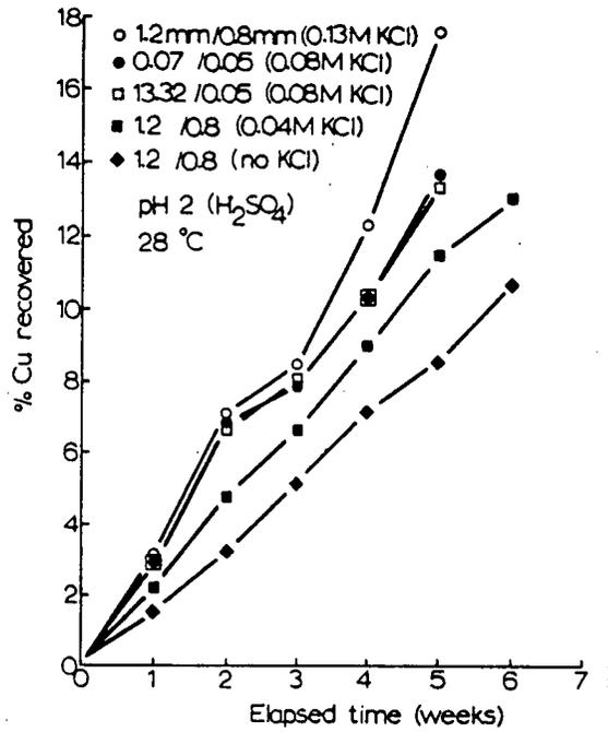
Figure 3.17 : KCl column leaching with Phelps-Dodge copper-bearing waste; the effect of particle size and KCl concentration (after Murr *et al.* [147]).
