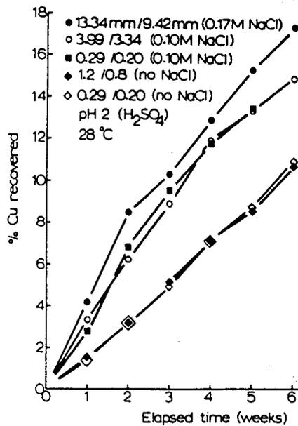
Figure 3.18 : NaCl column leaching with Phelps-Dodge copper-bearing waste; the effect of particle size and NaCl concentration (after Murr *et al.* [147]).
