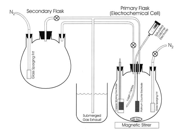
Figure 7 Electrochemical cell apparatus
