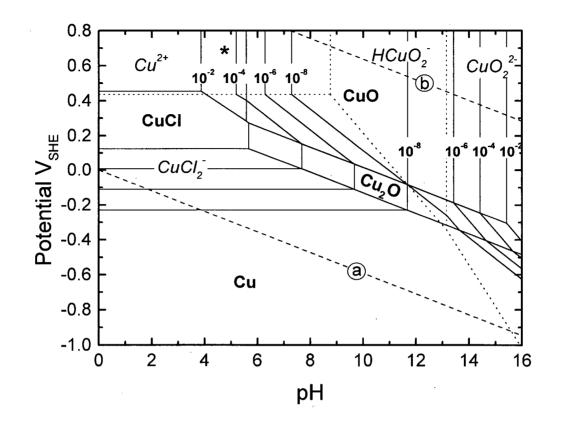
Figure 16 Potential-pH equilibria for the Cu-Cl<sup>-</sup>-H<sub>2</sub>O system
