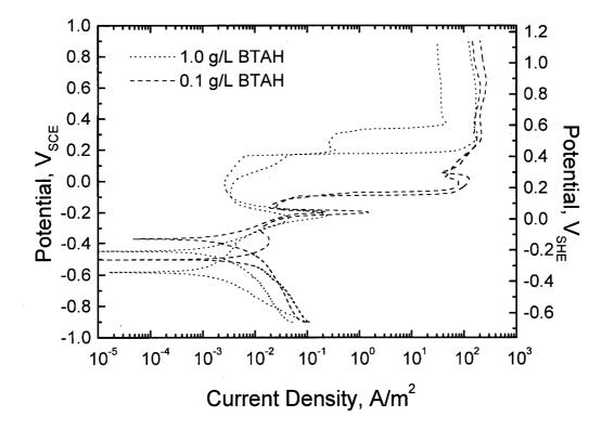
Figure 12 Polarisation scans in 1M NaCl containing 1.000 or 0.100 g/l BTAH. Scan rate = 1.0 mV/s
