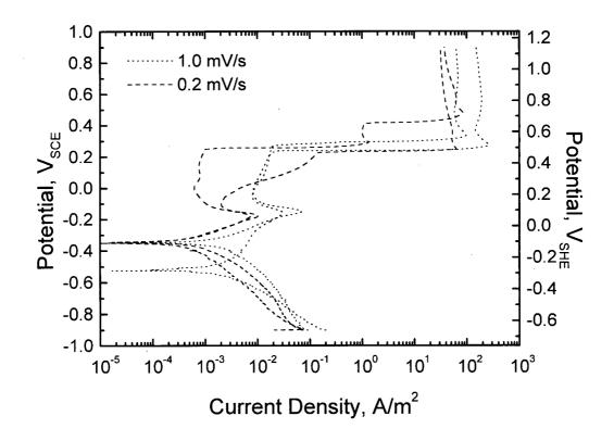
Figure 11 Polarisation scans in 1M NaCl containing 1.114 g/l TTAH
