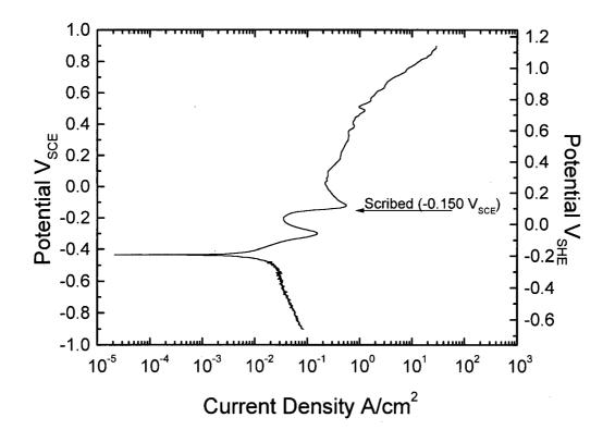
Figure 20 Scribing test on Cu in 1M NaBr containing 1.0 g/l BTAH at pH 6.0. Surface scribed at -0.150  $V_{SCE}$
