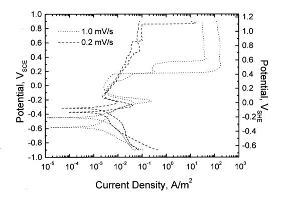
Figure 10 Polarisation scans in 1M NaCl containing 1.000 g/l BTAH
