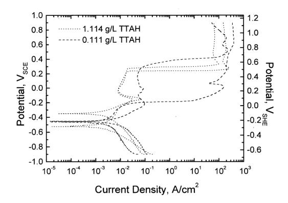
Figure 13 Polarisation scans in 1M NaCl containing 1.114 or 0.111 g/l TTAH. Scan rate = 1.0 mV/s
