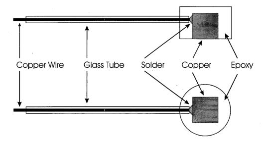
Figure 6 Schematic of the working electrode assembly
