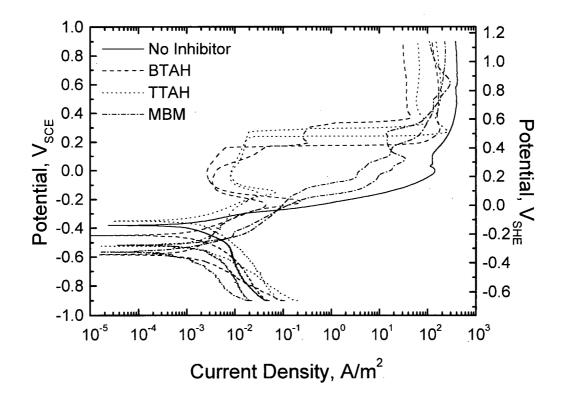
Figure 9 Polarisation scans with no inhibitor, BTAH, TTAH or MBM in 1M NaCl. Scan rate = 1.0 mV/s
