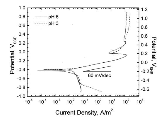
Figure 17 Polarisation behaviour of Cu in 1M NaBr at pH 6.5 and 3.0. Triangular insert shows a slope of 60 mV per decade in current density
