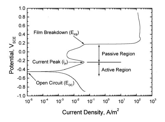
Figure 8 Sample polarisation scan with major features labelled
