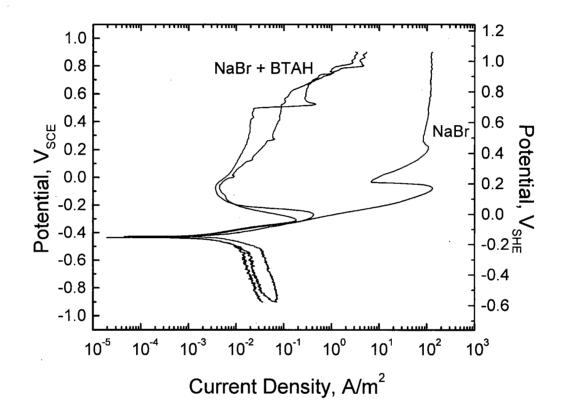
Figure 18 Polarisation behaviour of Cu in 1M NaBr containing 1.0 g/l BTAH at pH 6.0. Behaviour compared with as prepared 1M NaBr (pH 6.5)
