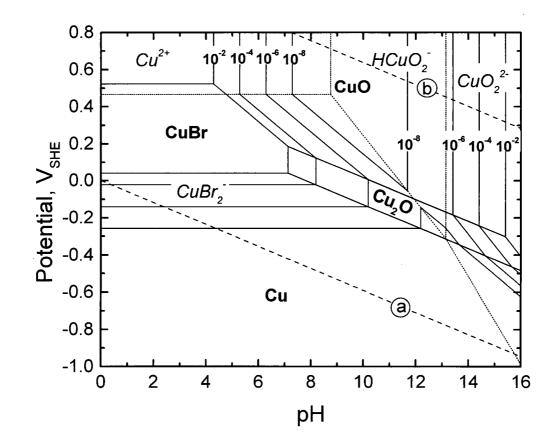
Figure 14 Potential-pH equilibria for the Cu-Br -H<sub>2</sub>O system
