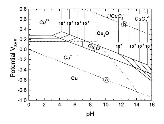
Figure 15 Potential-pH equilibria for the Cu-H<sub>2</sub>O system
