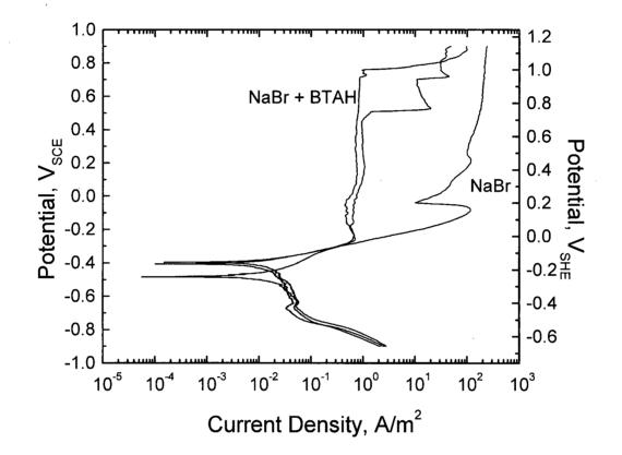
Figure 19 Polarisation behaviour of Cu in 1M NaBr containing 1.0 g/l BTAH at pH 3.0 Behaviour compared with 1M NaBr at pH 3.0
