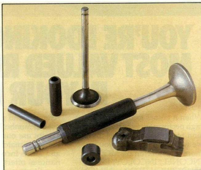
Fig. 2. Sintered \alpha -SiC/TiB 2 particulate ceramic composite valve-train components, including guides, roller follower, and rocker-arm pads, provide the potential for super-hot running engines and extremely low wear (Produced from Sohio Engineered Materials).
