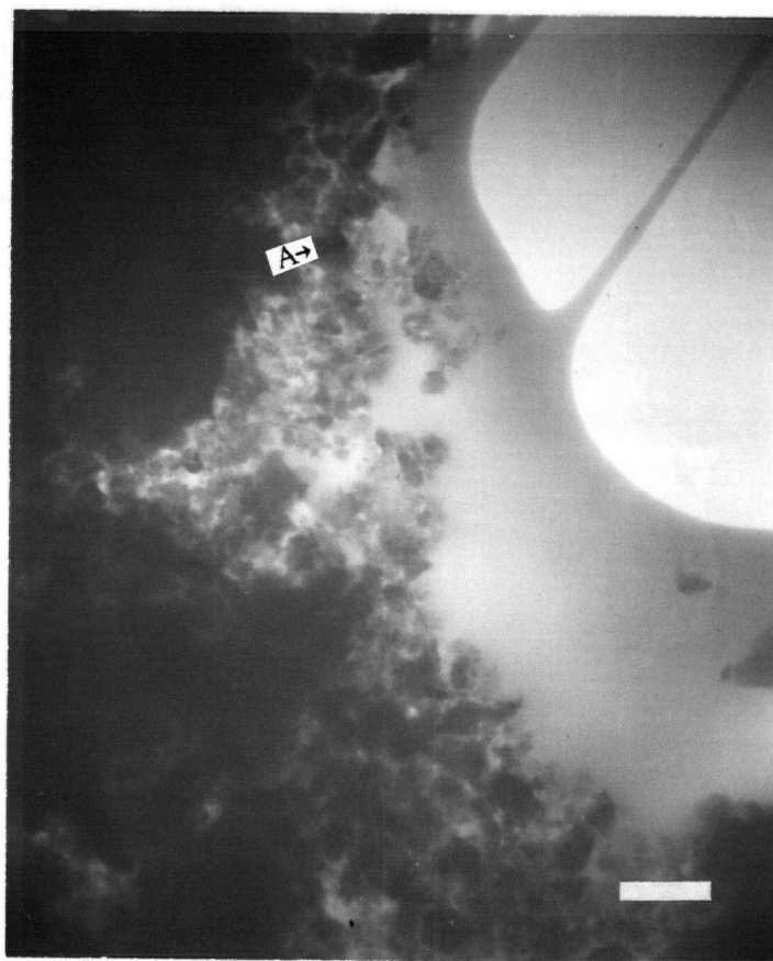
Fig. 21(a). STEM micrograph of mullite + \text{SiO}_2 + C showing the general nature of the phases present (bar = 2\mu\text{m} ).
