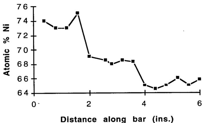
Figure [23] - EDXA results for Ni<sub>3</sub>Al bar
