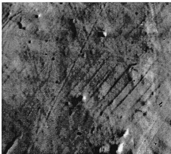
**Figure [45] - Strain induced martensite transformation observed during cavitation testing of 58 at. % Ni (1000X)**
