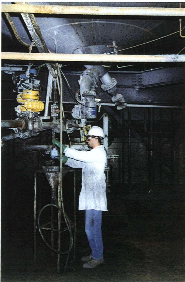
Figure 4-1. Sample taking from the sample point of the IPC thickener underflow line.
