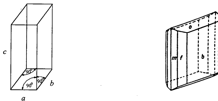
Figure 2.12 Orthorhombic unit cell and equilibrium crystal shape of antlerite (see also Appendix I-F).
