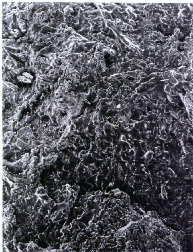
Figure 1.6. Photomicrograph of Type-A crack surface taken near the surface of the refractory with an SEM at a magnification of 30X showing smooth regions indicative of the presence of molten and/or viscous material at time of crack formation.
