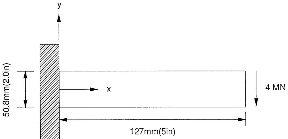
Figure 5.14. Schematic illustration of beam bending problem employed for verification of load-deflection calculation.
