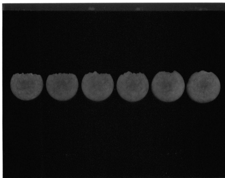
Figure 3.6 Damage profile of type II rod I ( R=0.45 ). Cross sections are at 30 mm intervals from the central load point (left) to the maximum extent of longitudinal damage (right).
