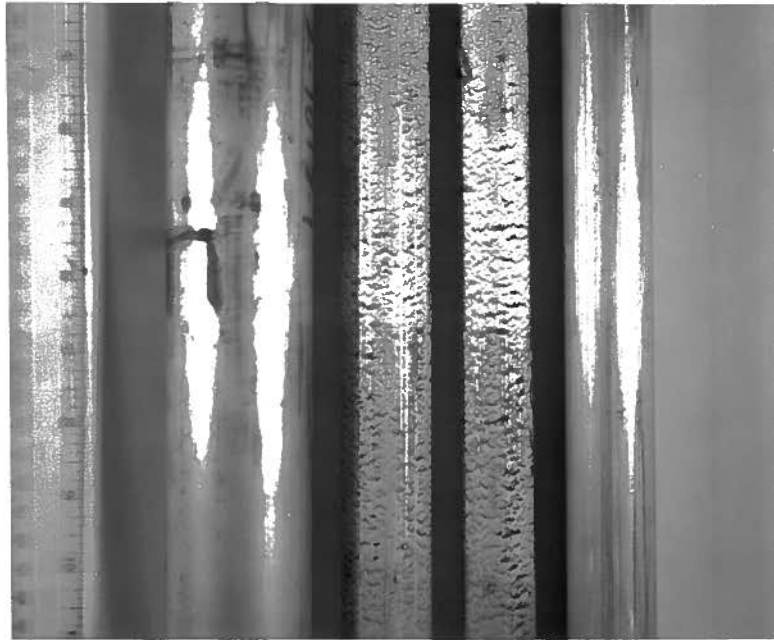
Figure 4.14 Low speed cracking at the front end of two extrudates
