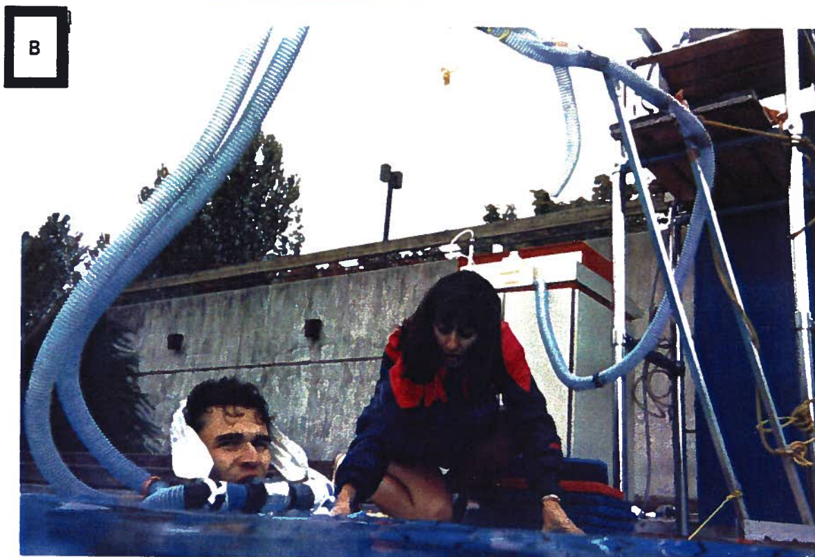
Figure 3. WI running; an above and below surface picture. A. Underwater picture of a subject WI running. The waist harness is shown in this picture. During testing the water ski belt would be worn on top of this harness (see Figure 2). Also shown are the positions of the 2 HR monitors worn for WI running testing. B. Mouthpiece apparatus assembly for WI running testing is shown. The mouthpiece is secured on the subject with head support for VO_{2max} testing.
