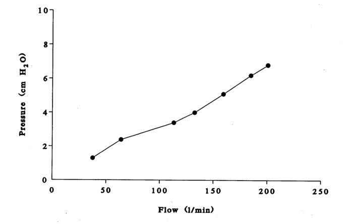
Appendix F: Resistance of the Ventilatory Endurance Apparatus. As air flow increases, resistance increases.
