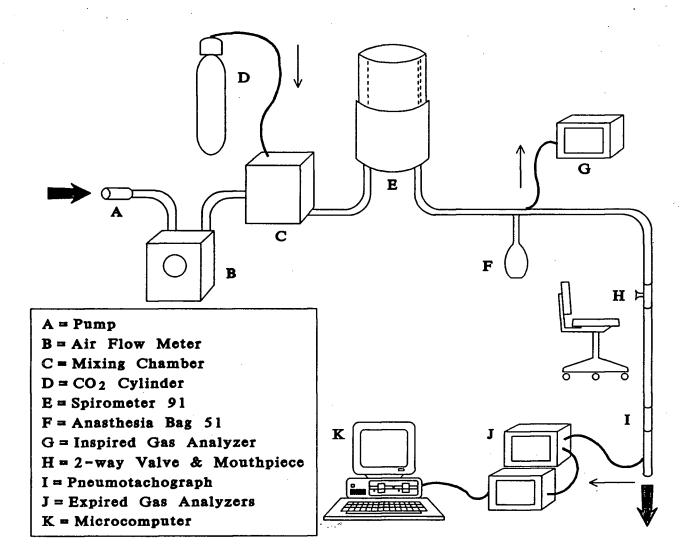
Figure 1: Ventilatory Endurance Apparatus for testing and training respiratory muscles. Arrows indicate direction of air flow.
