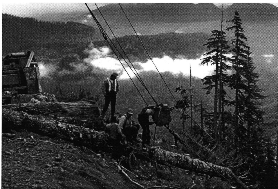
Figure 12. MSP (dropline) carriage used with the swing yarder.
