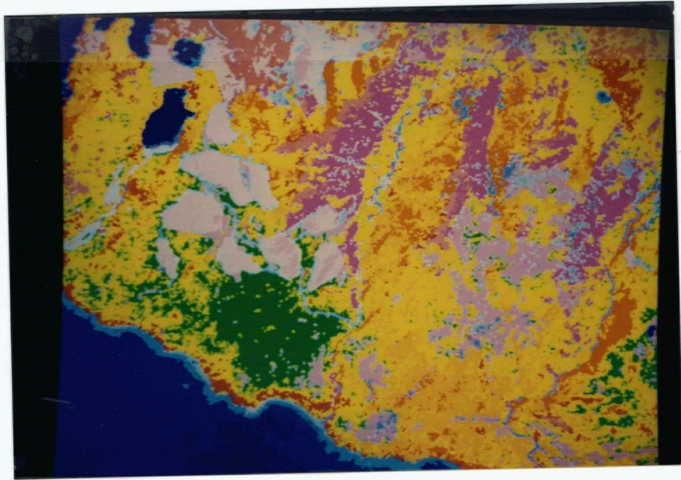
Figure 11. Results of maximum-likelihood classification of Carmanah TM data. Blue is water, light blue is clouds, cyan is shoreline, green is mixed cedar/hemlock stands of normal stocking, purple is upland conifers, red is mixed spruce and hemlock, orange is conifers on north-facing slopes, deep pink is new and old regenerating stands, light pink is alpine conifers, orange-yellow is densely stocked cedar and hemlock stands, yellow is cedar/hemlock/fir, violet is scrub stand, light violet is new clearcuts, pale violet is old clearcuts, light cyan is creeks, black is null class. (a) June, 1992 thematic map (b) September, 1992 thematic map (c) multitemporal (combined) thematic map.
