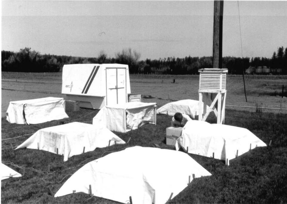
Figure 1. Reflective tarpaulin shelters set up outside the Red Rock Research Station, Prince George, in June 1992. The Fiberglass Insulated Seedling Transporter (FIST) canopy is seen in the far left corner of the picture. The shelter to the left of the canopy is Treatment 10 - a purpose-built shelter manufactured commercially. The ambient temperature was recorded inside the weather station shown on the right.
