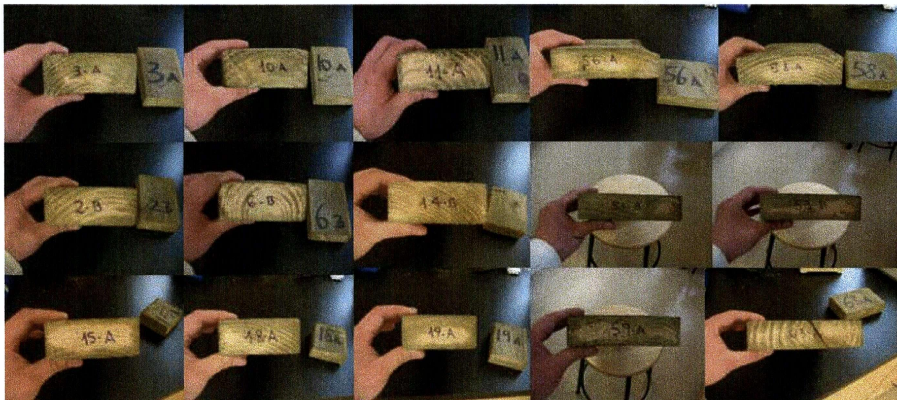
Figure 5-1 Cross section of the CX™ treated boards
