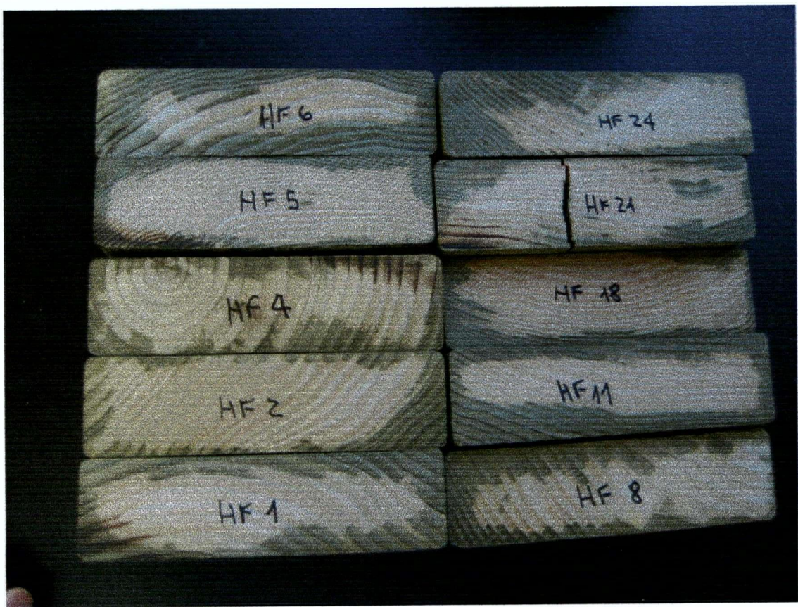
Figure 4-7 Cross section of the references samples of the hem- fir CAz treated boards
