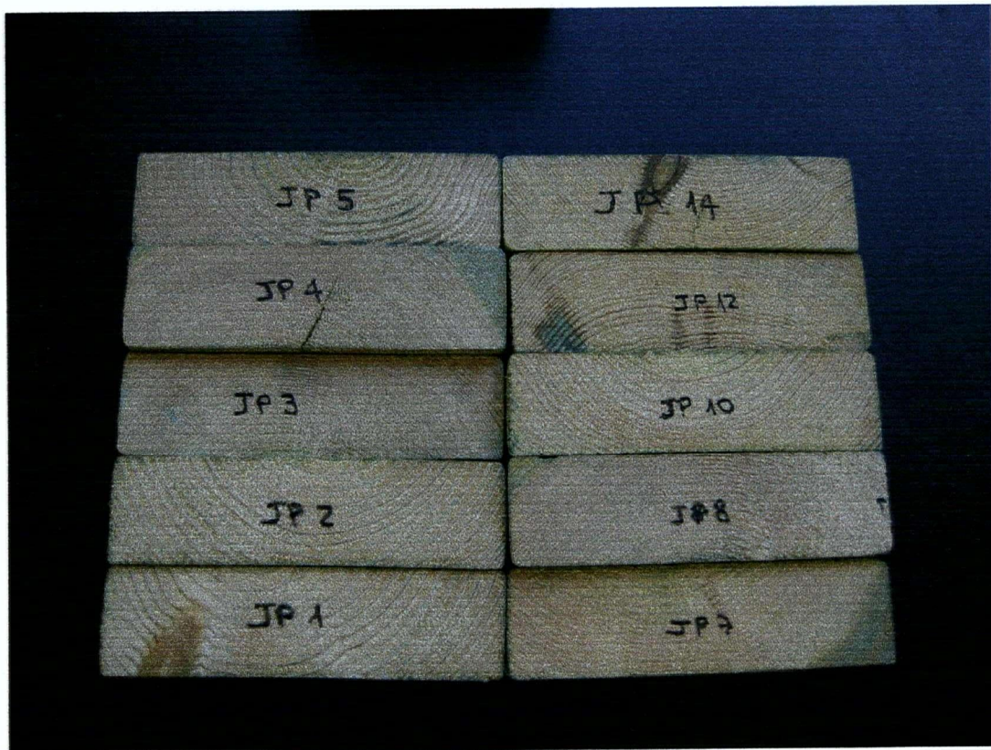
Figure 4-6 Cross section of the references samples of the jack pine CAz treated boards
