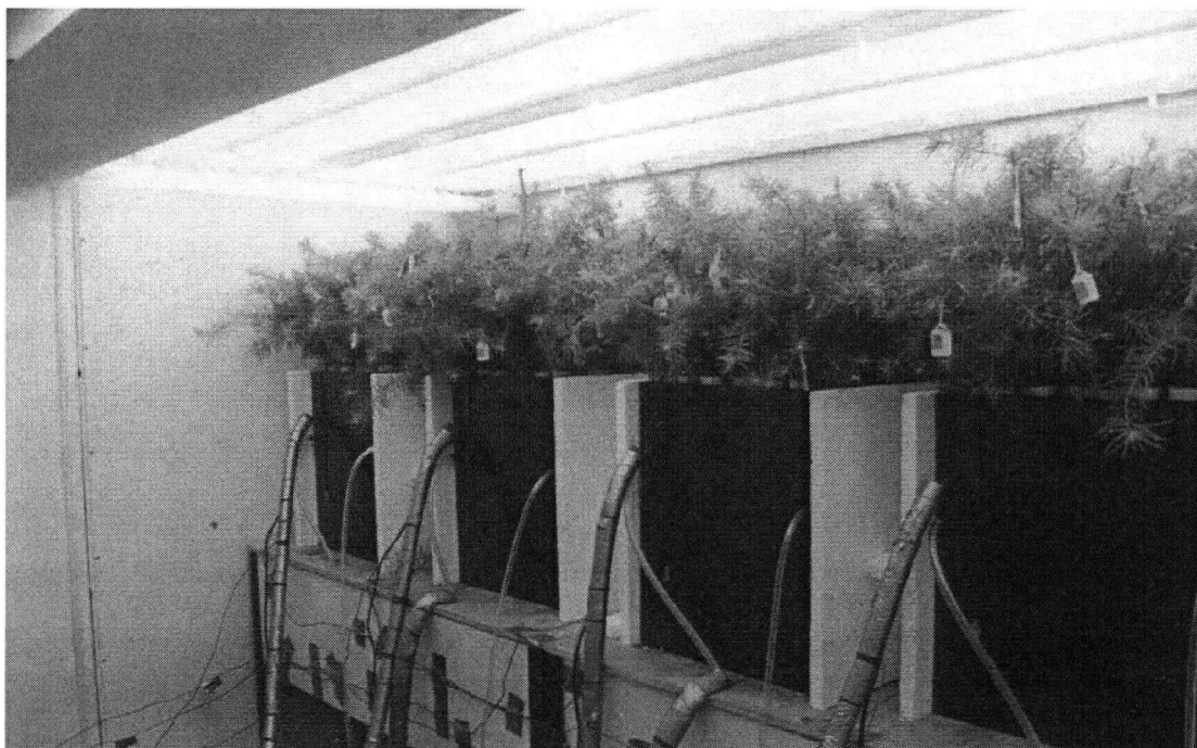
Figure 2.2. Picture of the aerogenic mist chambers (AMCs) and seedlings following transfer. From left to right the chambers are at 16, 24, 16 and 24°C.
