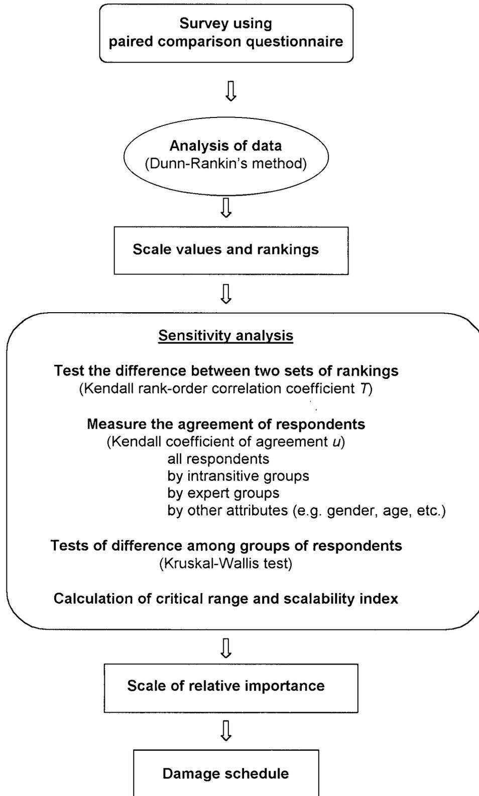
Figure 3.1 General model for constructing the damage schedule.
