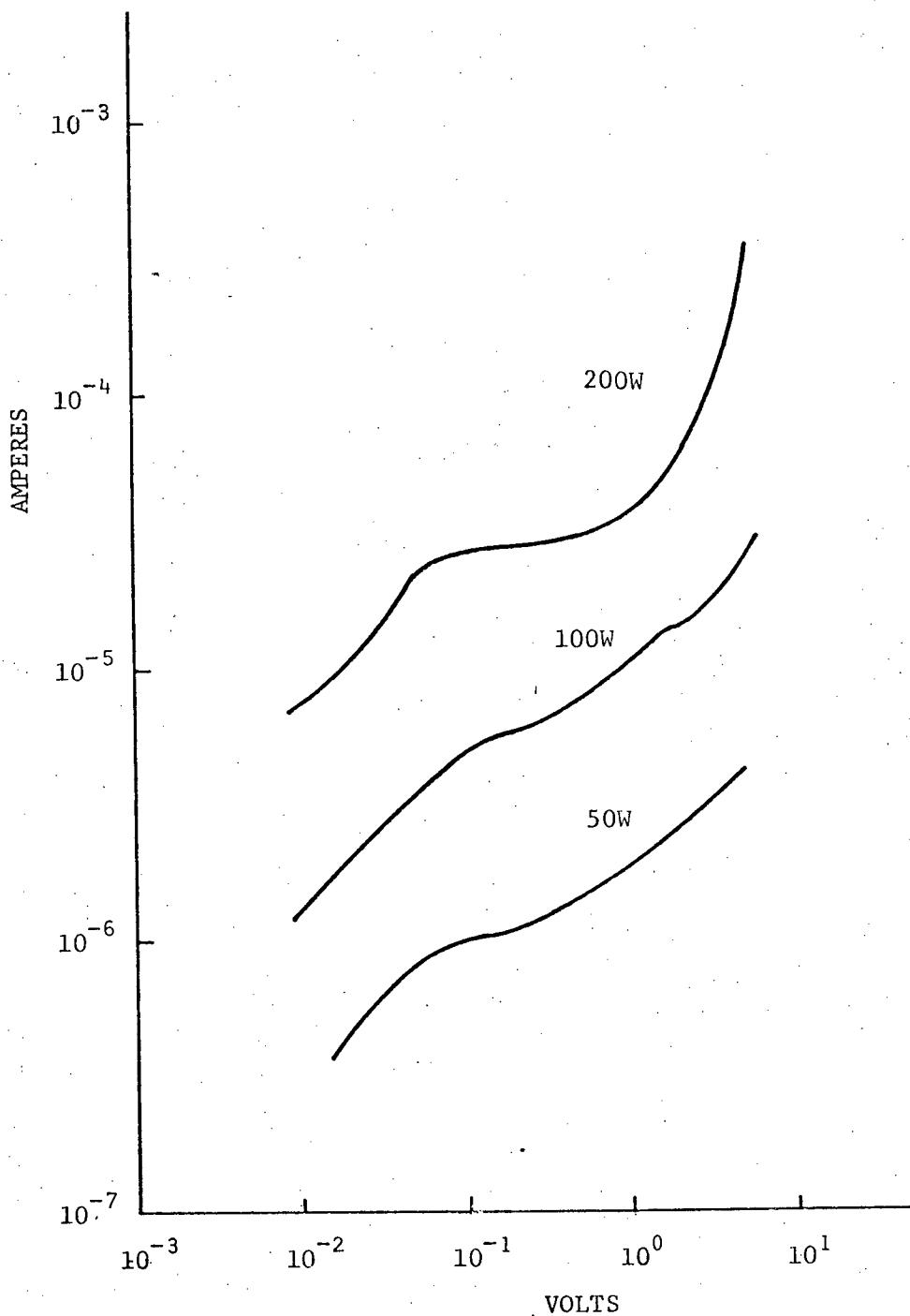
Fig. 6.11 Dark reverse I-V characteristics for  $\text{Cu}_2\text{O}/n\text{-Si}$  diodes fabricated at different sputtering power levels.
