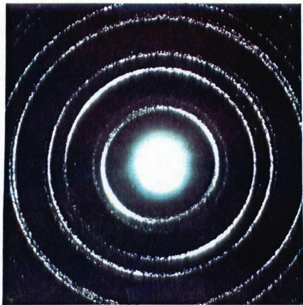
Fig. 4.1e      Electron diffraction pattern taken from gold film.
