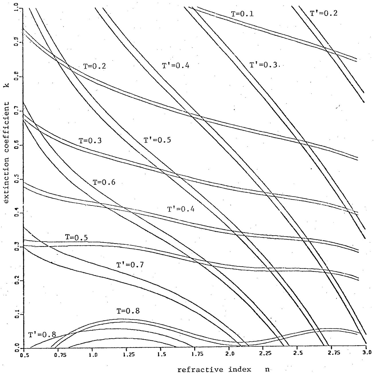
Fig. 5.3 Transmittance curves for a sample with thickness of  $1080\text{\AA}$  ( $T$ ) and for a sample with thickness of  $360\text{\AA}$  ( $T'$ ). The width of the contours represents an experimental error in transmittance measurements of  $\pm 1\%$  of their nominal values. Curves were computed for  $n_s = 1.5$  and  $\lambda = 6000\text{\AA}$ .
