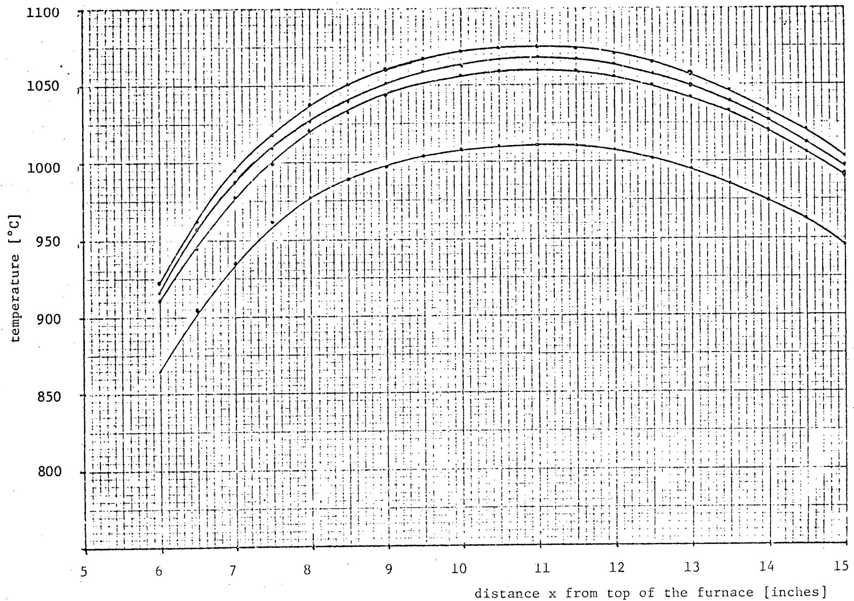
Fig. A.2 Temperature profile of the oxidation furnace at 1.48 l/min. of air flow. The distance is measured from point L, see Fig. A.1.
