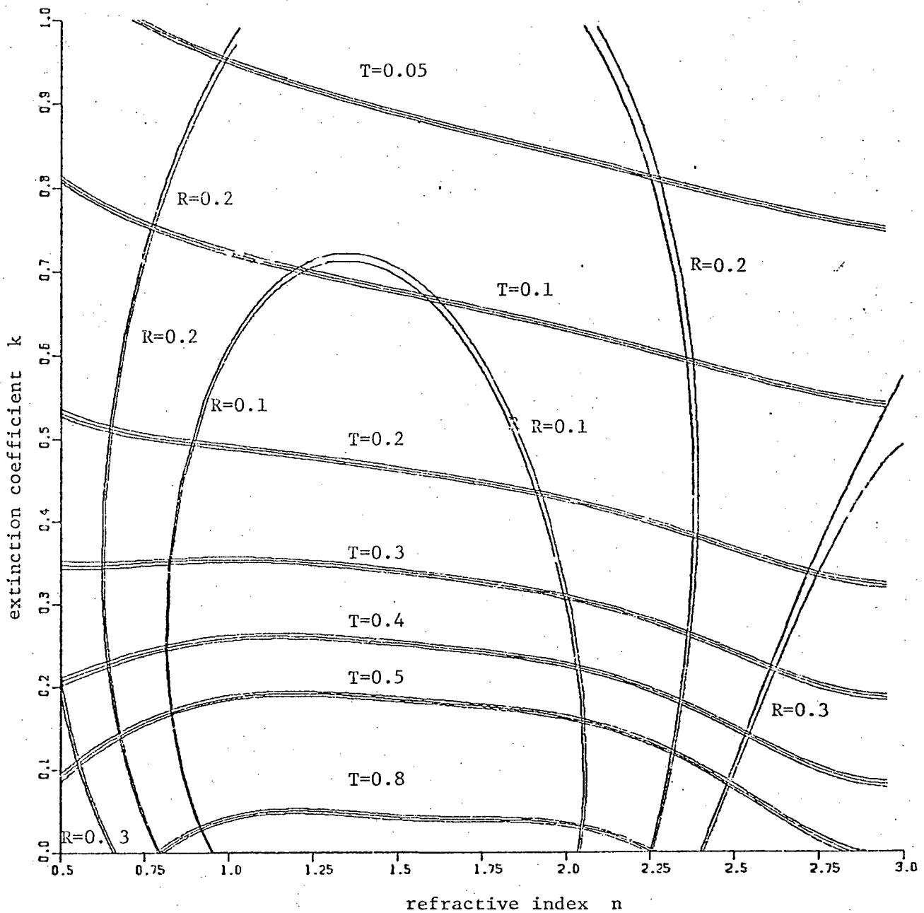
Fig. 5.4 Transmittance and reflectance curves for film with thickness of 1080 Å. The countours width indicates an error in transmittance and reflectance measurements  $\pm 1\%$  of their nominal values. Curves were computed for  $n_s = 1.5$  and  $\lambda = 4000\text{\AA}$ .
