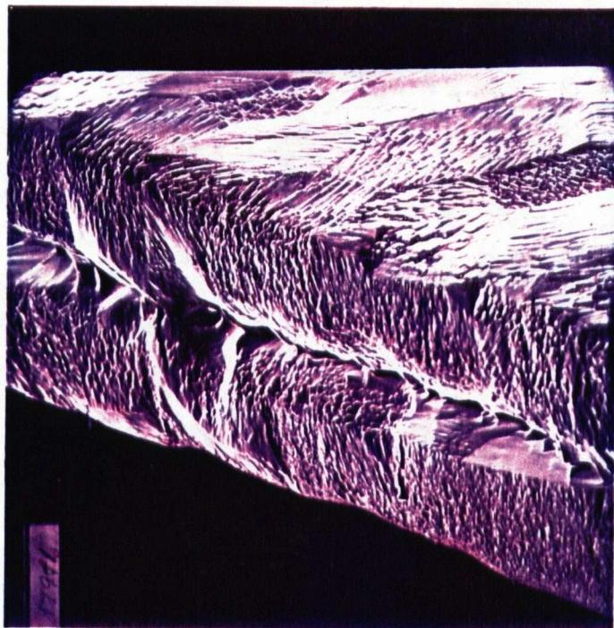
Fig. A.5      Cross section SEM print of completely oxidized Cu foil.
