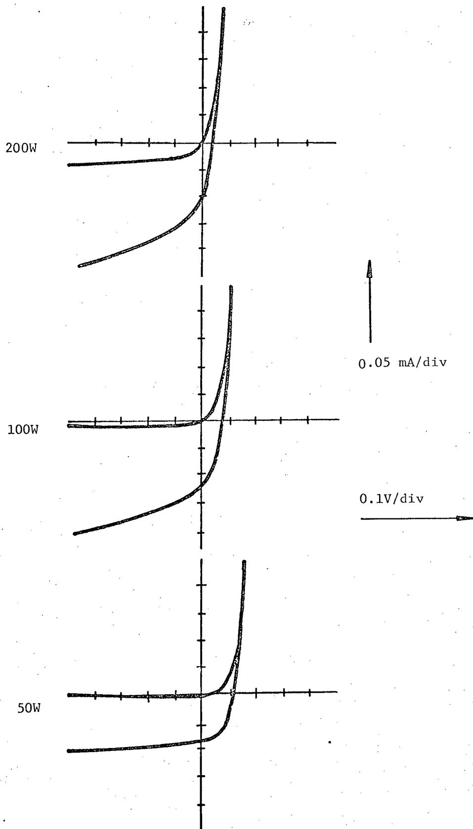
Fig. 6.7 Dark and illuminated ( $100 \text{ mW cm}^{-2}$ ) I-V characteristics for  $\text{Cu}_2\text{O}/\text{n-Si}$  diodes fabricated at different sputtering power levels.
