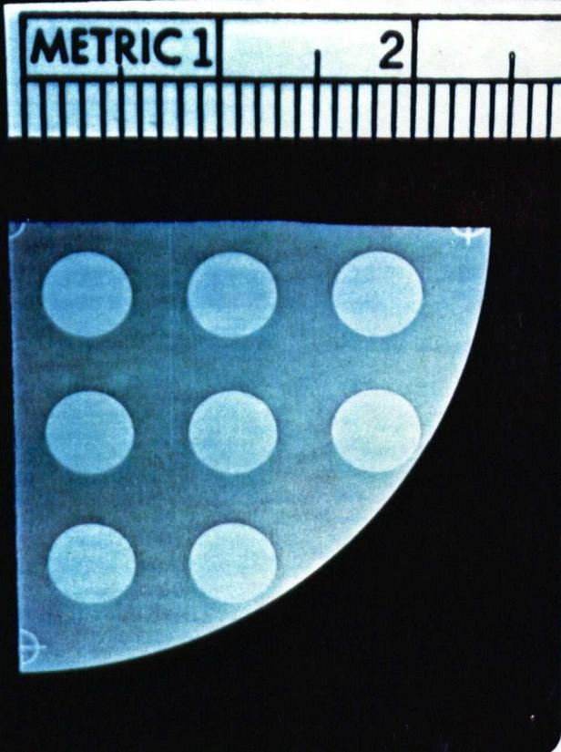
(a) Silicon wafer prepared for  $\text{Cu}_2\text{O}$  deposition.
