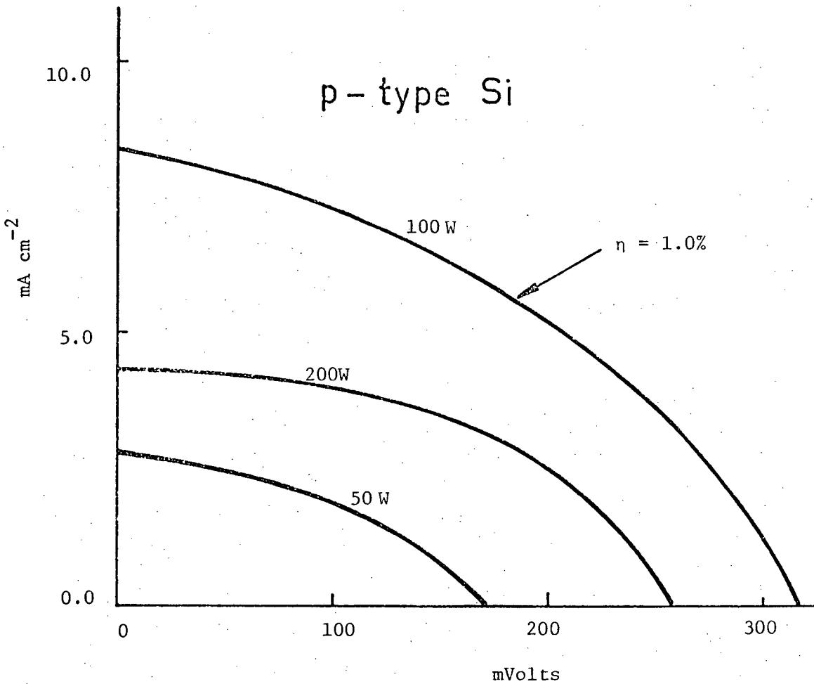
Fig. 6.12 Illuminated ( $100 \text{ mW cm}^{-2}$ ) I-V characteristics for  $\text{Cu}_2\text{O}/\text{p-Si}$  heterojunction diodes fabricated at different r.f. power levels.
