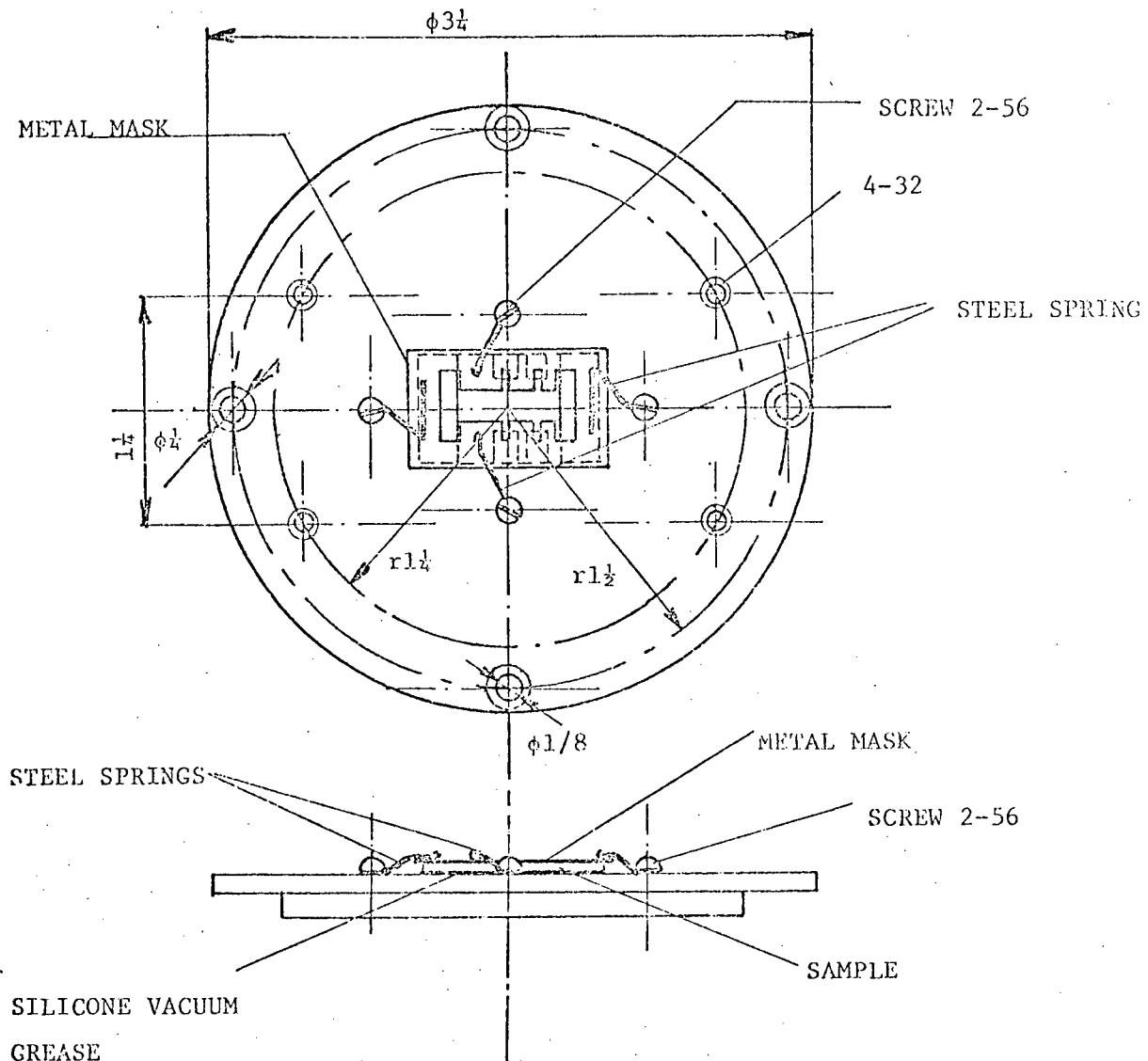
Fig. 3.4b Substrate table sample holder as used for deposition of samples for determination of thermal activation energies for conductivity.
