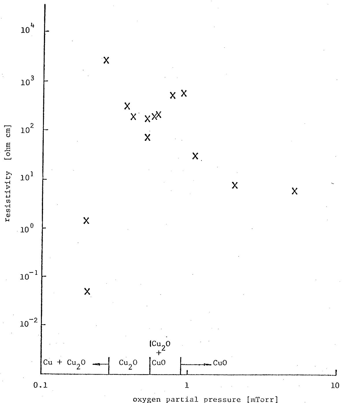
Fig. 4.6 Resistivity data for films deposited by d.c. sputtering at 70 mA and total pressure of 75 mTorr. The partial pressure boundaries for the various film compositions are from Table 4.2.
