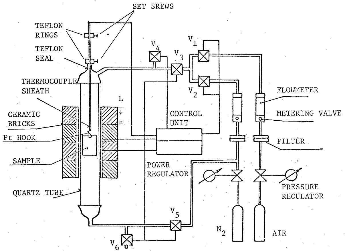
Fig. A.1 Vertical furnace for thermal oxidation and single crystal growth of  $\text{Cu}_2\text{O}$ .
