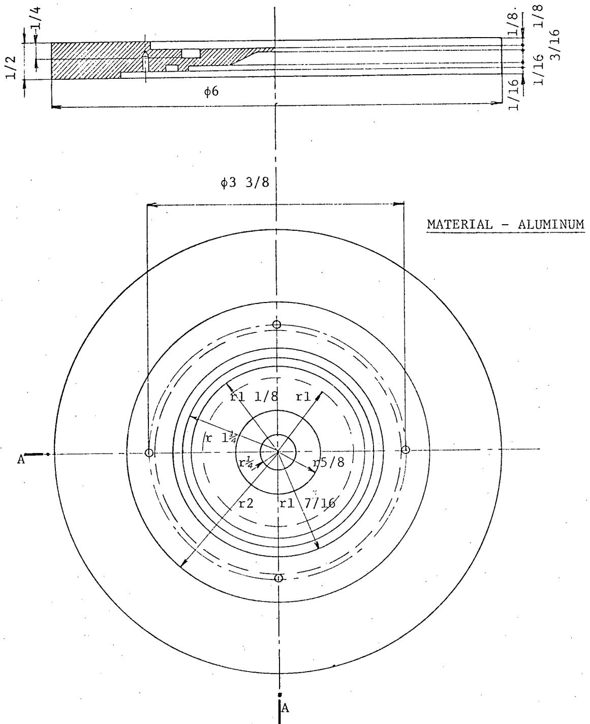
Fig. 3.4a Custom-made substrate table enabling efficient cooling of samples during their deposition. All dimensions are in inches.
