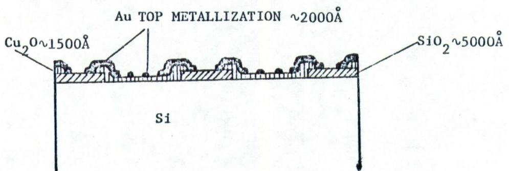
(c) Schematic view of  $\text{Cu}_2\text{O}/\text{Si}$  solar cell cross section.
