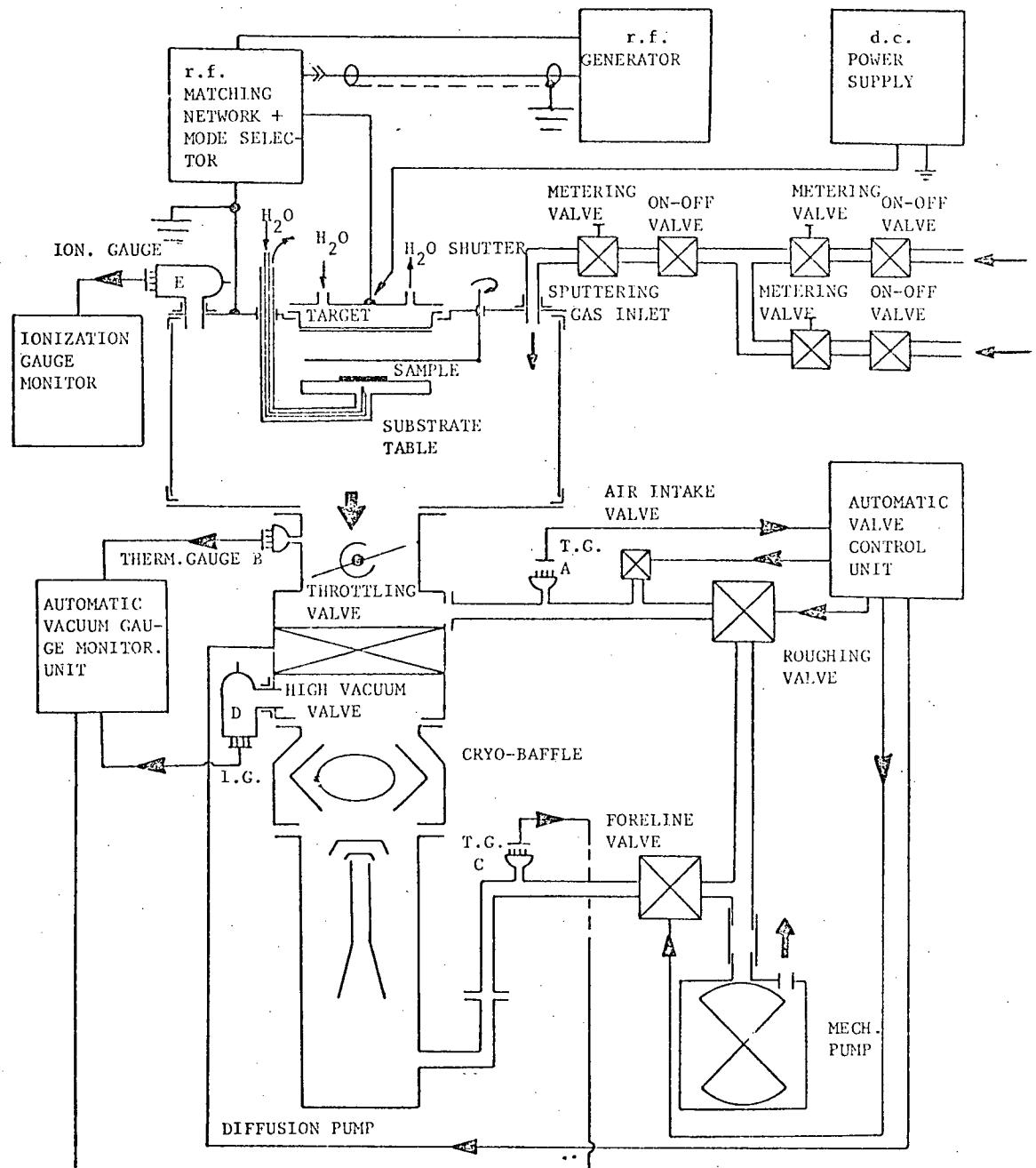
Fig. 3.1 Schematic diagram of reactive sputtering system used for copper oxide film deposition
