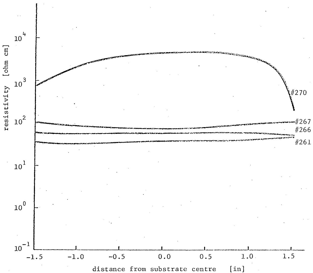
Fig. 4.13 Variation of resistivity with radial distance along copper oxide films. The sample numbers refer to those marked on Fig. 4.5.
