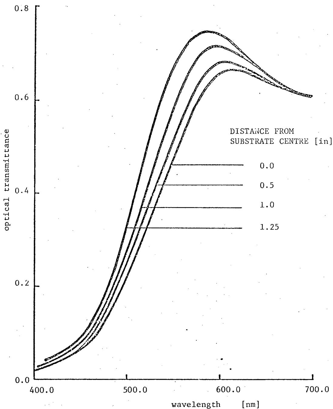
Fig. 4.3 Variation of optical transmittance with radial distance along copper oxide film (sample #234, see Fig. 4.5). Film thickness = 950 Å. Compare data with that of Fig. 4.2 and note the reduction in Cu content on moving away from the centre of the substrate.
