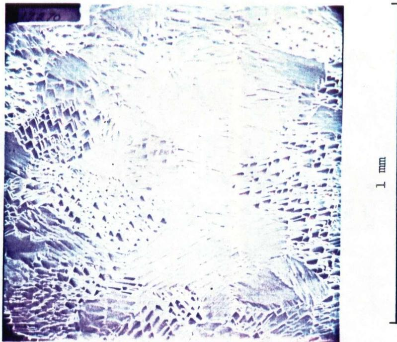
Fig. A.3 SEM print of  $\text{Cu}_2\text{O}$  shortly after the completion of oxidation process.
