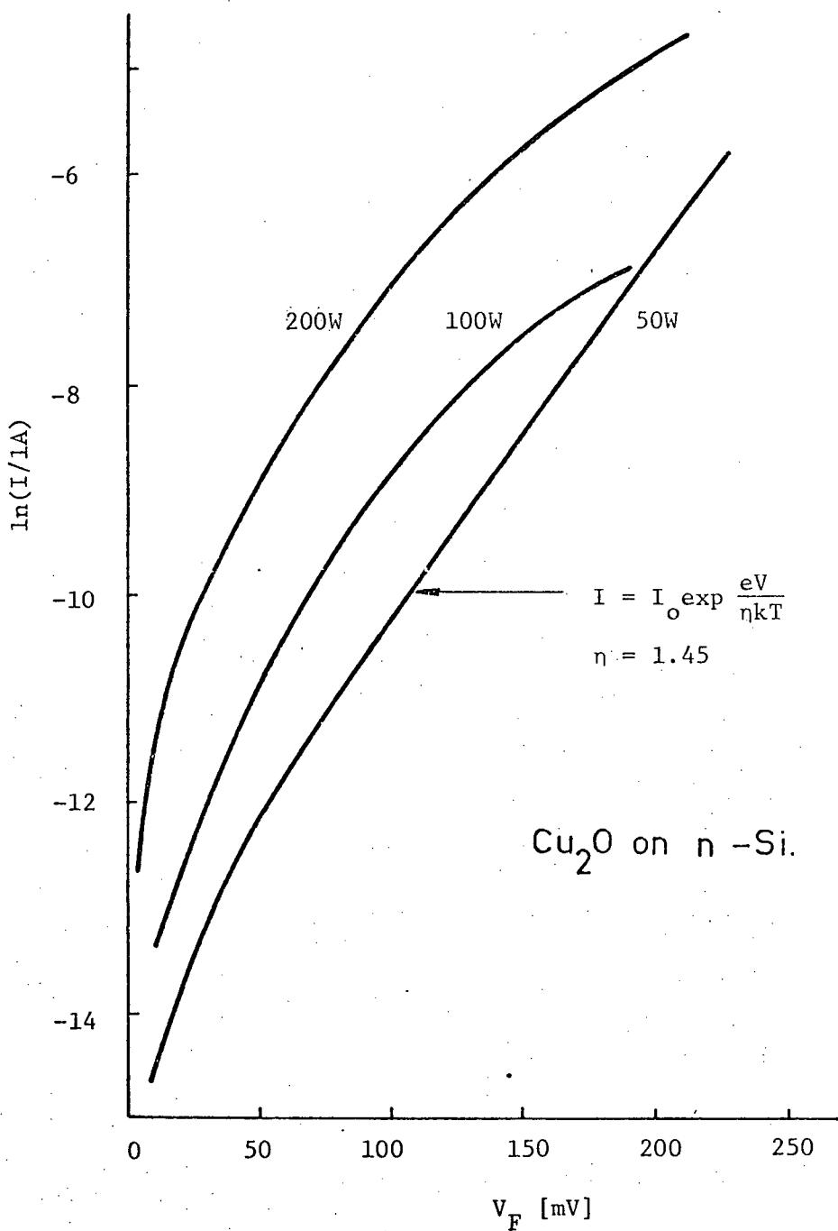
Fig. 6.9 Semilog plot of the forward I-V characteristics from the diodes used to obtain Fig. 6.8.
