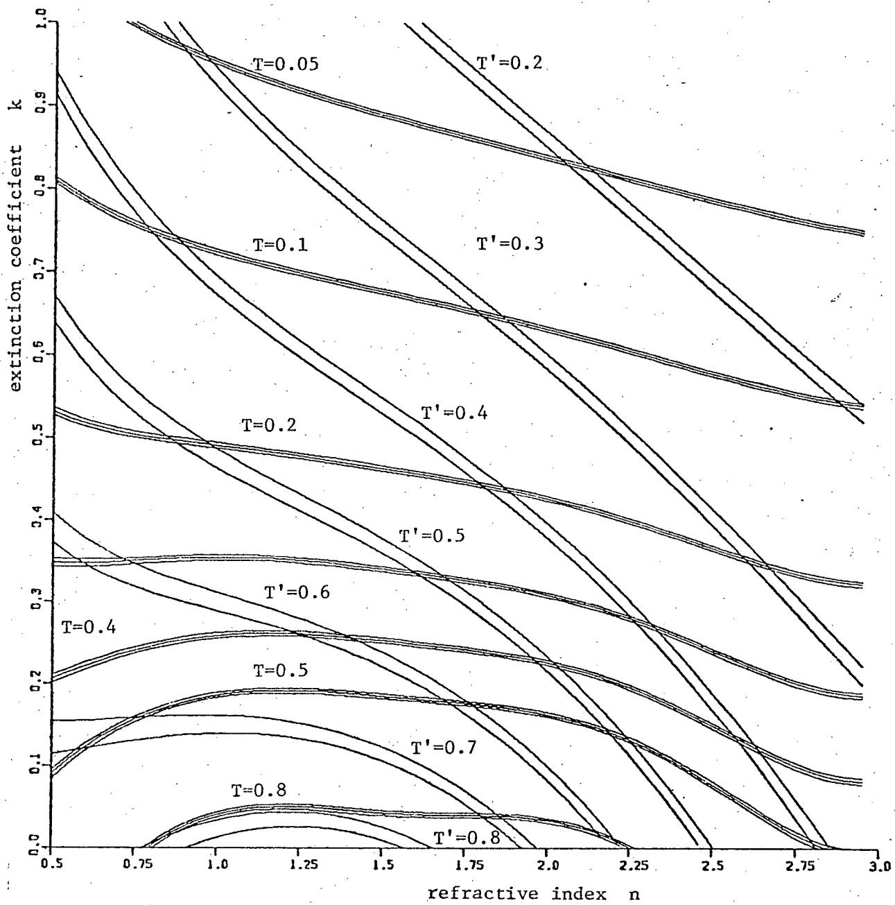
Fig. 5.2 Transmittance curves for two samples of the same material with thicknesses of  $1080\text{\AA}$  (triple line ( $T$ )) and  $360\text{\AA}$  (double line ( $T'$ ))). The width of the contours represents an experimental error in transmittance measurements of  $\pm 1\%$  of their nominal values. Curves were computed for  $n_s = 1.5$  and  $\lambda = 4000\text{\AA}$ .
