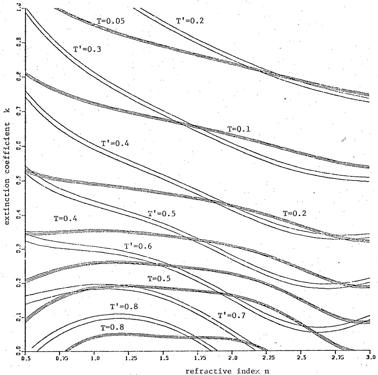
Fig. 5.1 Transmittance curves for two samples of different thickness as a function of refractive indices of the film. The width of the contours indicates an experimental error in transmittance measurement of  $\pm 1\%$  of the nominal transmittance value. The double line represents a sample with film thickness =  $540\text{\AA}$  ( $T'$ ) and the triple line a sample with thickness =  $1080\text{\AA}$  ( $T$ ). Curves are computed for  $n_s = 1.5$  and  $\lambda = 4000\text{\AA}$ .
