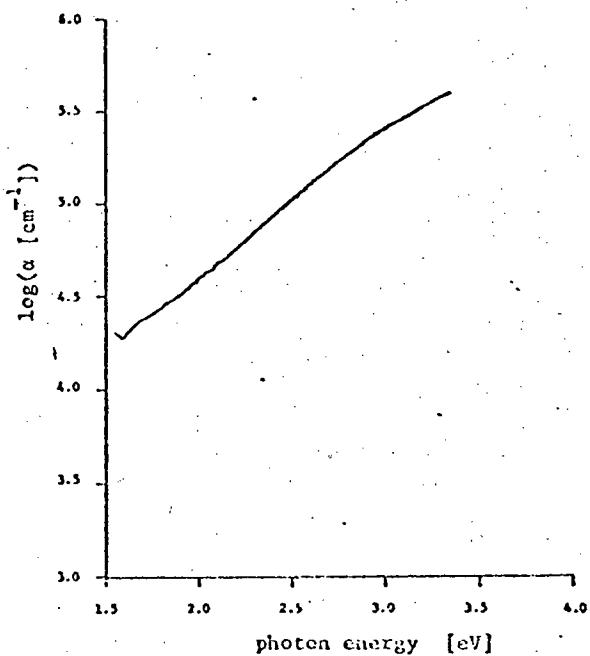
Fig. 5.10 Optical properties of  $\text{Cu}_2\text{O}+\text{CuO}$  1050 Å thick film deposited on the Suprasil 2 substrate at 200W of r.f. power and .7 mTorr of oxygen.
