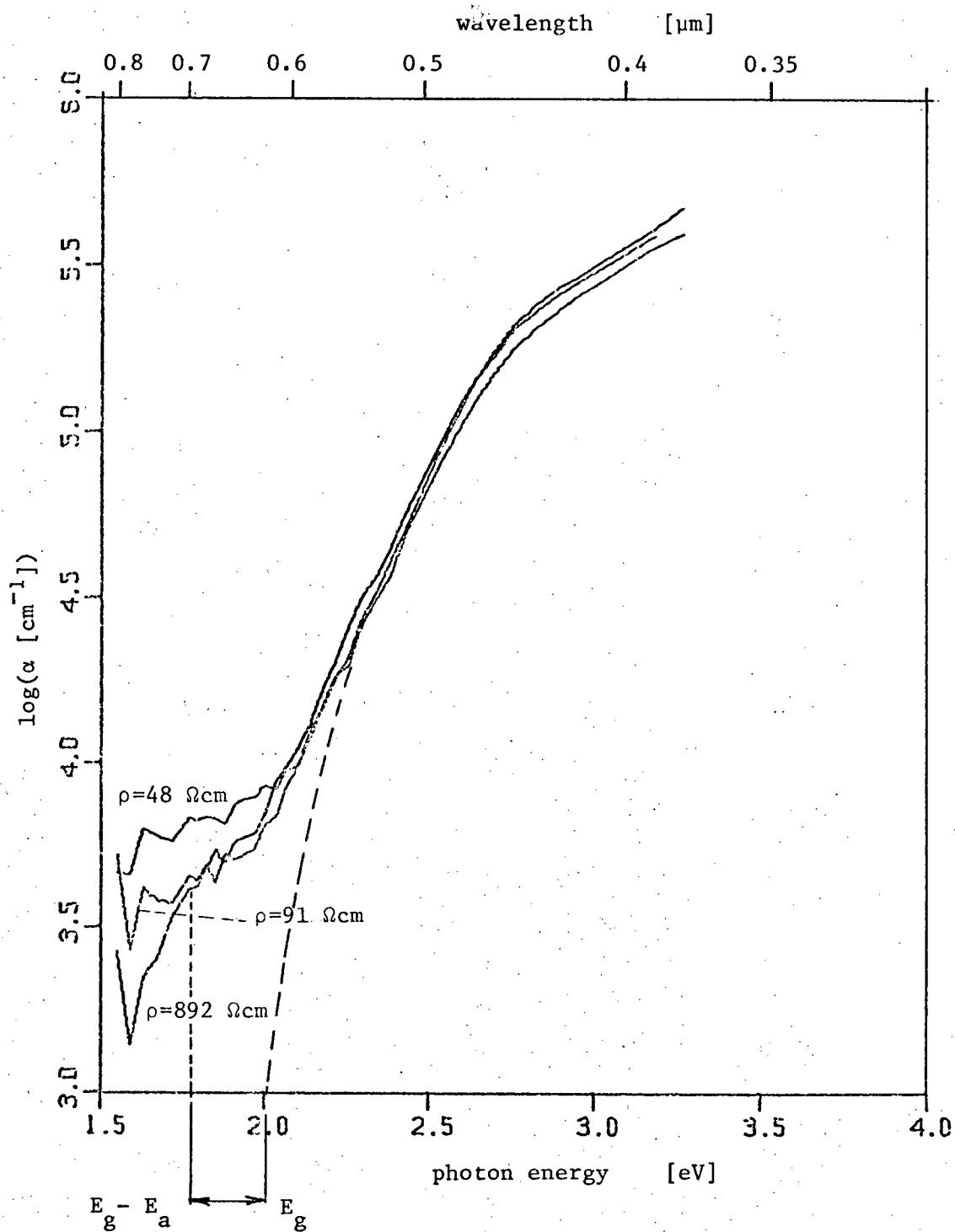
Fig. 5.13 Dependence of the absorption coefficient  $\alpha$  on the photon energy of incident light for cuprous oxide films of different resistivities.
