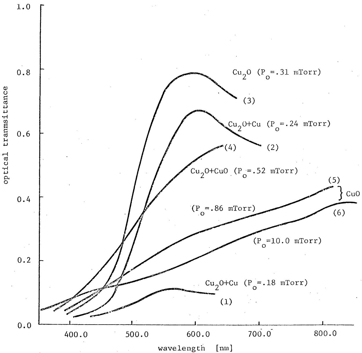
Fig. 4.2 Optical transmittance data for copper oxide films deposited by r.f. sputtering at 200W of forward power and total pressure of 25 mTorr. All data normalized to represent results for 1000 Å thick films.
