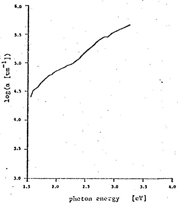
Fig. 5.6 Optical properties of  $\text{Cu}_2\text{O} + \text{Cu}$  1030 Å thick film deposited on Suprasil 2 substrate at 200W of r.f. power and .32 mTorr of oxygen.
