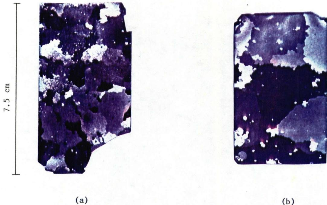
Fig. A.7      Photographs of the Cu<sub>2</sub>O samples prepared from 99.99% Cu with 63 ppm of Ni content. The thickness of the initial copper in both cases was 5 mil. (a) - sample annealed for 1½ hours; (b) - sample annealed for 5 hours.
