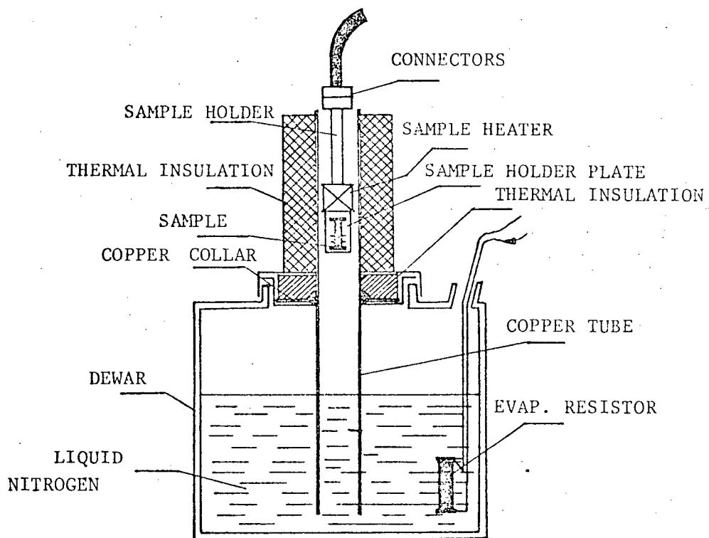
Fig. 4.8 Cryostat used for measurement of thermal activation energies for conductivity.
