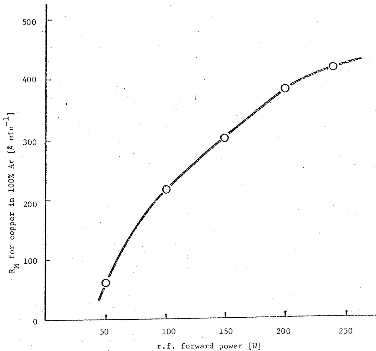
Fig. 4.11 Deposition rate of pure copper (measured at the center of substrate table) for various r.f. power levels and the total pressure of 25 mTorr.
