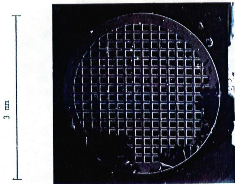
Fig. 3.2 3mm diameter 150 mesh EM copper grid.
