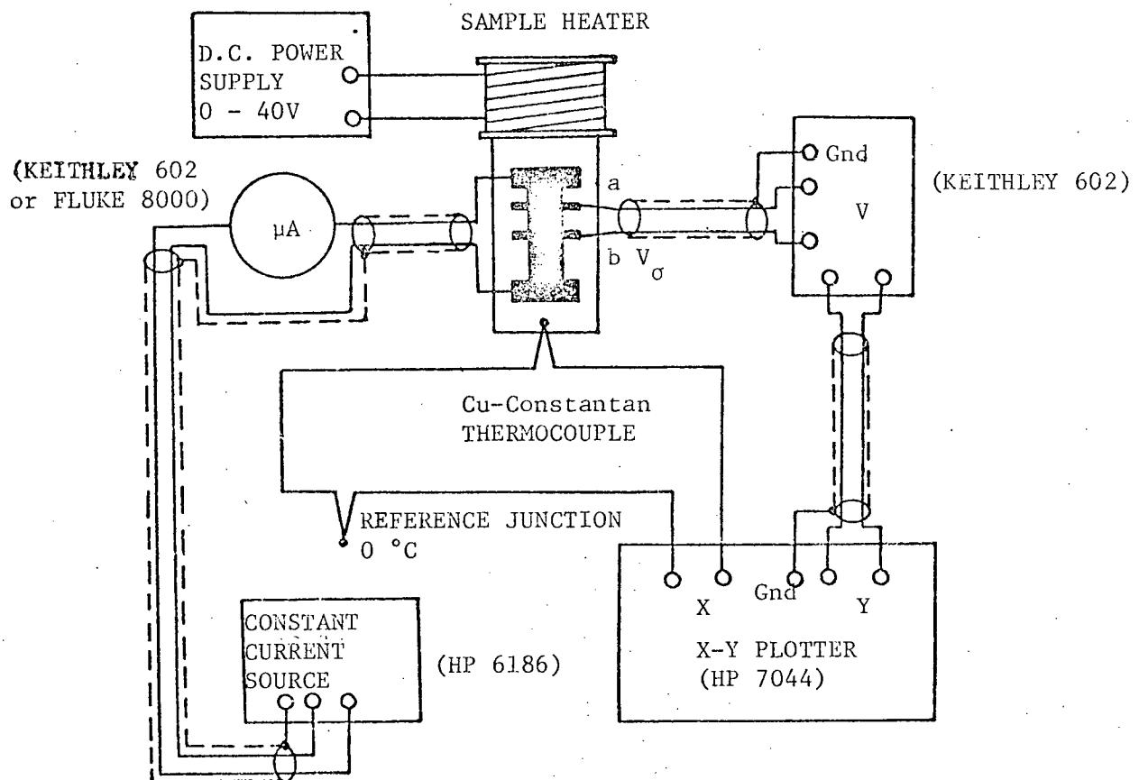
Fig. 4.10 Schematic diagram of the setup for measurement of thermal activation energy for conductivity.
