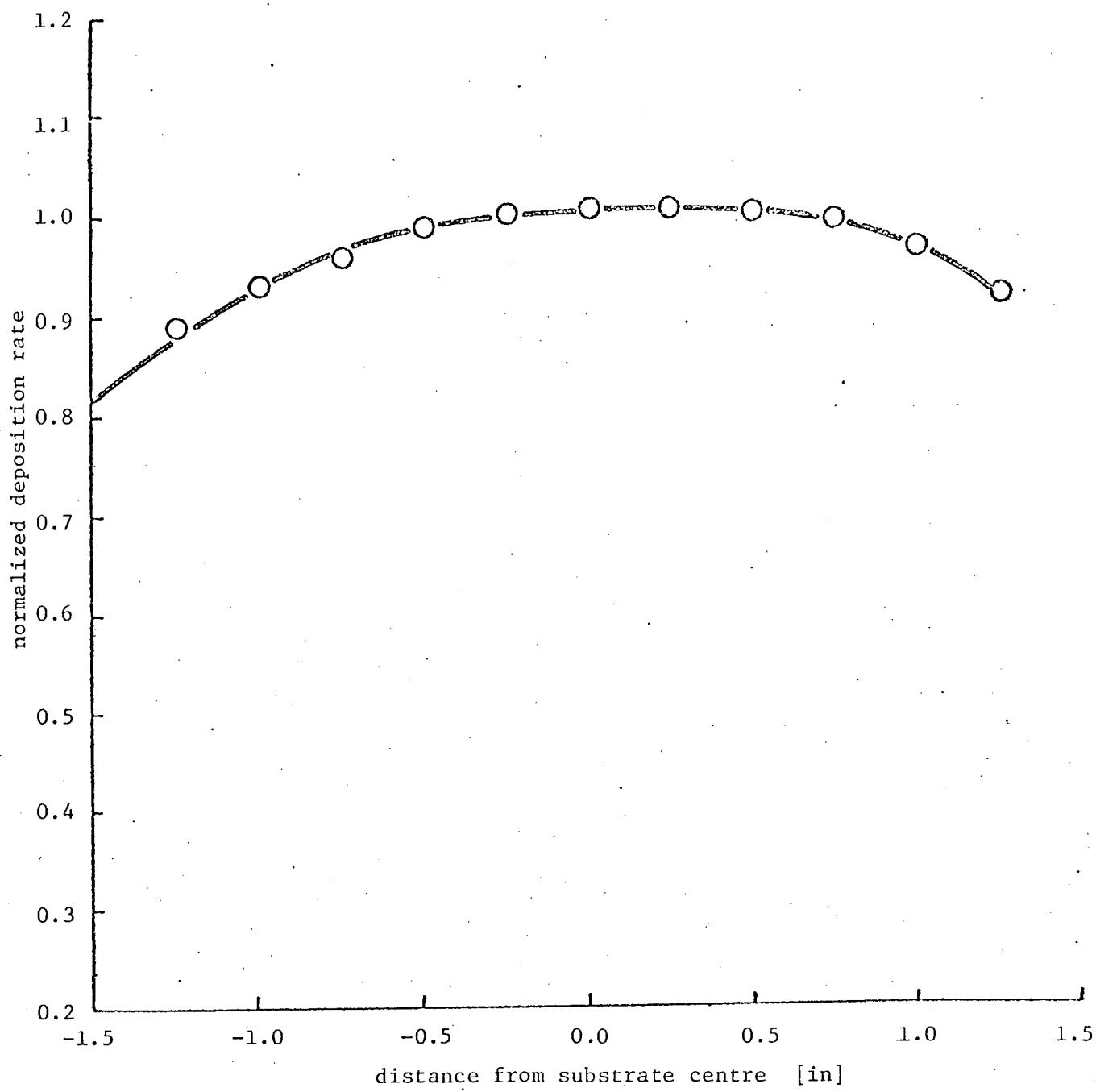
Fig. 4.14 Deposition rate of pure copper r.f. sputtered in 100% Ar, normalized with respect to the deposition rate at the centre of the substrate table. (Total pressure = 25 mTorr).
