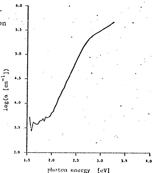
Fig.5.7 Optical properties of the  $\text{Cu}_2\text{O}$  1010 Å thick film deposited on Suprasil 2 substrate at 200W of r.f. power and .36 mTorr of oxygen. The film resistivity  $\rho = 91 \text{ ohm cm}$ .
