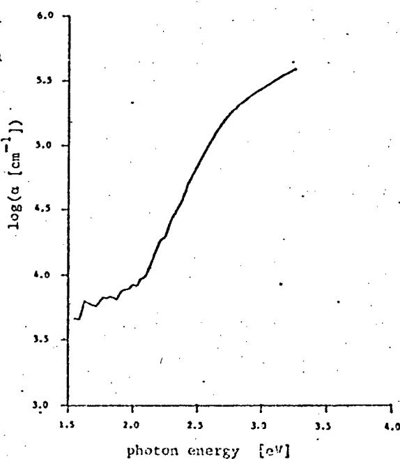
Fig.5.8 Optical properties of the  $\text{Cu}_2\text{O}$  1050 Å thick film deposited on the Suprasil 2 substrate at 200W of r.f. power and .4 mTorr of oxygen. The film resistivity  $\rho = 48 \text{ ohm cm}$ .
