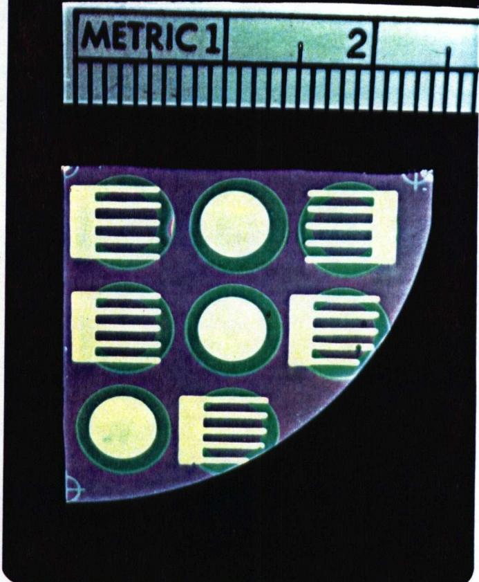
(b) Final  $\text{Cu}_2\text{O}/\text{Si}$  solar cell configuration.
