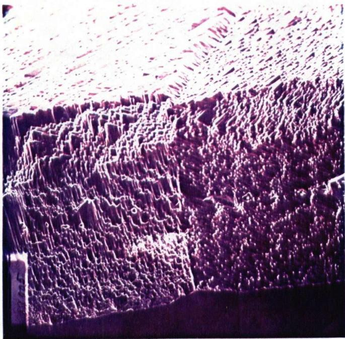
Fig. A.9      Cross section SEM print of completely annealed Cu<sub>2</sub>O sample.
