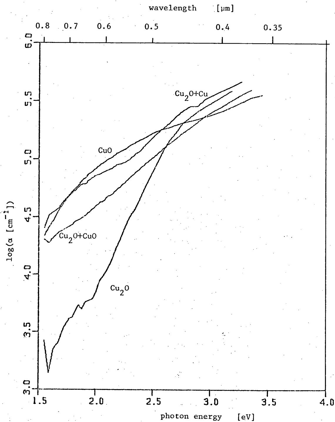
Fig. 5.12 Dependence of the absorption coefficient  $\alpha$  on the incident photon energy for various copper oxide films.
