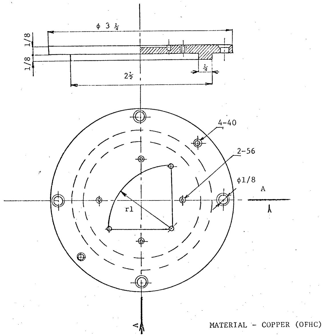
Fig. 6.1 Substrate table sample holder
