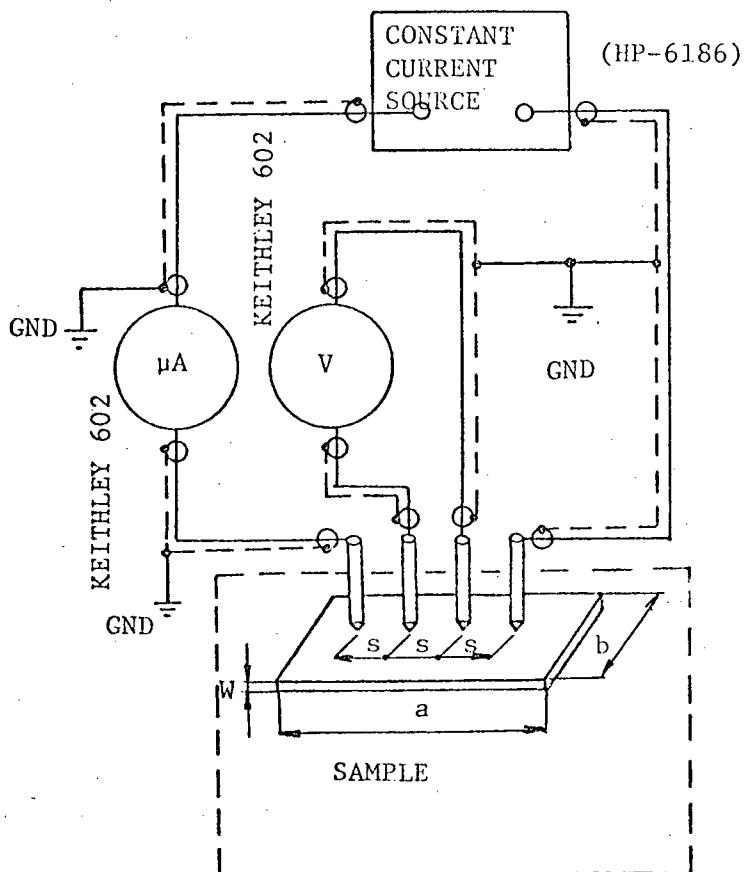
Fig. 4.4 Circuit diagram of the four-point probe set-up used for resistivity measurements.
