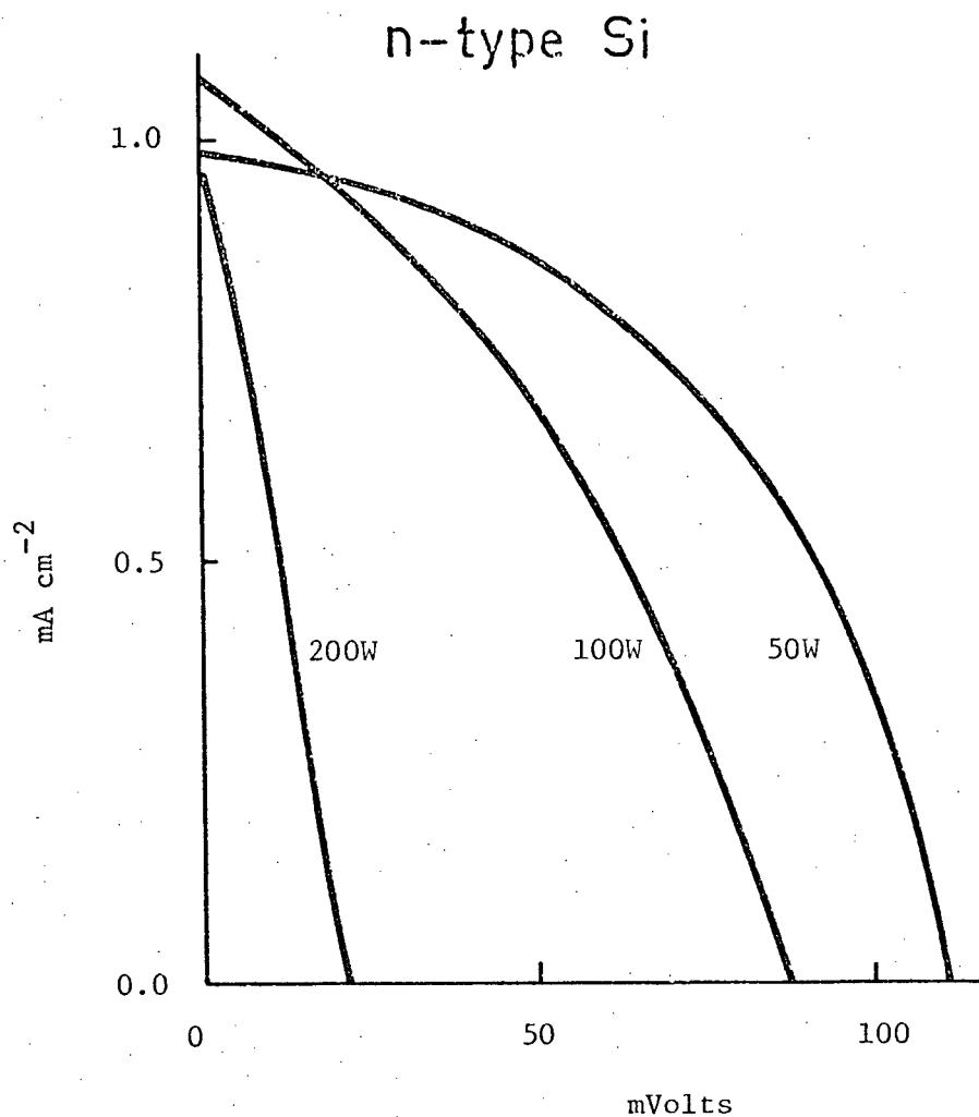
Fig. 6.8 Illuminated ( $100 \text{ mW cm}^{-2}$ ) I-V characteristics for  $\text{Cu}_2\text{O}/\text{n-Si}$  heterojunction diodes fabricated at different sputtering power levels.
