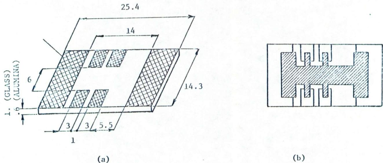
Fig. 3.3a Substrate with contact areas used for preparation of samples for determination of the thermal activation energies of conductivity. All dimensions are in millimeters.
