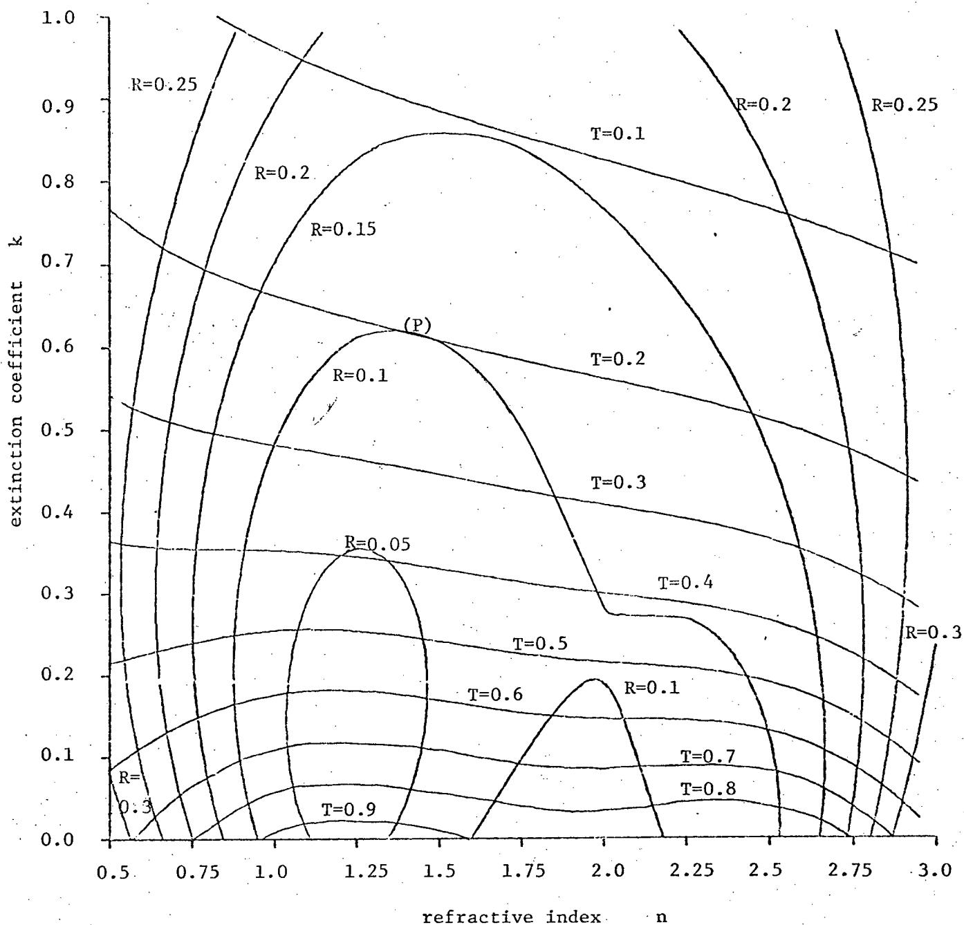
Fig. 5.5 Transmittance and reflectance curves for film with thickness of  $1000\text{\AA}$  at  $\lambda = 5000\text{\AA}$  and  $n_s = 1.5$ . Note, that in this particular case four different solutions for  $n, k$  can be obtained for example, for combination of  $R = 0.1$  and  $T = 0.6 - 0.8$ .
