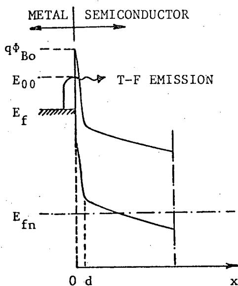
Fig. 6.10 Schematic energy diagram of a reverse biased sputter-damaged Schottky barrier. The damaged region is  $0 \leq x \leq d$ . The thermionic field emitted electrons are indicated by the arrow.  $E_f$  is the Fermi level in the metal and  $E_{fn}$  is the quasi-Fermi level for electrons in the semiconductor.
