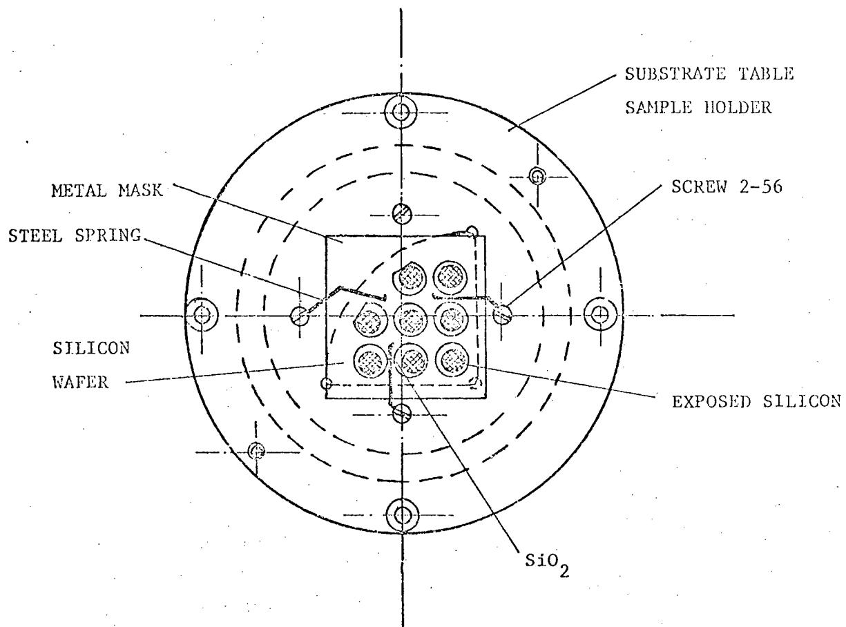
Fig. 6.2 Mask mounting for  $\text{Cu}_2\text{O}/\text{Si}$  heterojunction formation
