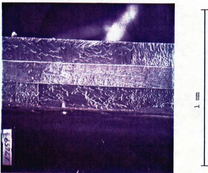
Fig. A.4 Cross section SEM print of partially oxidized Cu plate. Magnification x 125.
