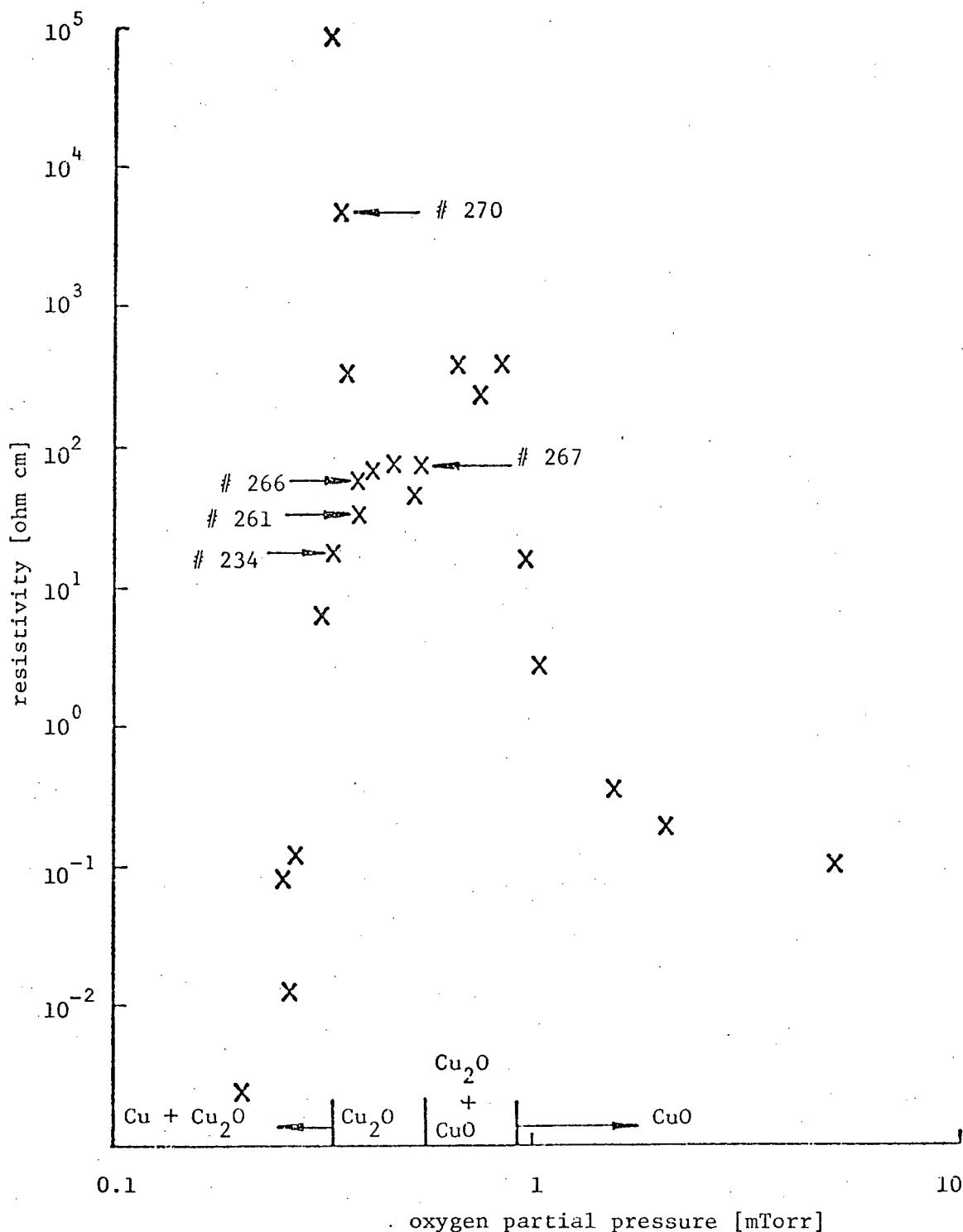
Fig. 4.5 Resistivity data for films deposited by r.f. sputtering at 200W and total pressure of 25 mTorr. The partial pressure boundaries for the various film compositions are from Table 4.2. The sample numbers shown identify the samples used to produce Figs. 4.3 and 4.13.
