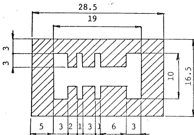
Fig. 4.7 Metal mask for deposition of samples used for measurement of thermal activation energies for conductivity. All dimensions are in millimetres.
