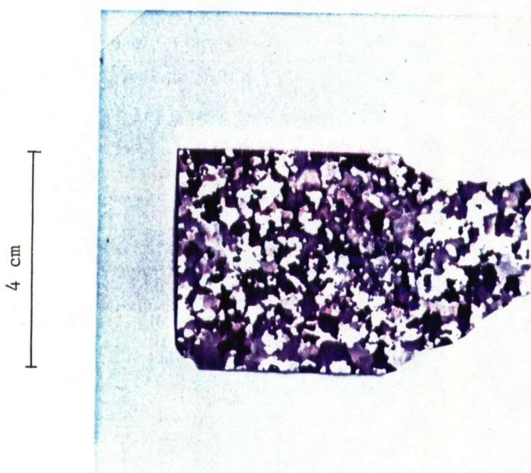
Fig. A.8      Photograph of the Cu<sub>2</sub>O sample prepared from 99.9% Cu 5 mil thick, annealed for 7 hours.
