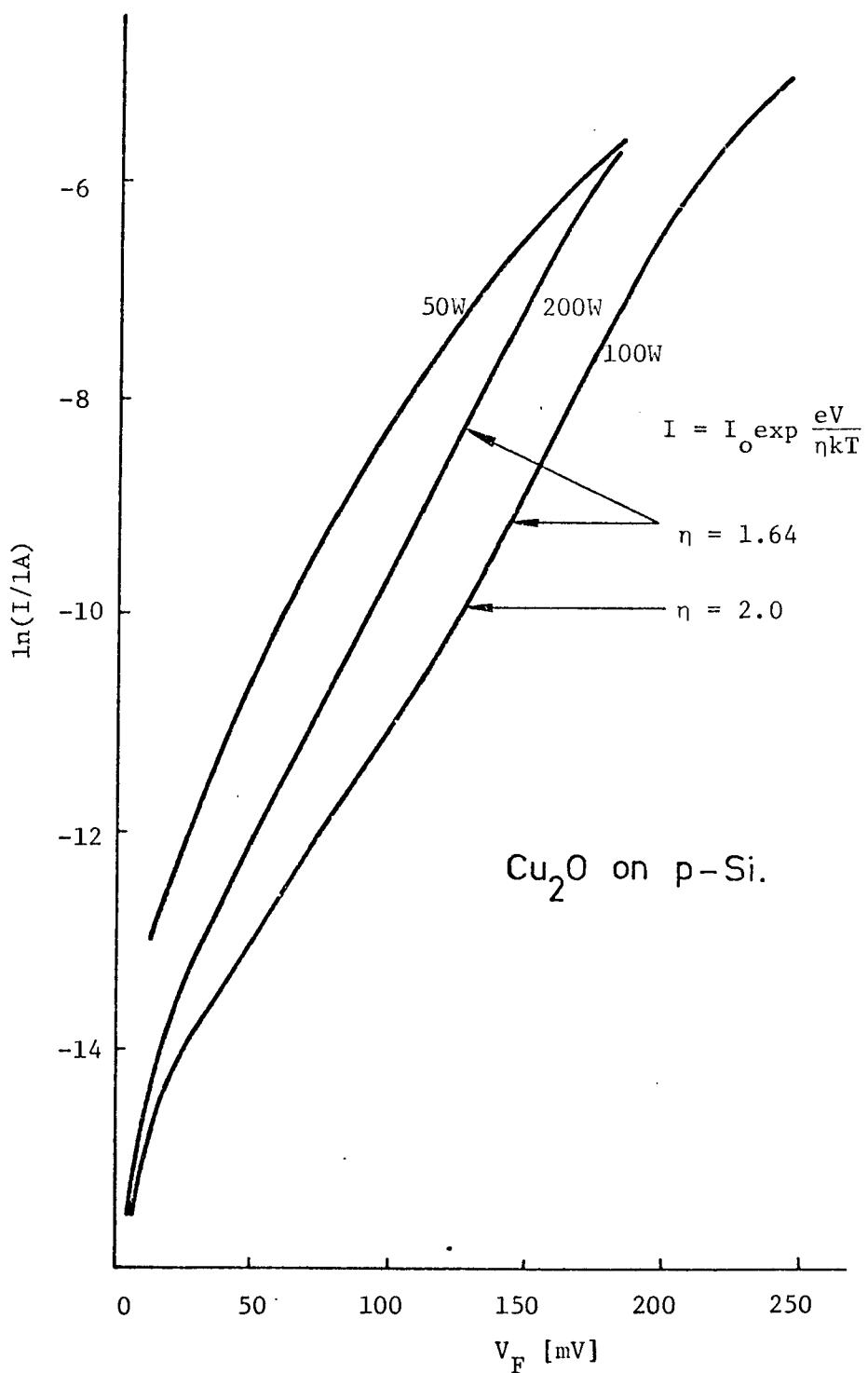
Fig. 6.13 Semilog plot of the forward I-V characteristics of  $\text{Cu}_2\text{O}/\text{p-Si}$  diodes formed by reactive sputtering.
