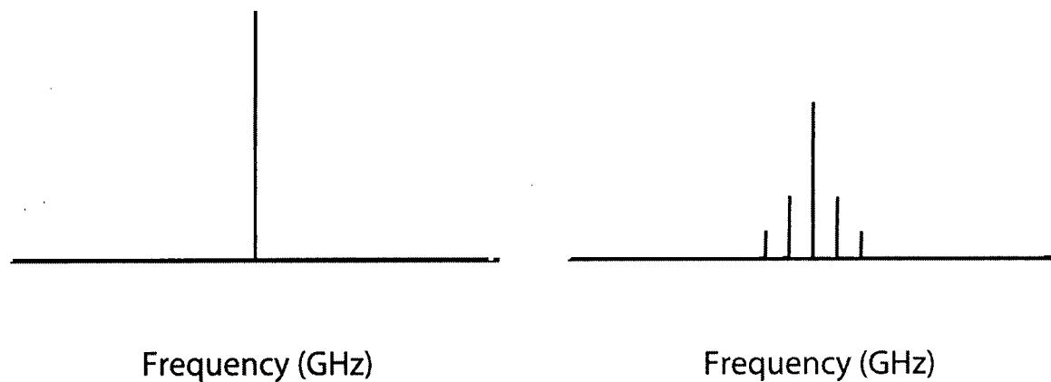
Figure 1-12: Illustrative optical power spectra when the laser is operating at constant power (left) and intentionally dithered using an external phase modulator (right), distributing the optical power over a number of subcarriers.
