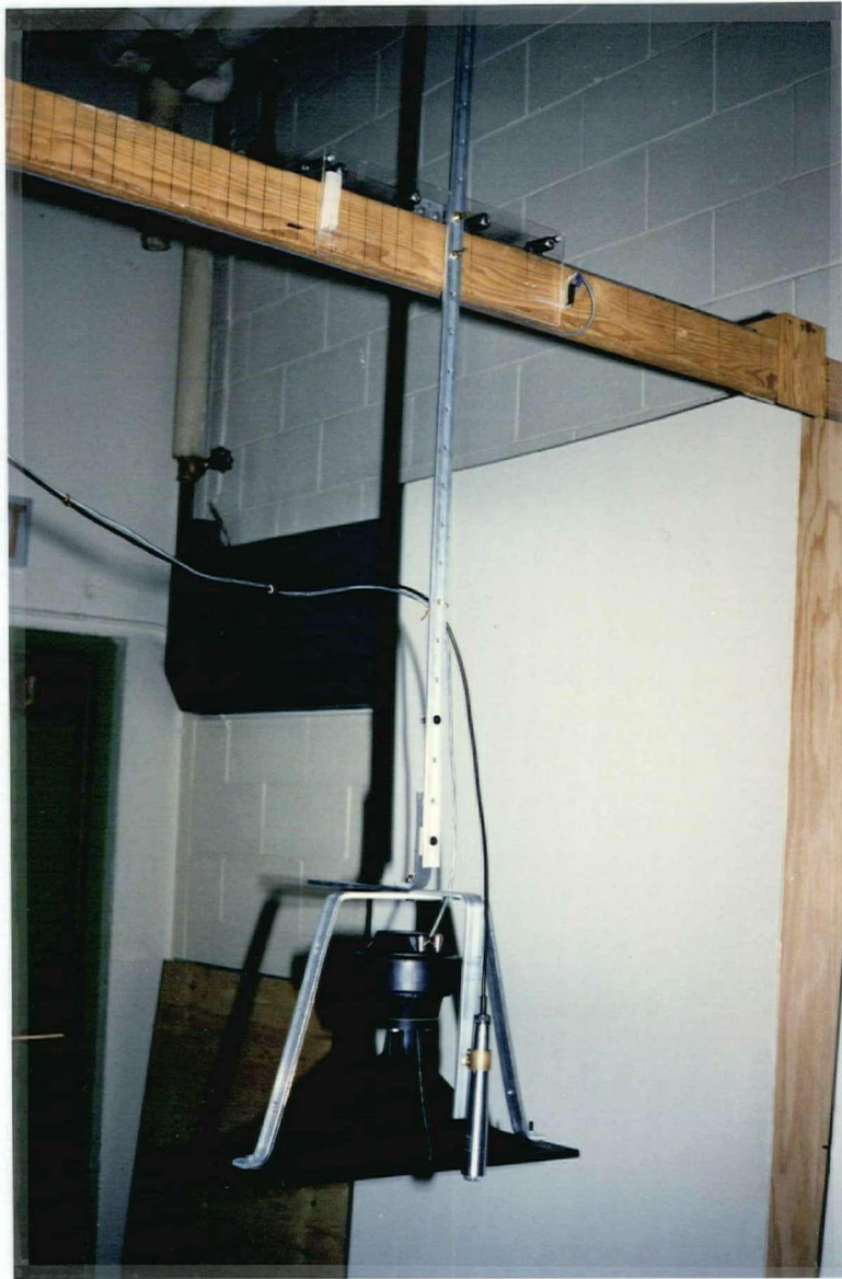
Fig. 3.2 Photograph of the Transducers as Mounted on the Trolley
