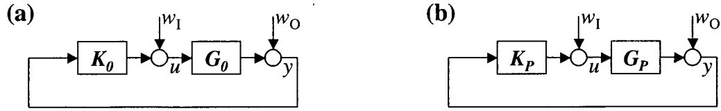
Figure 3.1: (a) Original and (b) modified closed-loop control systems.
