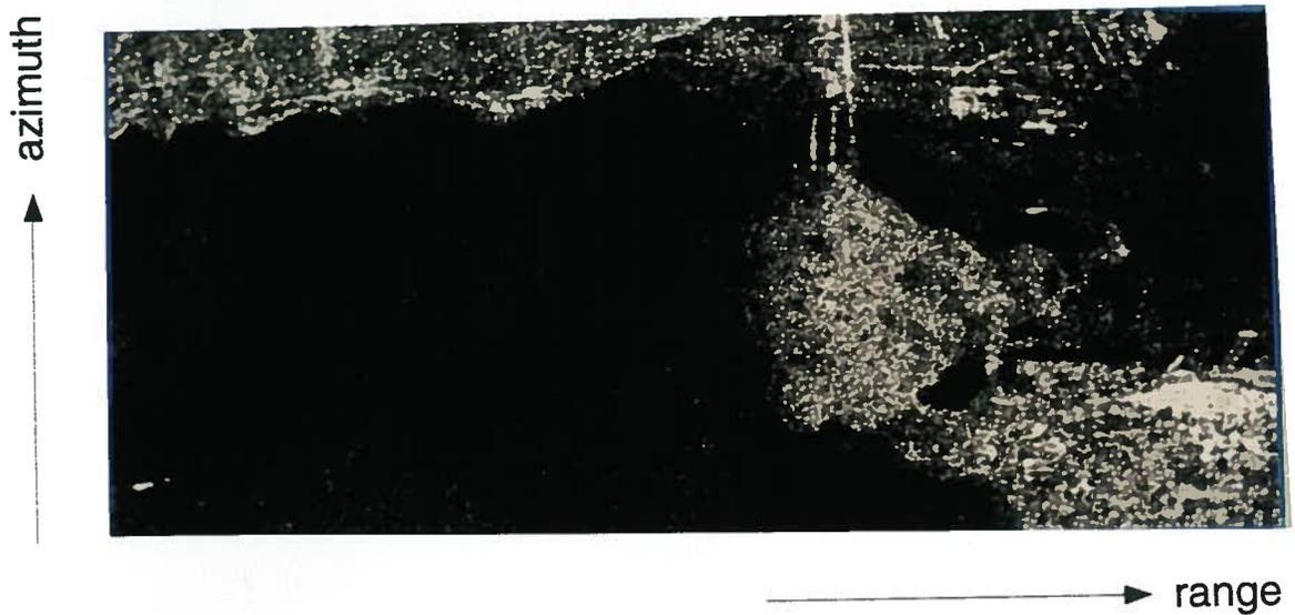
Figure 7.41: Image of Vancouver scene formed from skewed data with the original chirp scaling algorithm, with the reference range at the center of the image.
