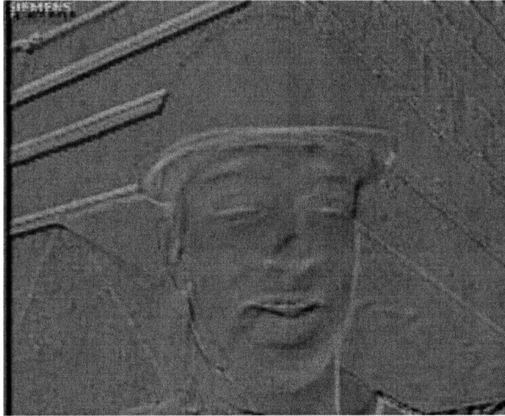
Figure 3.2: This image shows an example spatial difference image that is formed using the proposed scalability scheme. Notice how the image is composed of primarily high-frequency information.
