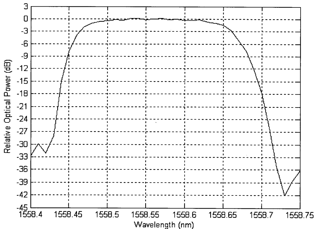
Figure B.2. The 3-dB pass-band of the filter was measured to be ~1558.47 nm to ~1558.66 nm.
