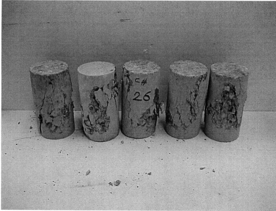
Figure 5.6 Tested Cylinders of Mix #26 (0.5% S_1 + 0.5% HPP)
