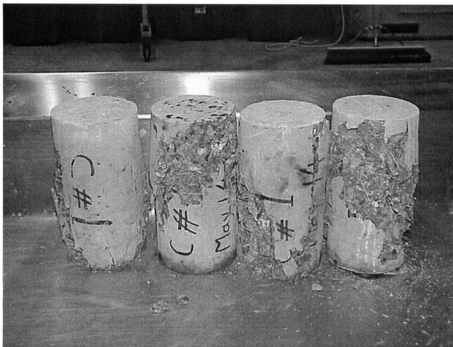
Figure 5.5 Tested Cylinders of Mix #1 (0.5% S 1 )
