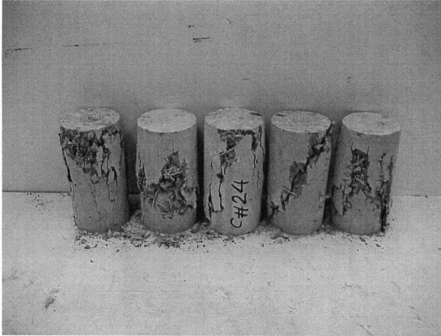
Figure 5.4 Tested Cylinders of Mix #24 (0.5% HPP)
