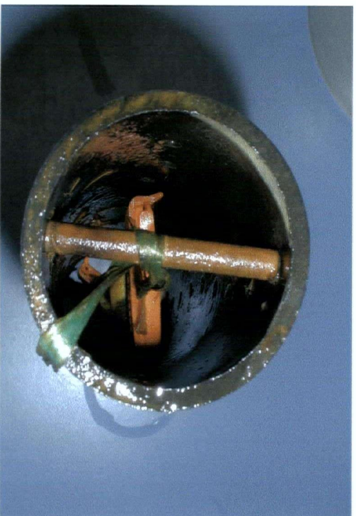
Photo A.11: XAD-7 resin pouch suspended through pipe in resin apparatus (June 7, 2002)
