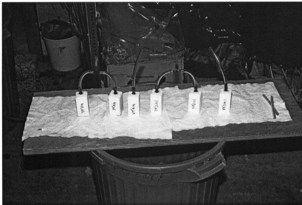
Figure 3.4 Photograph of 140 \mu fine pore diffusers
