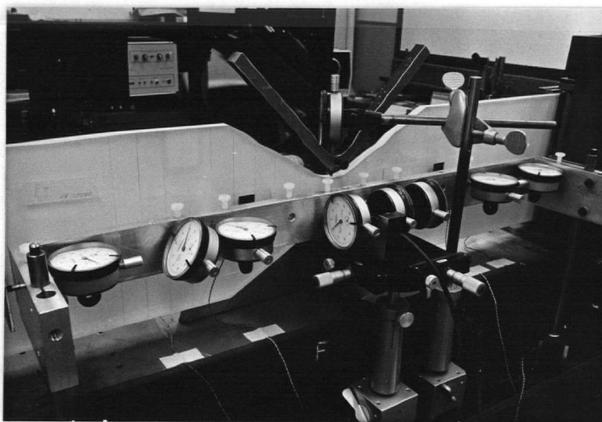
Fig. 5.14 Measurement of displacements u(y,0) by dial gages.
