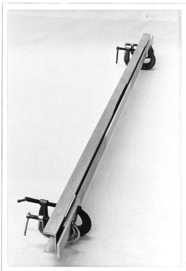
Fig. 5.10 The arrangement in bending of the beam experiments.
