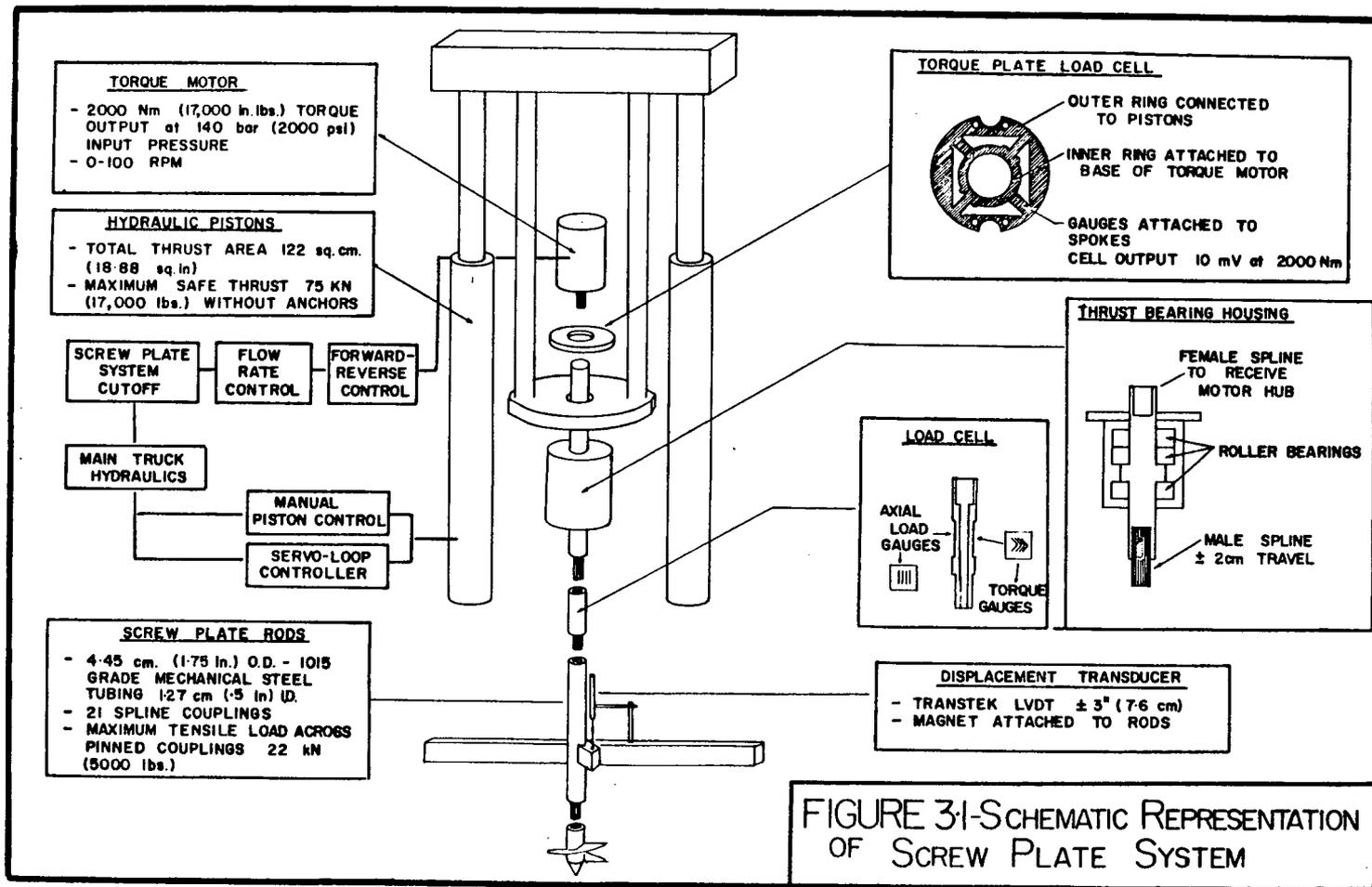
FIGURE 3-1-SCHMATIC REPRESENTATION OF SCREW PLATE SYSTEM
