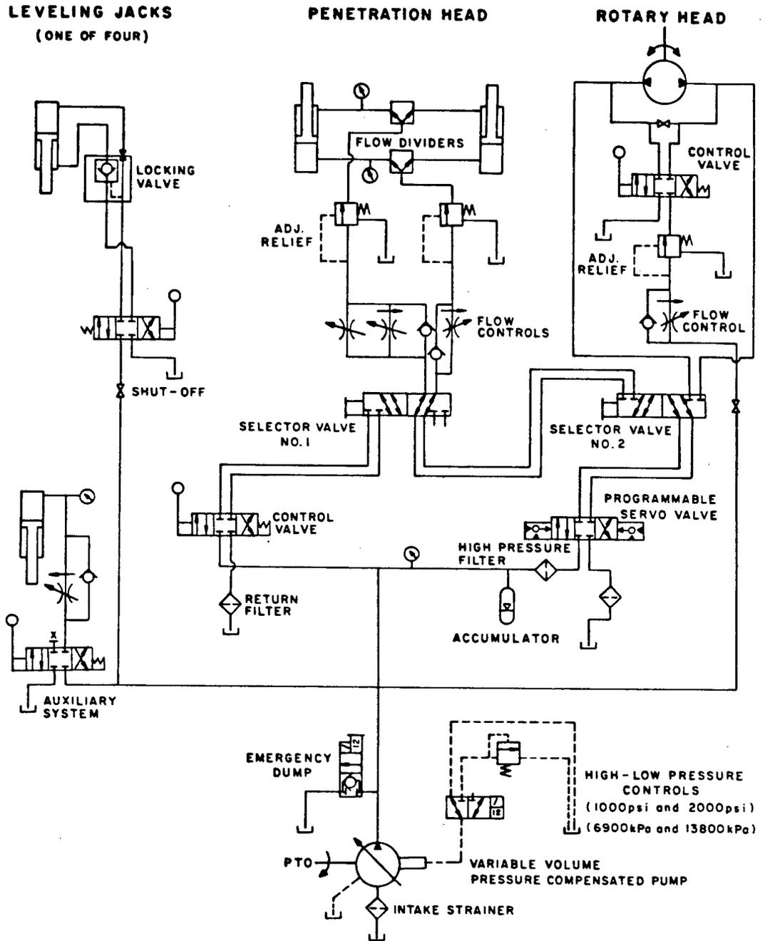
FIGURE 3-4 - SCHEMATIC OF HYDRAULIC CONTROL SYSTEM
