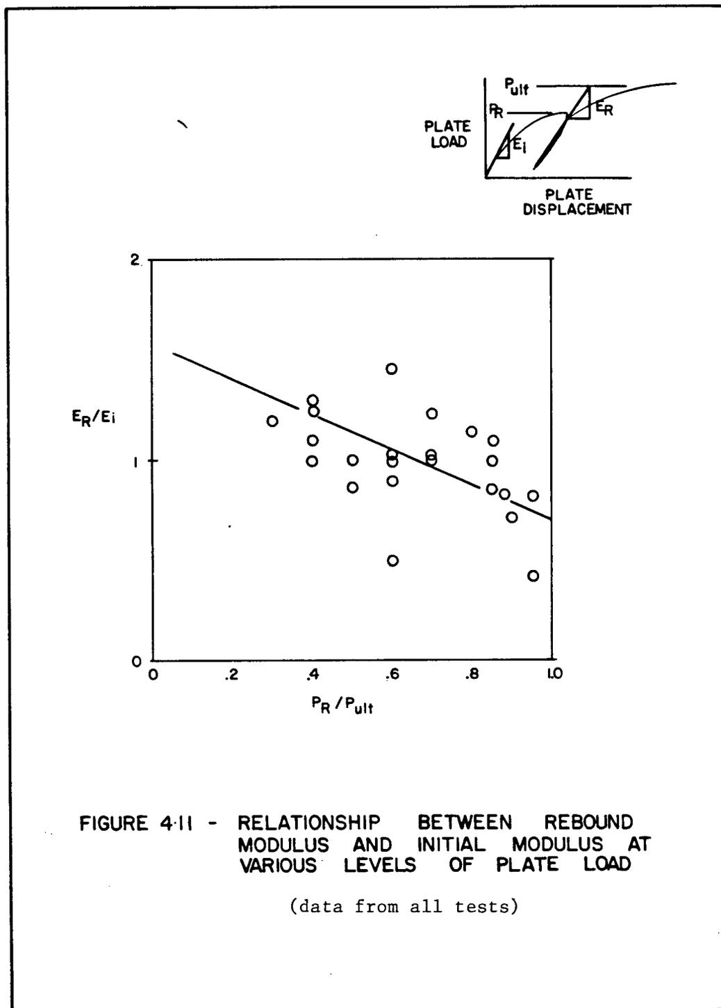
FIGURE 4-11 - RELATIONSHIP BETWEEN REBOUND MODULUS AND INITIAL MODULUS AT VARIOUS LEVELS OF PLATE LOAD
