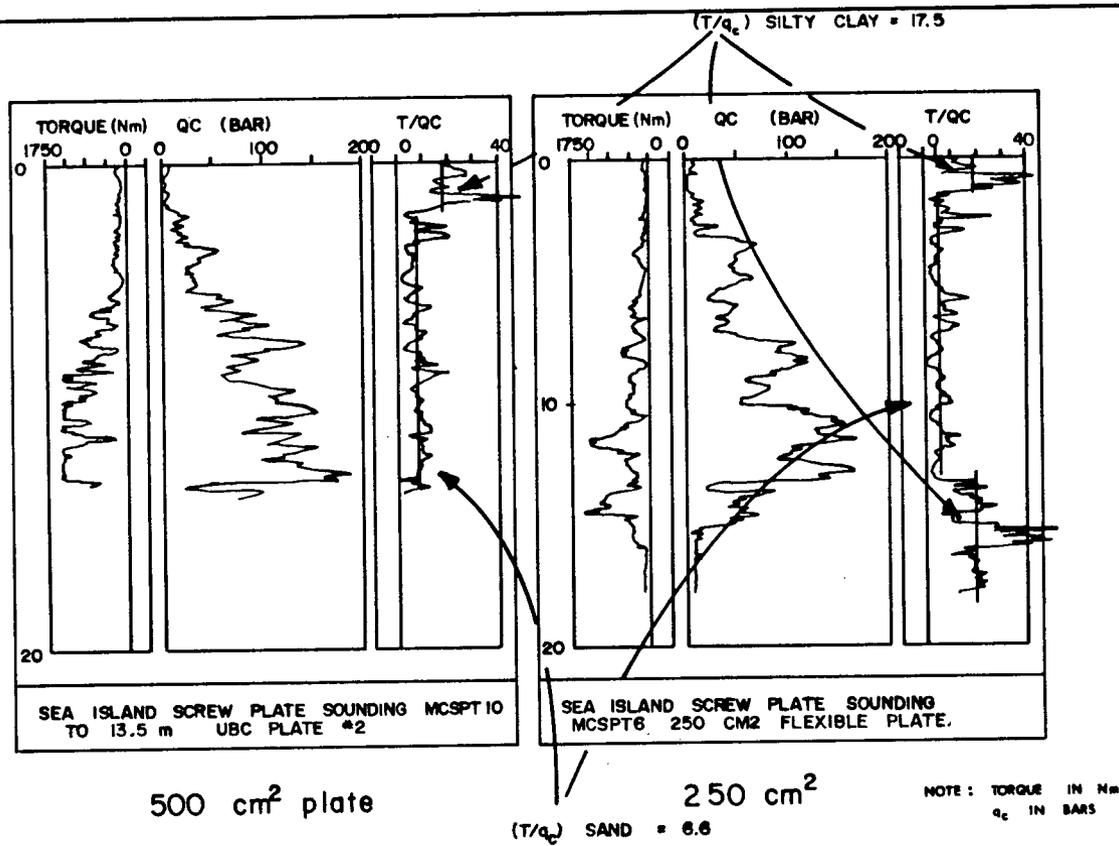
FIGURE 4-17 - RELATIONSHIP BETWEEN INSTALLATION TORQUE AND CONE RESISTANCE AT SAND AND SILTY CLAY SITE
