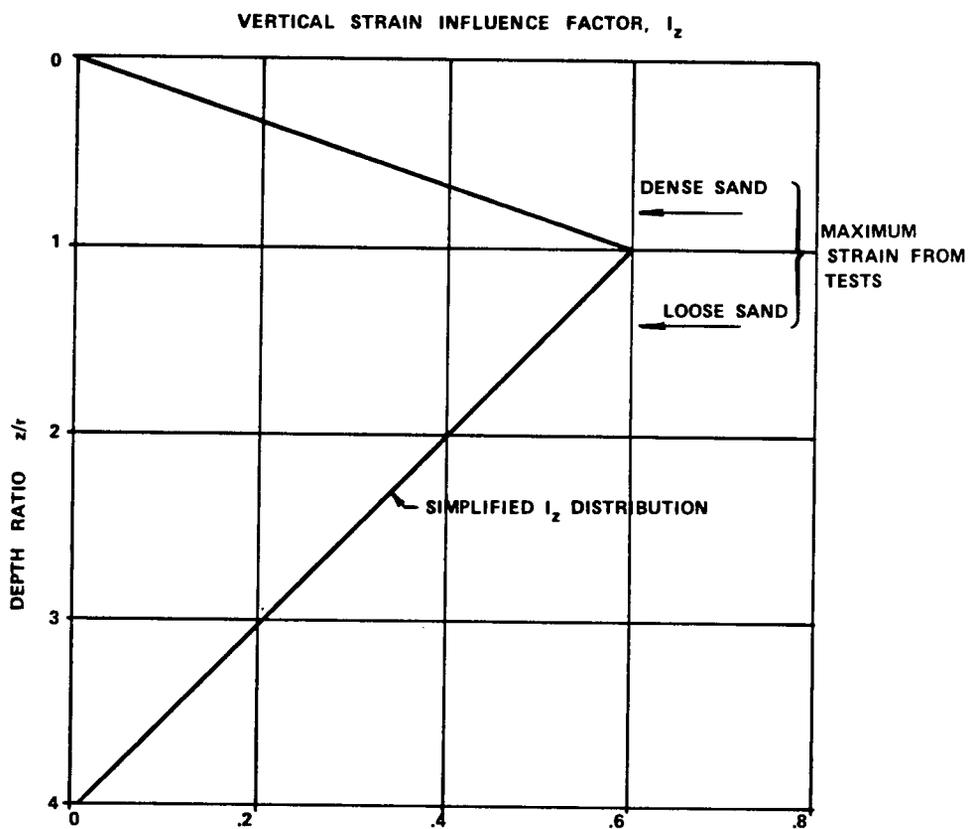
FIGURE 2-3 - SIMPLIFIED DISTRIBUTION OF VERTICAL STRAIN BENEATH LOADED CIRCULAR AREA
