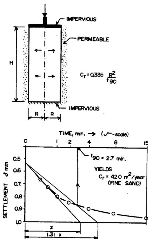
FIGURE 2.4- DETERMINATION OF COEFFICIENT OF CONSOLIDATION
