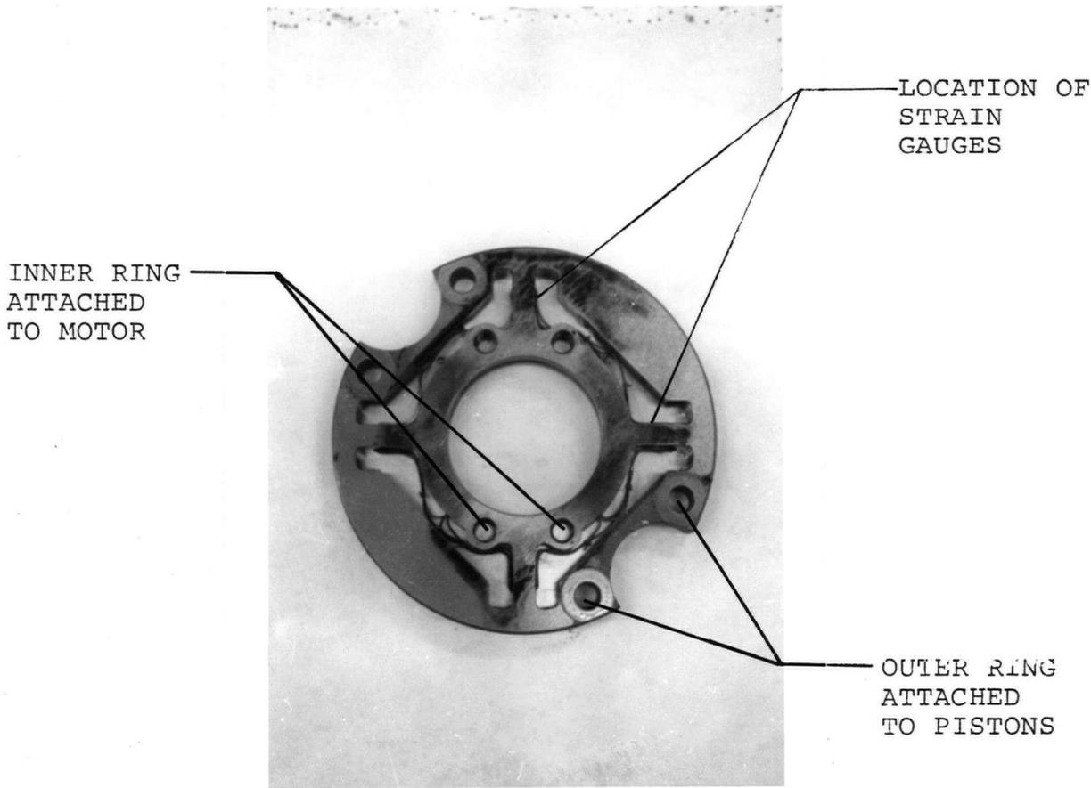
FIGURE 3.5 TORQUE LOAD CELL
