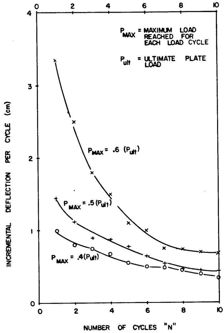
FIGURE 4.14 - INCREMENTAL PLASTIC DEFLECTION PER CYCLE
