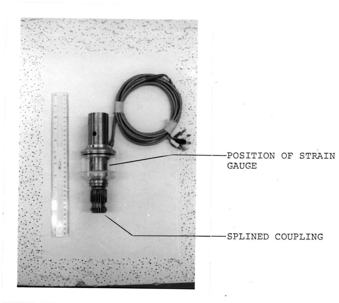
FIGURE 3.6 AXIAL LOAD CELL
