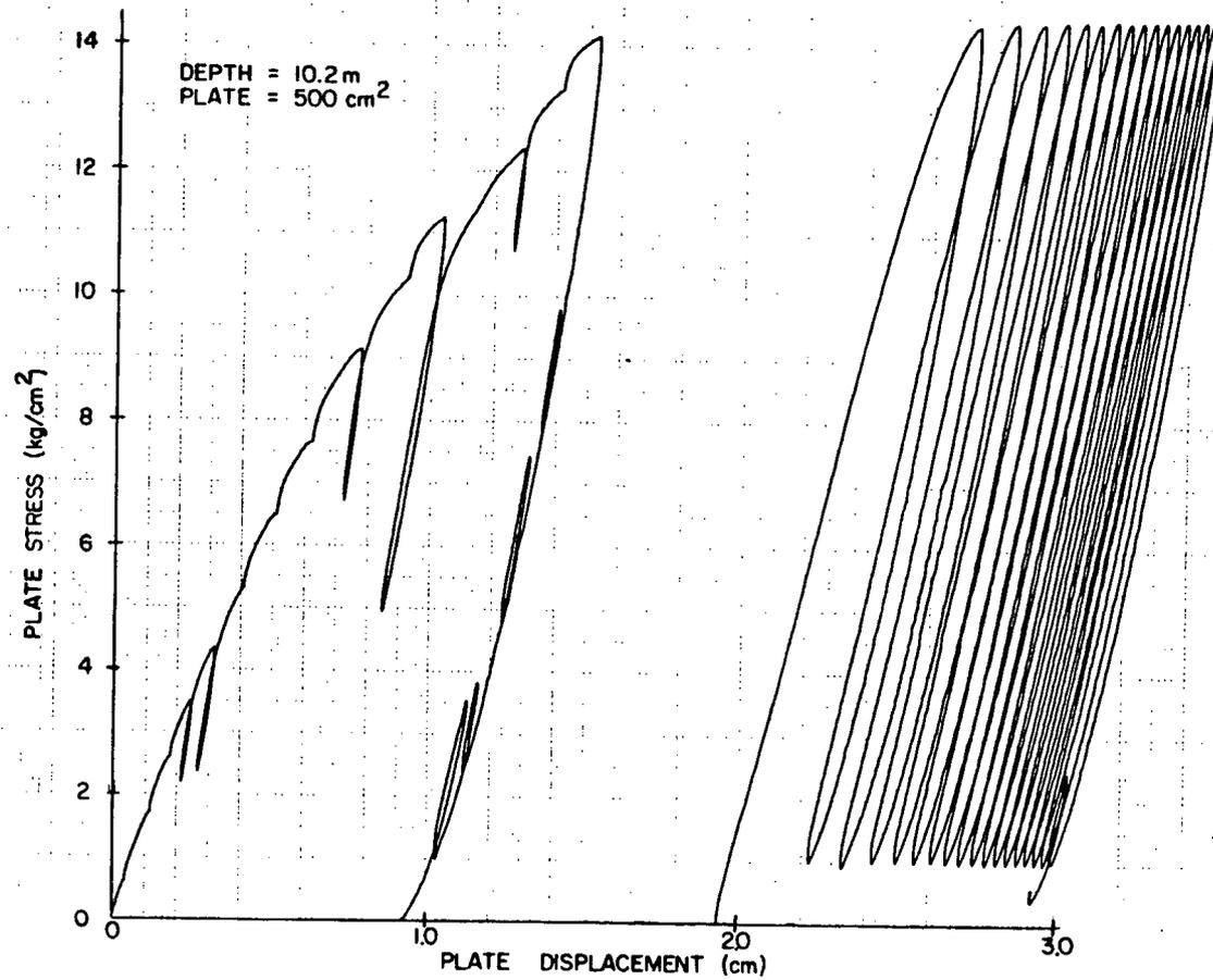
FIGURE 4.4-TYPICAL LOAD DISPLACEMENT CURVE IN SAND
