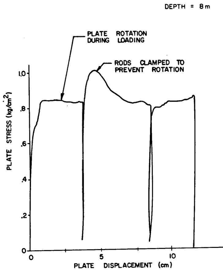
FIGURE 4-21 - EFFECT OF PLATE ROTATION DURING TESTING IN LANGLEY SENSITIVE CLAY
