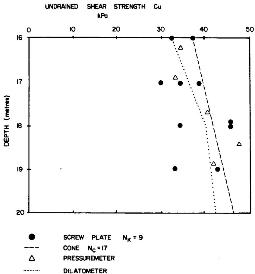
FIGURE 4.15 - COMPARISON OF UNDRAINED SHEAR STRENGTHS
