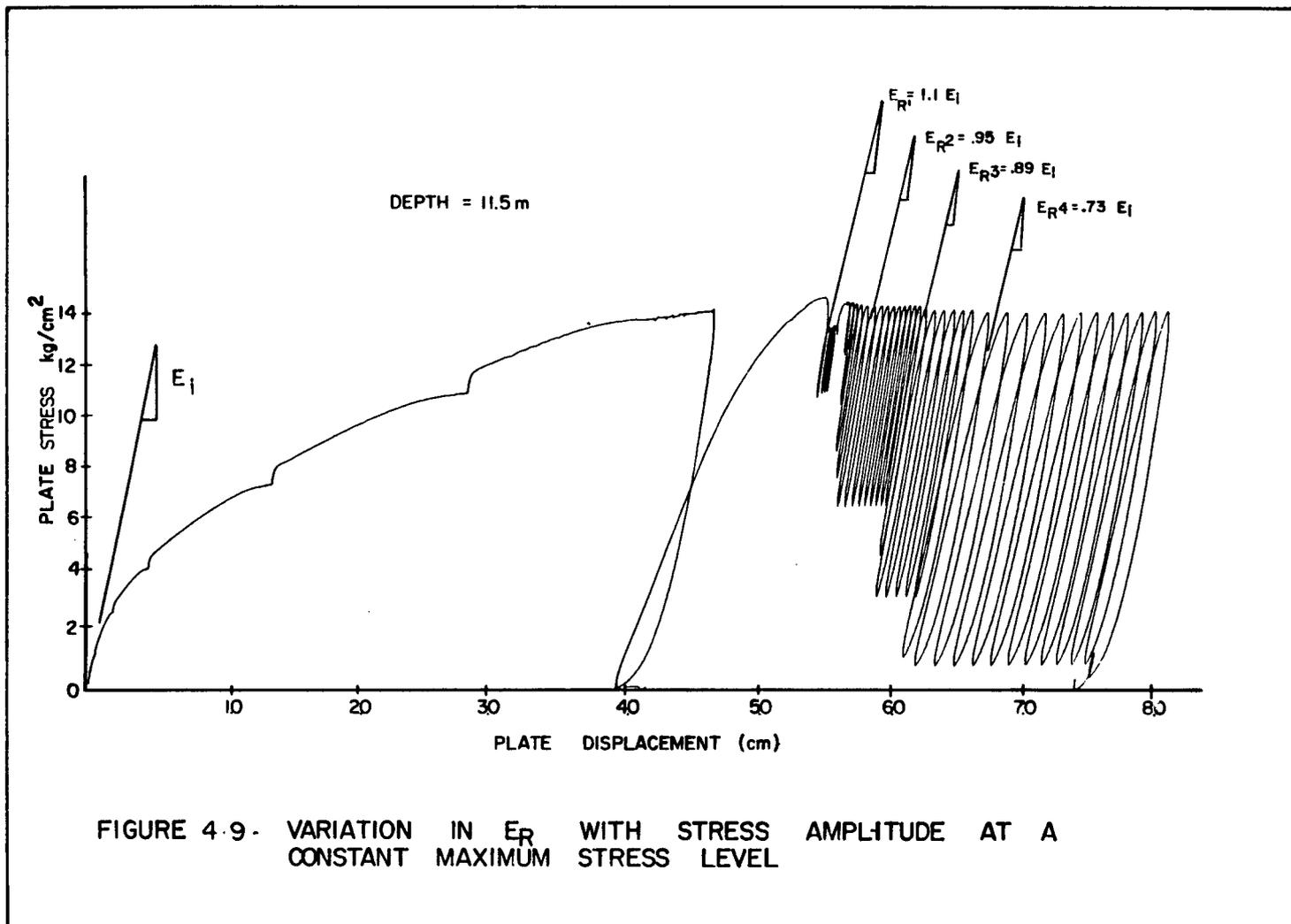
In this instance,  $E_i$  and  $E_R$  represent the slope of the stress displacement curve.
