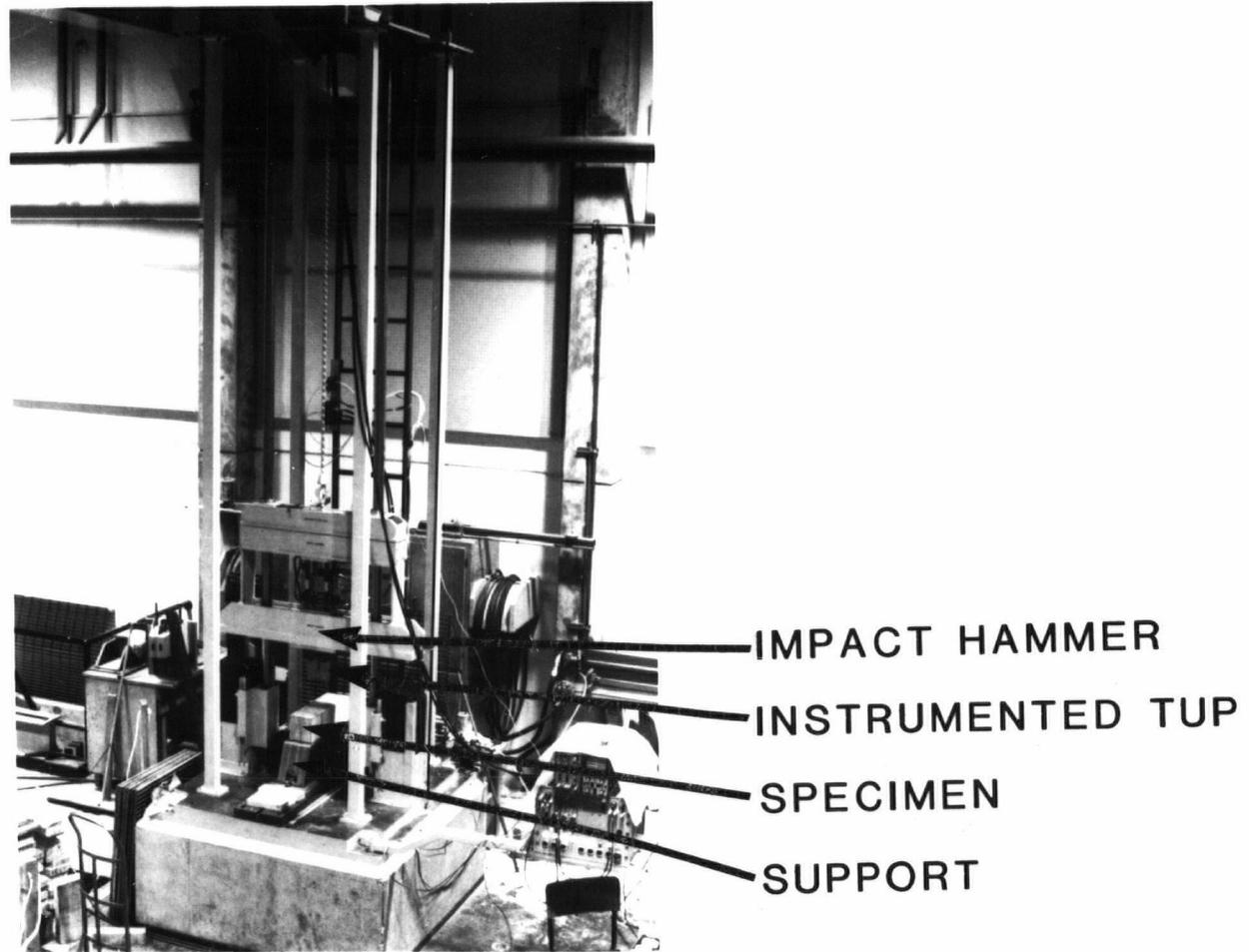
Figure 4.1-The Drop Weight Impact Testing Machine
