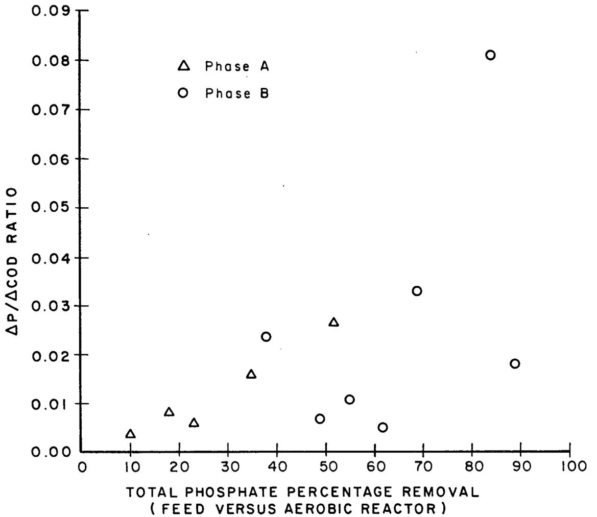
FIG. II - 3 :  $\Delta P/\Delta COD$  RATIO VS. %P REMOVED BY SYSTEM.
