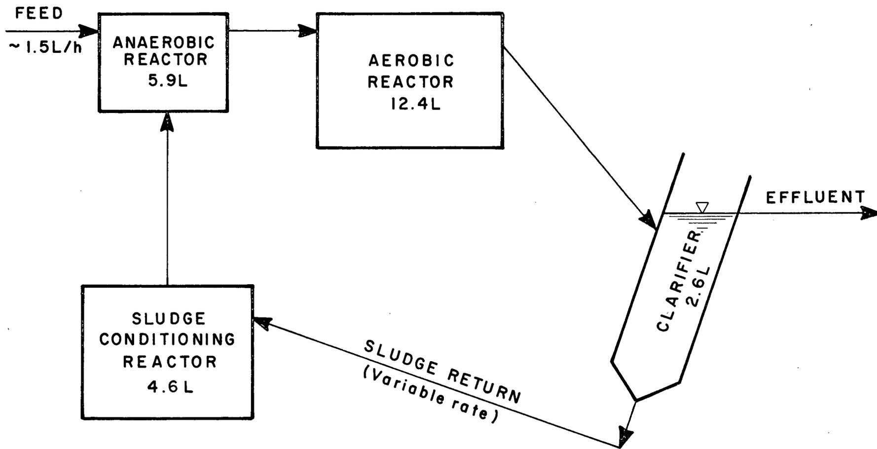
FIG. 3.9: MODIFIED PHOSPHORUS REMOVAL SYSTEM .
