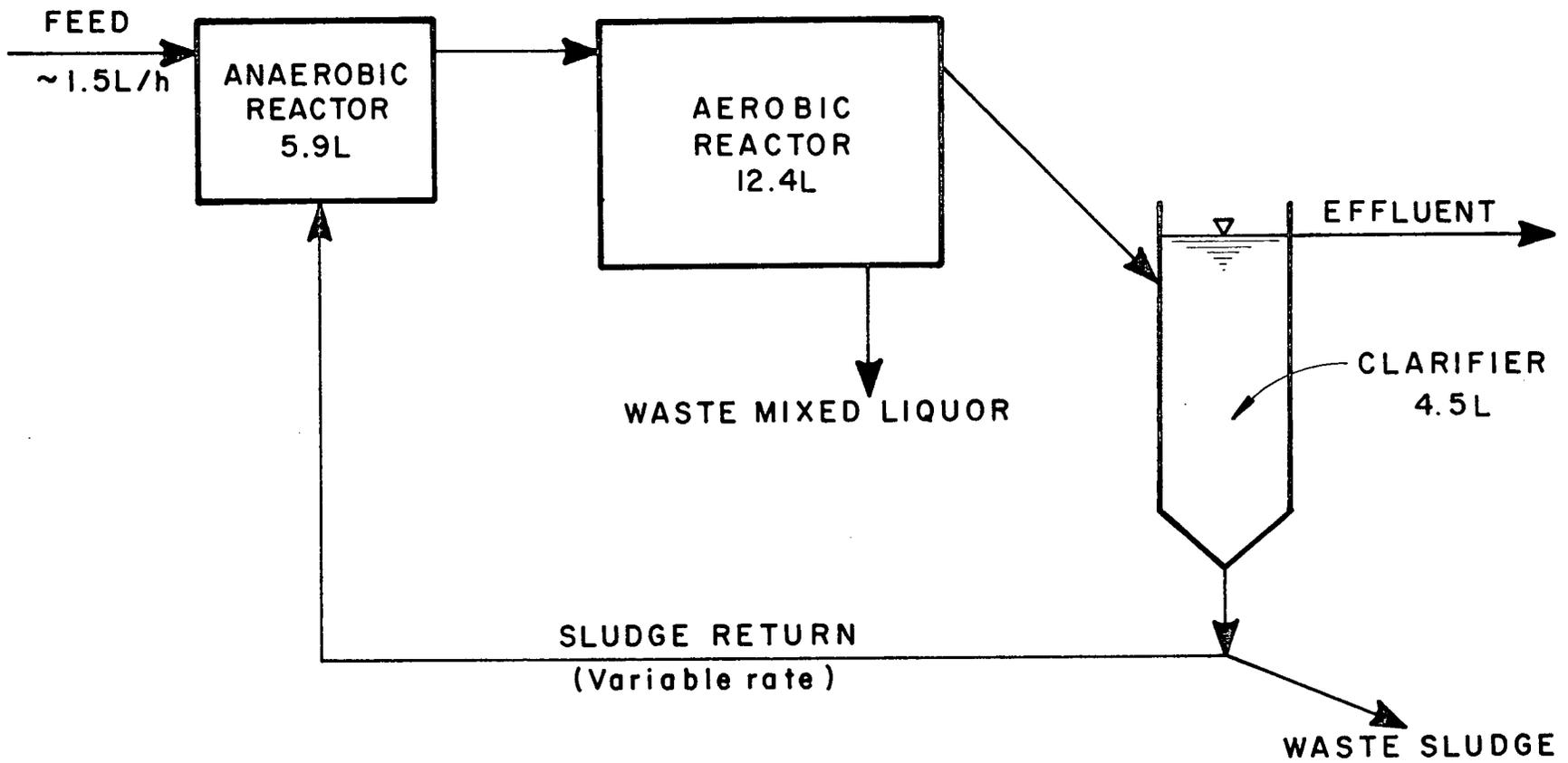
FIG.3.8: INITIAL PHOSPHORUS REMOVAL SYSTEM .
