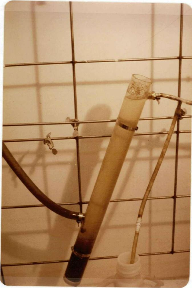
FIGURE 3.6: CLARIFIER (SUBSTITUTED MODEL)
