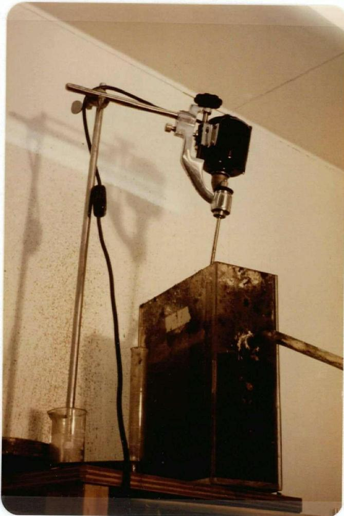
FIGURE 3.7: SLUDGE CONDITIONING REACTOR
