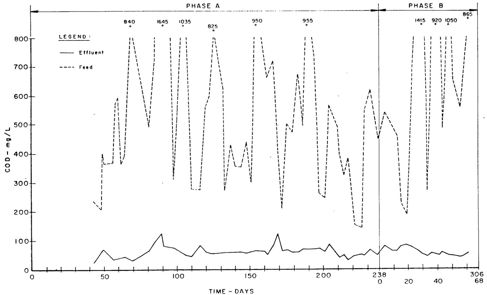
FIG. II-1: FEED AND EFFLUENT COD CONCENTRATION.
