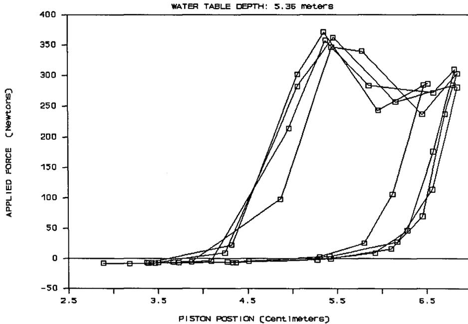
**Figure 14:** Force-displacement loop using the two-plate type piston.
