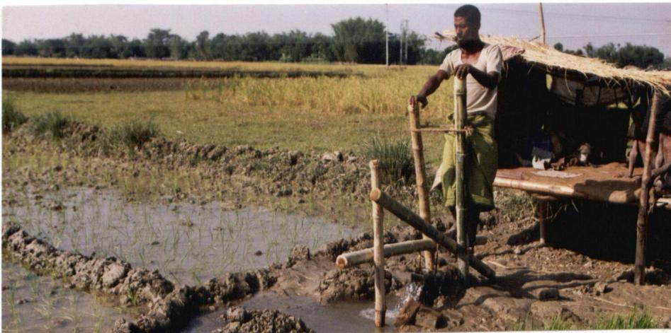
**Figure 7:** Field operation of the Treadle pump in Bangladesh.
