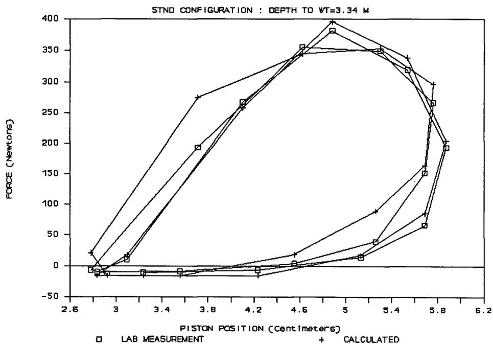
Figure 21: Comparison of calculated and laboratory results.
