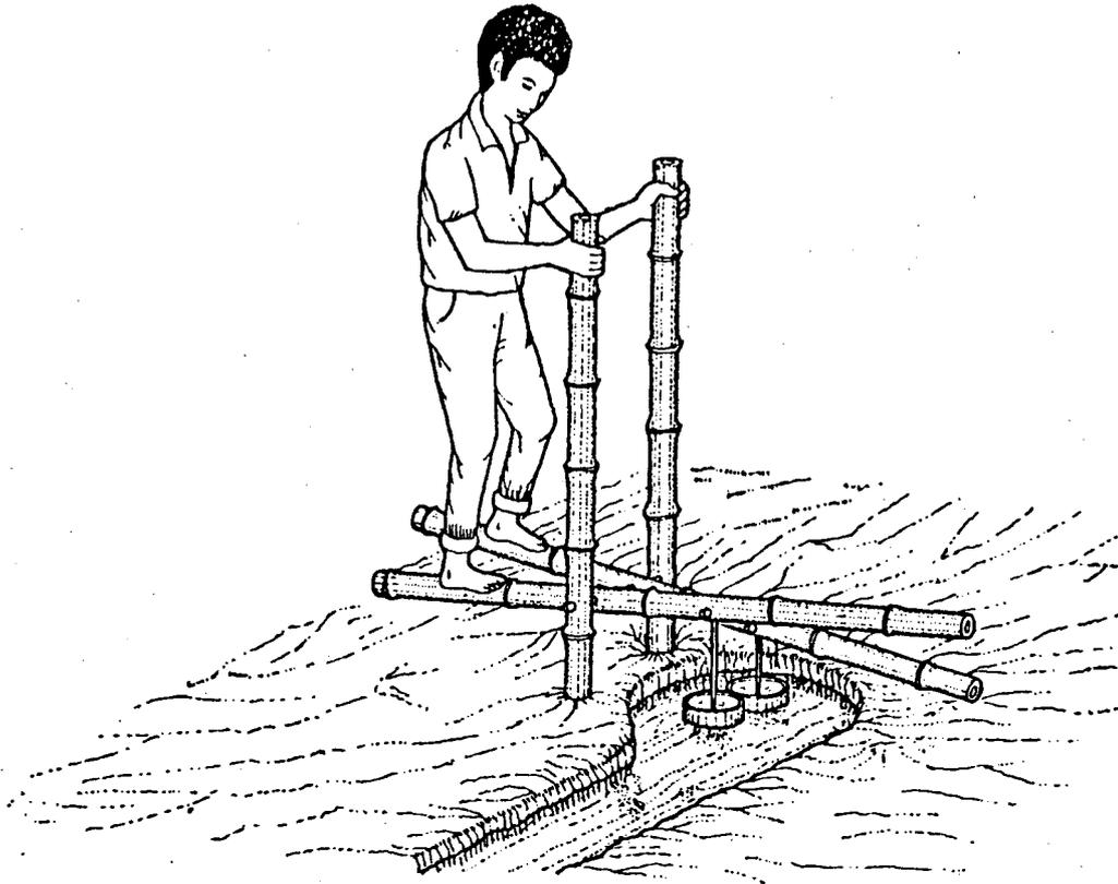
Figure 4: Centrally pivoted "dheki" type Treadle operation.
