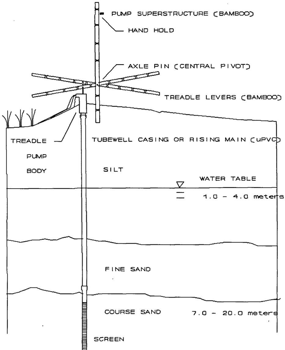
Figure 5: "Dheki" style field installation of the Treadle pump.
