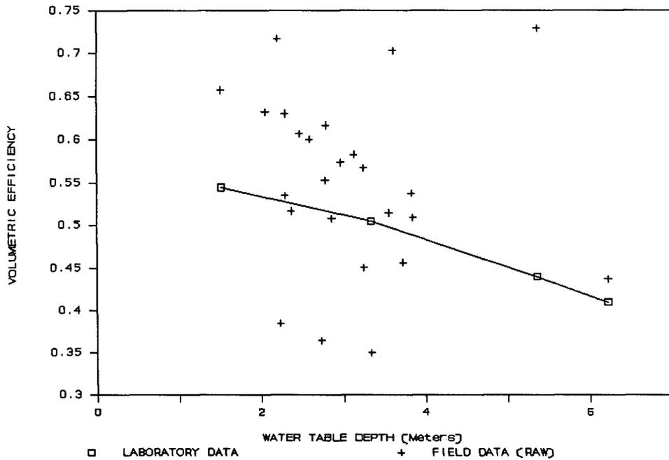
Figure 17: The effect of water table depth on volumetric efficiency.
