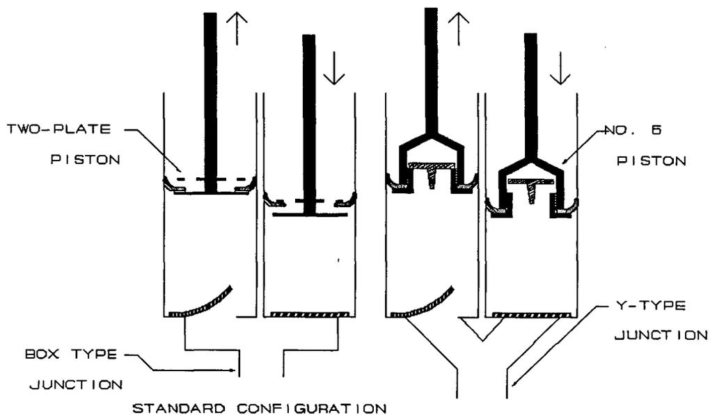
Figure 6: The two piston configurations, the two-plate design and the No. 6 style piston, and the two types of junctions.
