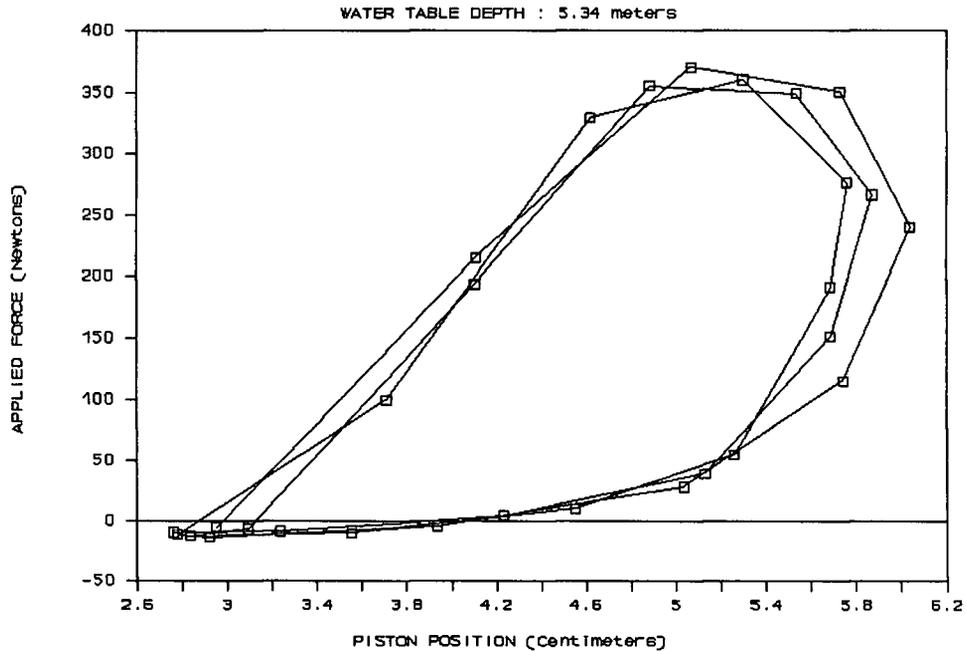
Figure 15: Force-displacement loop using the No.6 type pistons.
