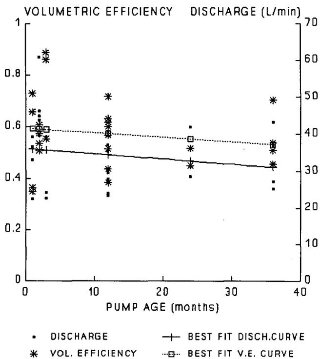
Figure 19: Effect of pump age on volumetric efficiency and discharge from field tests.
