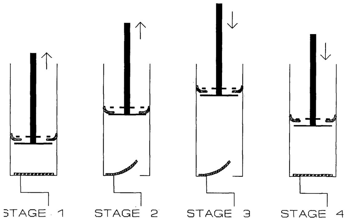
Figure 8: The pump cycle defined by valve positions.
