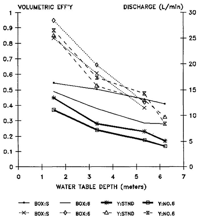
Figure 20: Effect of pump configuration on laboratory measured volumetric efficiency and discharge.
