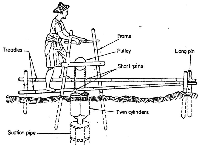
Figure 3: Rope and pulley type Treadle operation.
