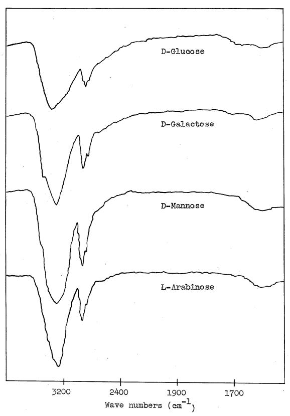
The infra-red absorption was measured in a Perkin-Elmer Recording Spectrophotometer using pressed potassium bromide pellets.
