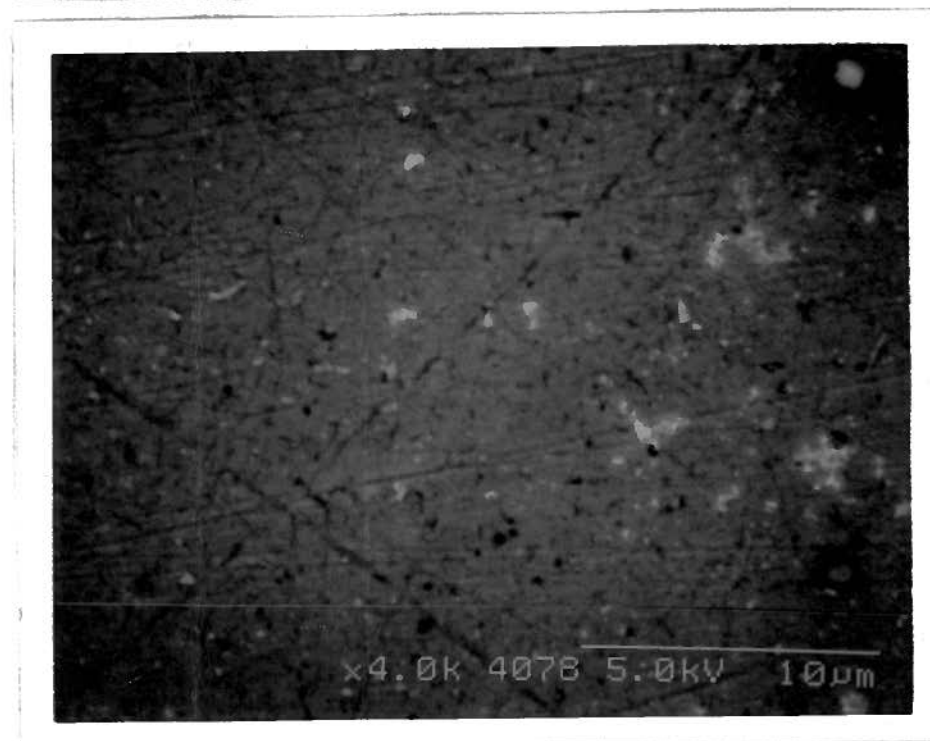
Figure 3.10 SEM micrographs of : (a) sample A, blank aluminum; (b) sample A1, sample A after corrosion; (c) sample C, ZPO treated aluminum; (d) sample C1, sample C after corrosion.
