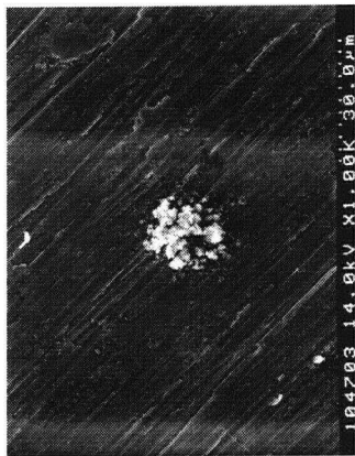
(a) blank sample (x1000) shows corrosion product
