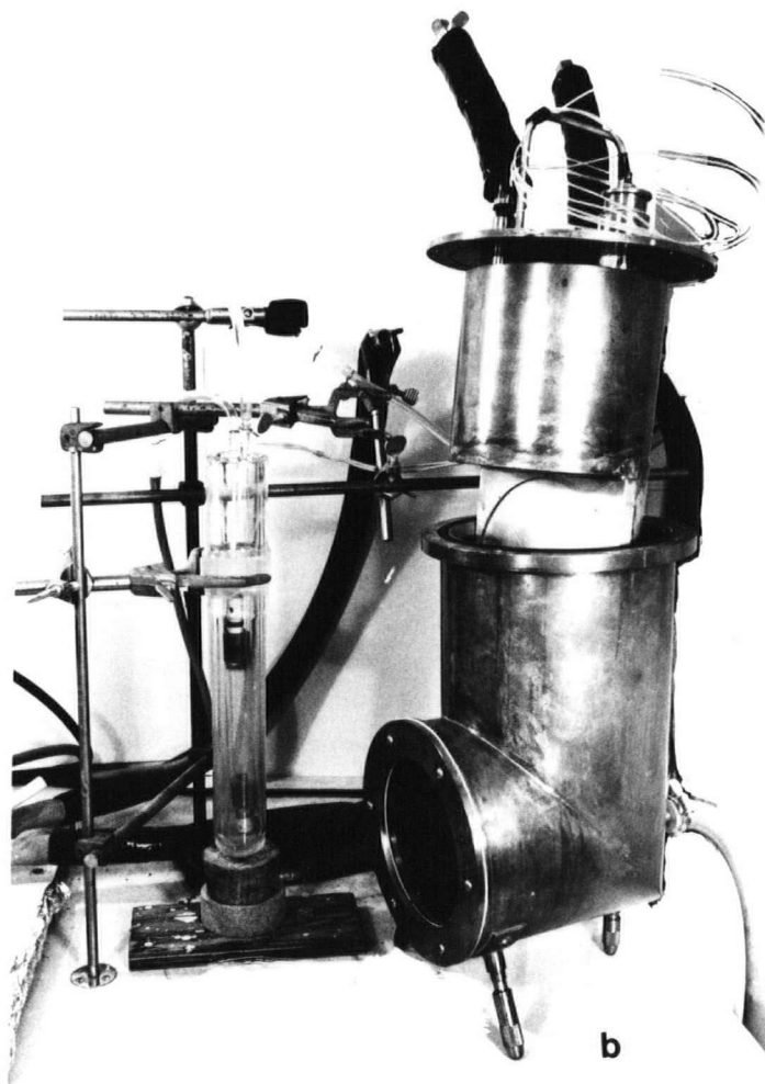
Figure 31. Apparatus for Irradiations in the Solid State. (a) Part A; (b) Part A being inserted into Part B.
