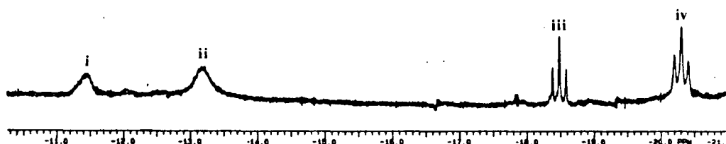
Figure 4.16 The upfield ^1\text{H} NMR spectrum (300 MHz, toluene- d_8 / n -butanol, ambient temperature) of in situ products from the reaction of 3a with \text{H}_2 , after 6 h from mixing; resonances 'i' - 'iv' are discussed in the text.
