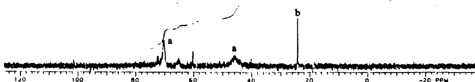
Figure 4.27 The 31 P{ 1 H} NMR spectrum (121 MHz, 1:1 v/v DMA/C 6 D 6 , 5 °C, under hydrogen), acquired within 2 h of starting the reaction, of the 1a-catalytic hydrogenating solution containing initially 0.04 M 1-hexene. Peaks marked 'a' are due to 1a; peak 'b' is due to Ph 3 PO; other peaks are unidentified.
