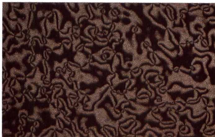
Figure 1-5: Texture of a nematic liquid crystal 1
