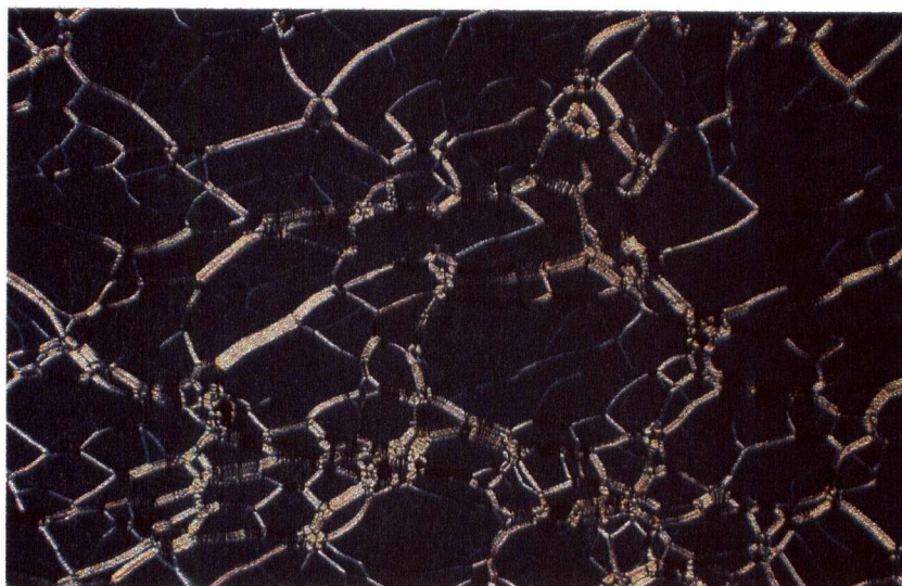
Figure 1-7: Texture of a chiral nematic liquid crystal 1
