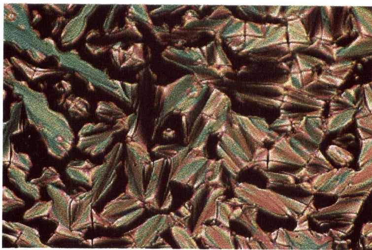
Figure 1-9: Texture of a smectic A liquid crystal 3
