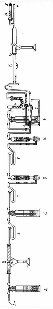
Purification Train for Gases and "Bottling Apparatus"
