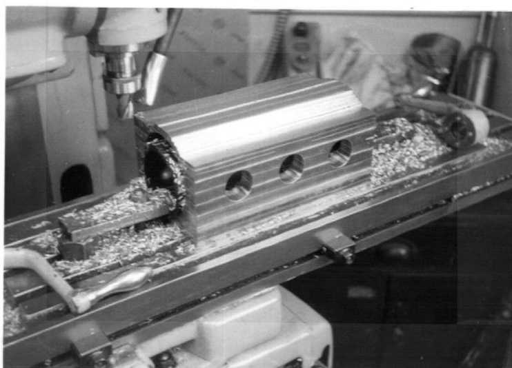
Figure 10. Reduction of Weight of Piston Block
