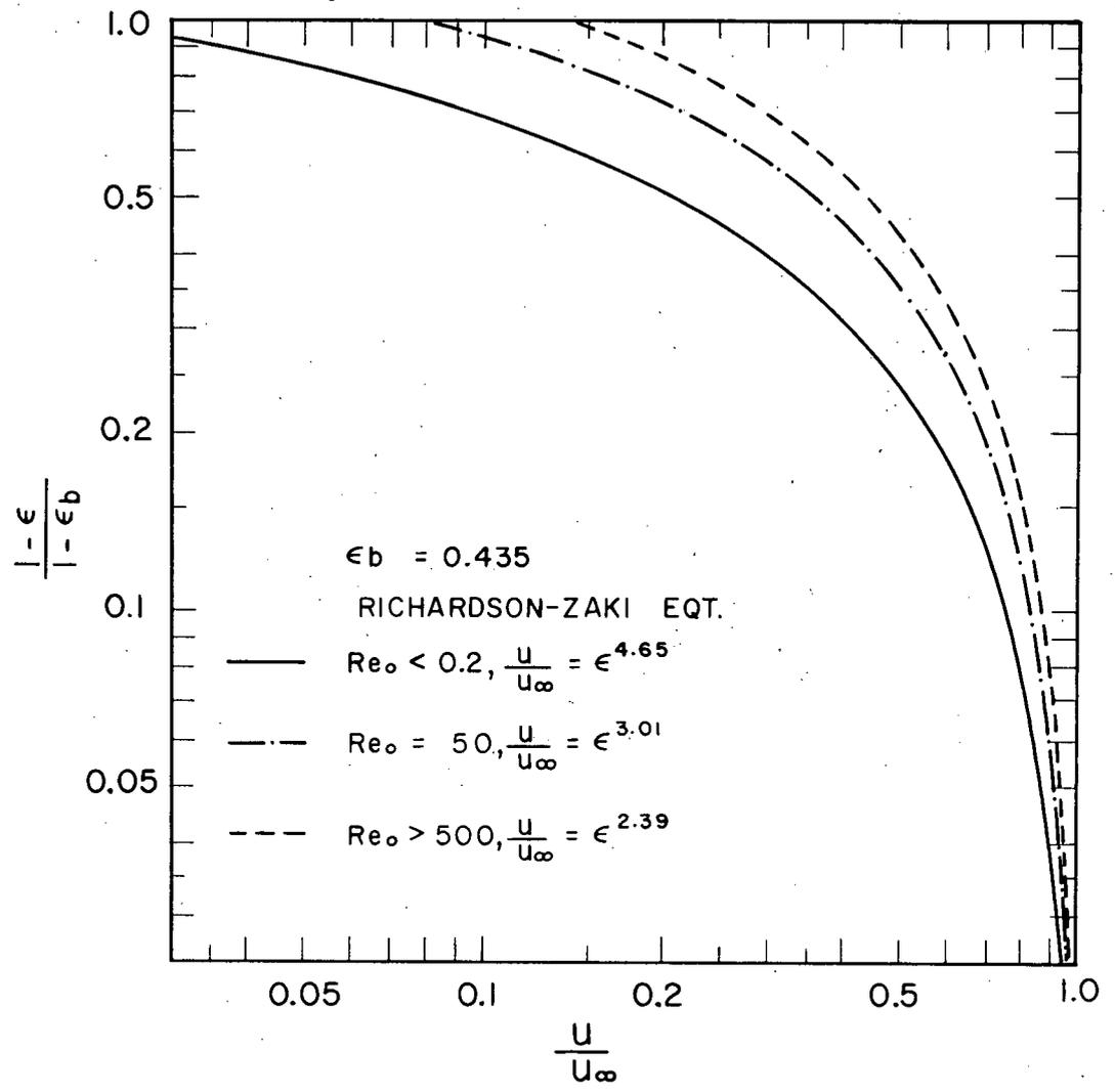
Figure 2. Beranek-Klumpar Plot based on Richardson-Zaki Empirical Equations
