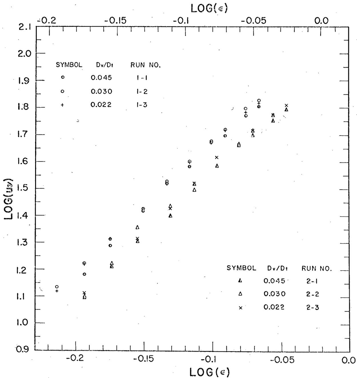
Figure 9. Wall Effect on Glass Bead Settling
