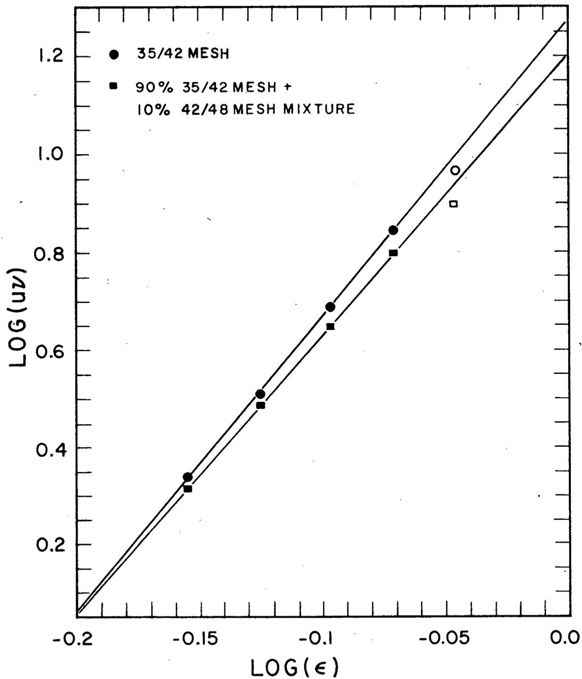
Figure 3. Comparison of Settling Rates of Different Size Distributions of Particles
