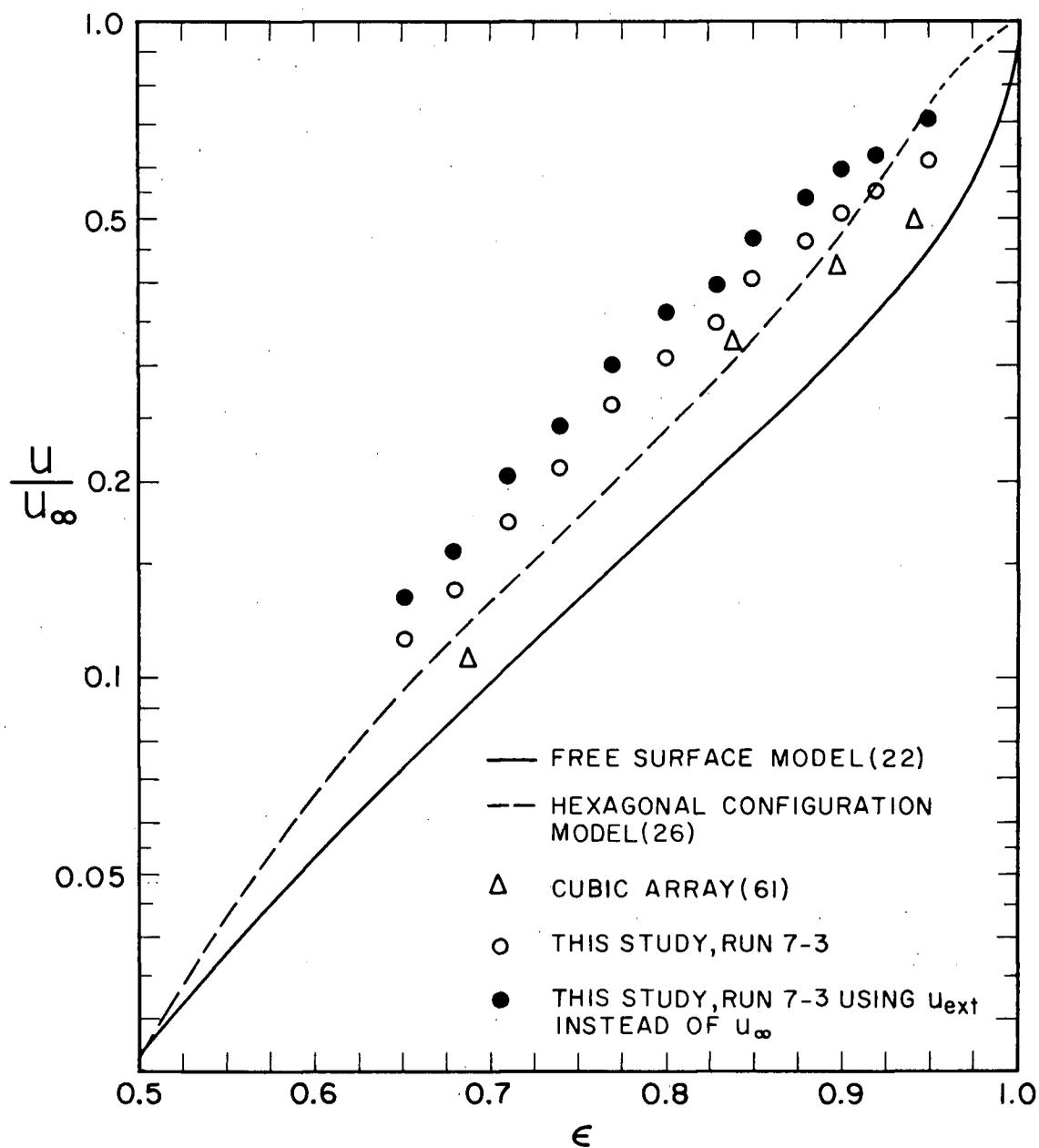
Figure 18. Comparison of the Present Results for Spheres to Models in the Literature
