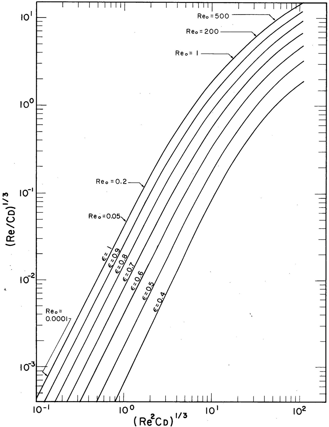
Figure 1. Modified Plot of  $C_D$  -  $Re$  for Single Particle and Suspension
