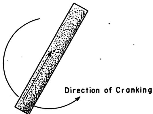
Figure 7. Illustration of Suspension Circulation
