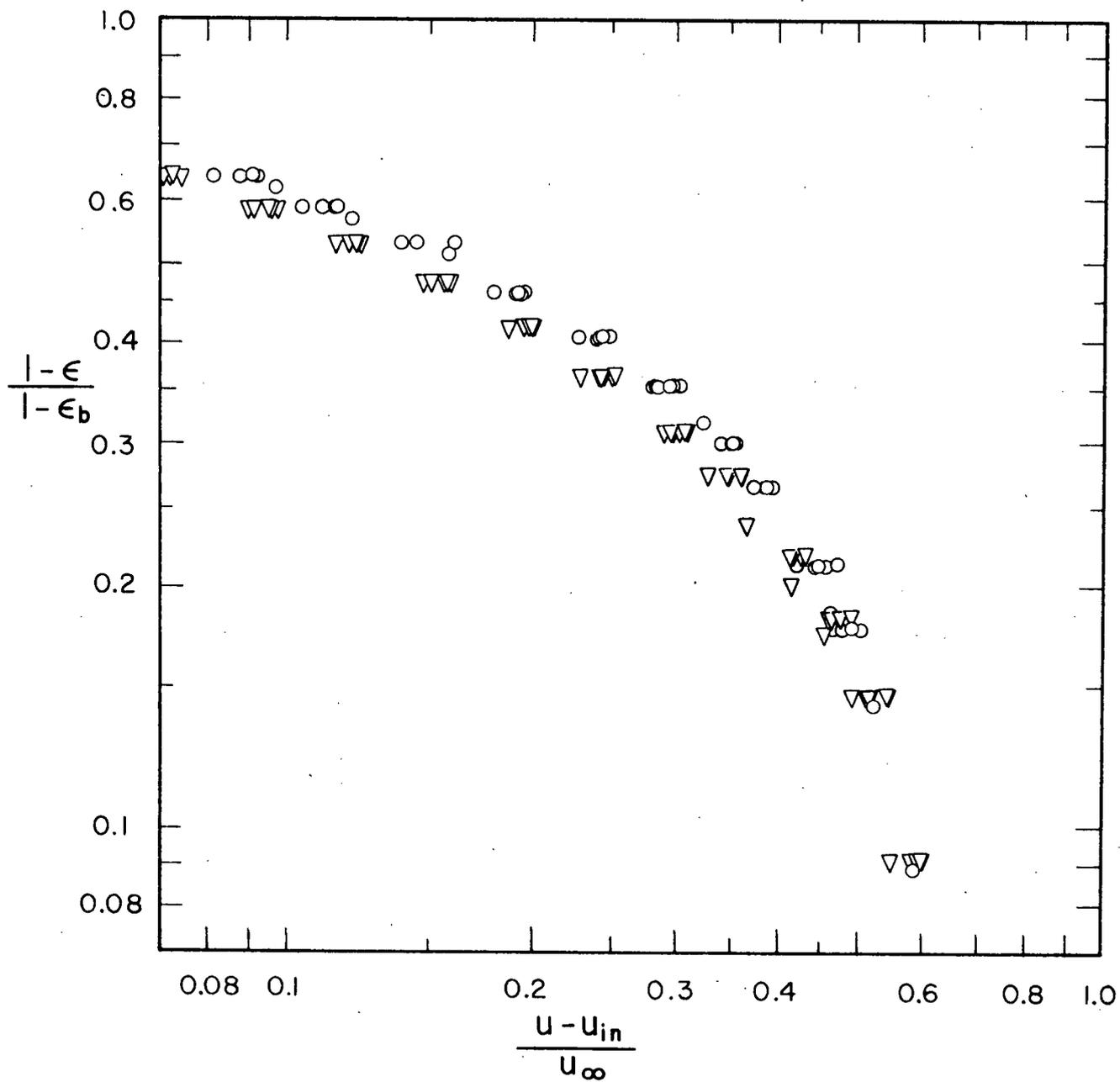
Figure 16c. Beranek-Klumpar Plot using  $(u-u_{in})/u_\infty$
