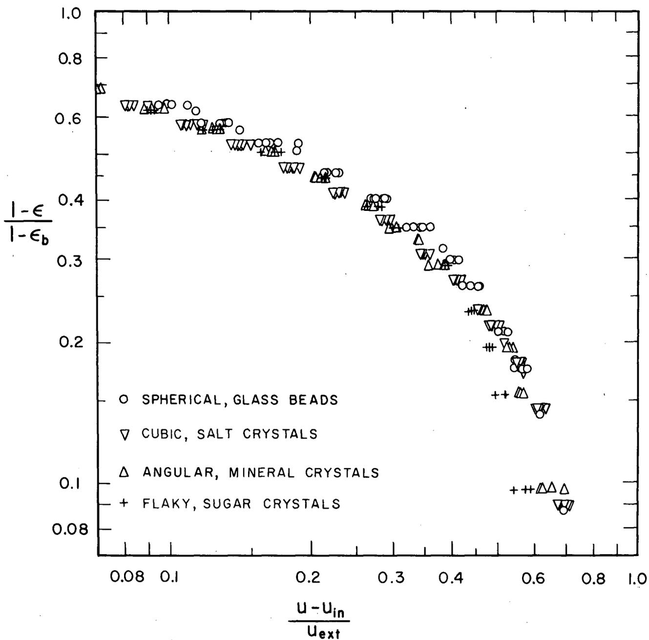
Figure 16a. Beranek-Klumpar Plot using  $(u-u_{in})/u_{ext}$
