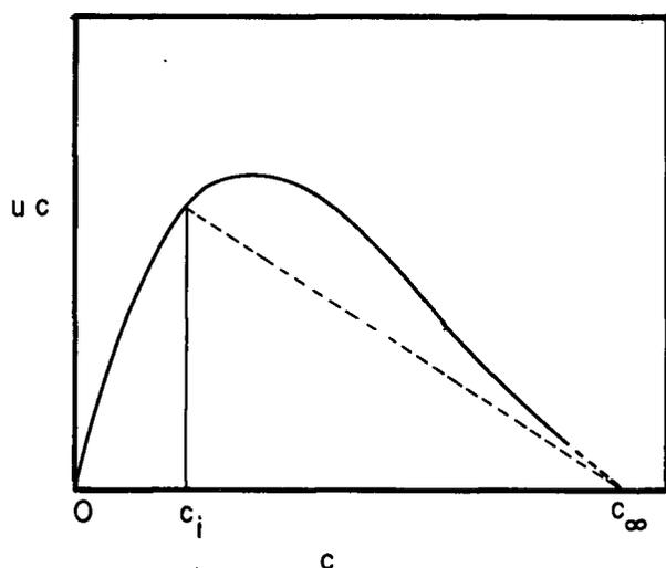
Figure I-1. Sedimentation Flux Plot, Single Concave
