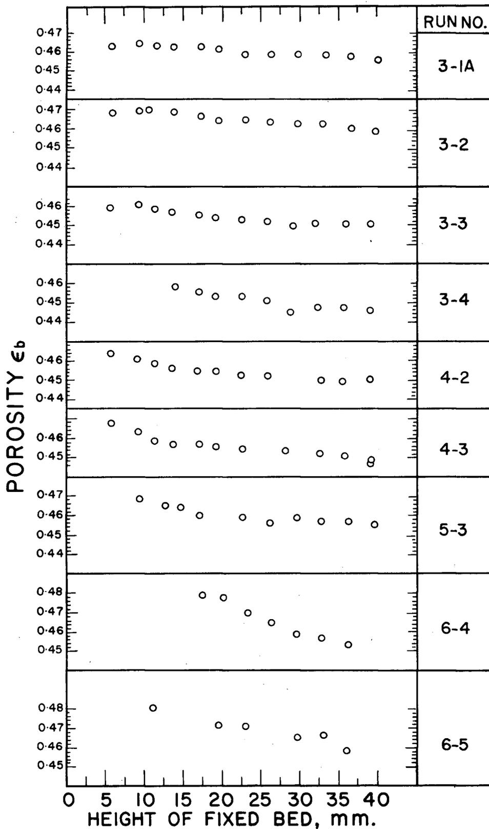
Figure 15b. Settled Bed Porosity of Cubic Particles
