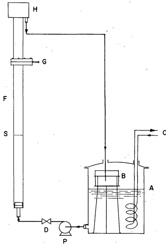
Figure 4. Schematic Drawing of Liquid Elutriation Apparatus
