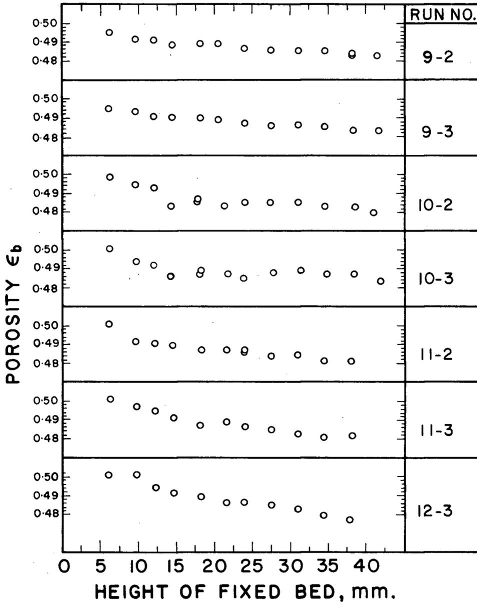
Figure 15c. Settled Bed Porosity of Mineral and Sugar Crystals
