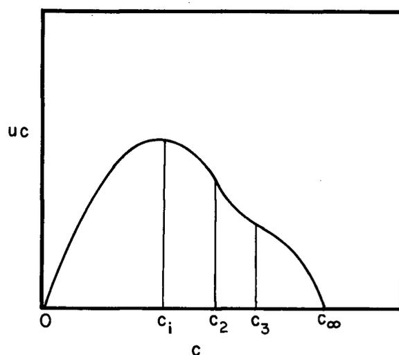
Figure I-2. Sedimentation Flux Plot, Double Concave
