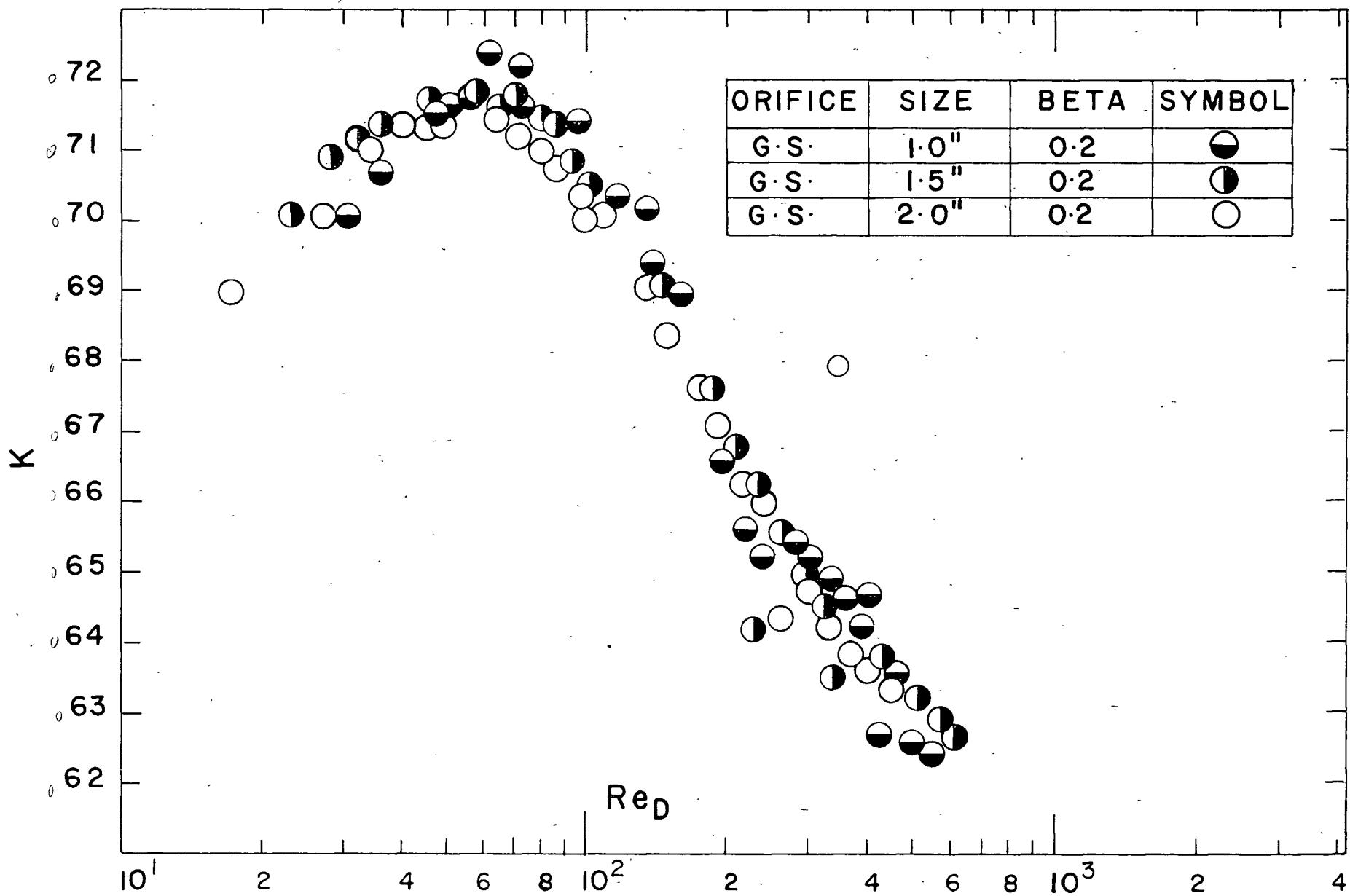
FIGURE 15: CALIBRATION RESULTS - G.S.,  $\beta = 0.2, 1.0, 1.5$  AND 2.0 INCH TEST LINES
