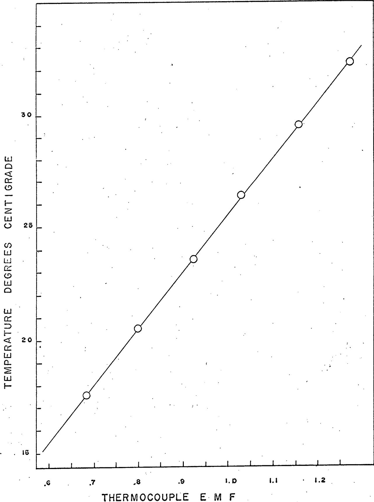
FIGURE 4-5 CALIBRATION OF THERMOCOUPLE 5
