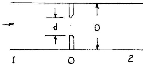
Fig. 9 Schematic Drawing of an Orifice Plate for
