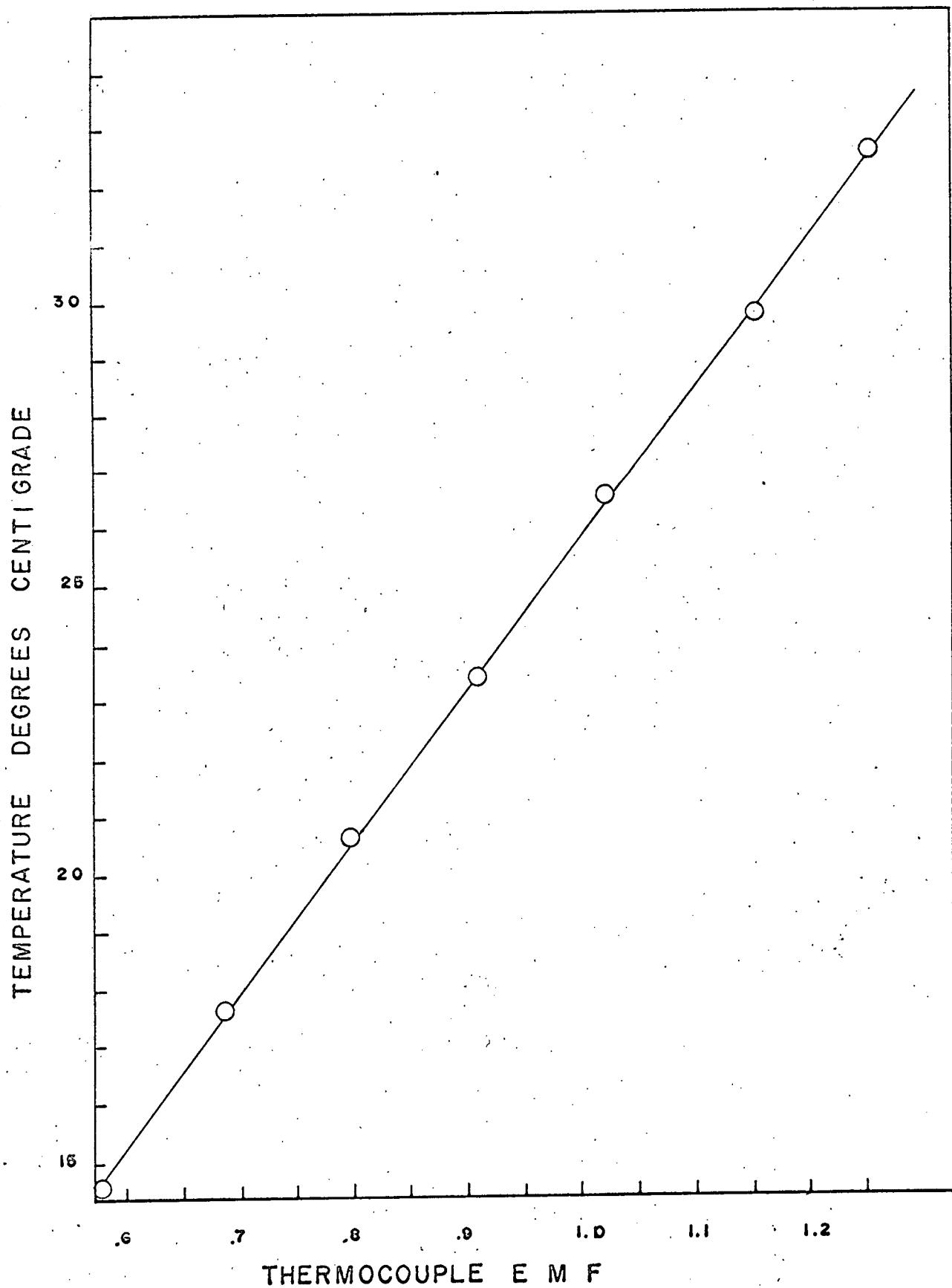
FIGURE 4-1 CALIBRATION OF THERMOCOUPLE I
