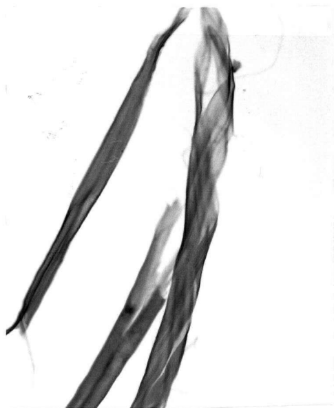
Figure 5.7: Examples of fibre damage (x100) a. Unraveled end b. Pulled back to a point
