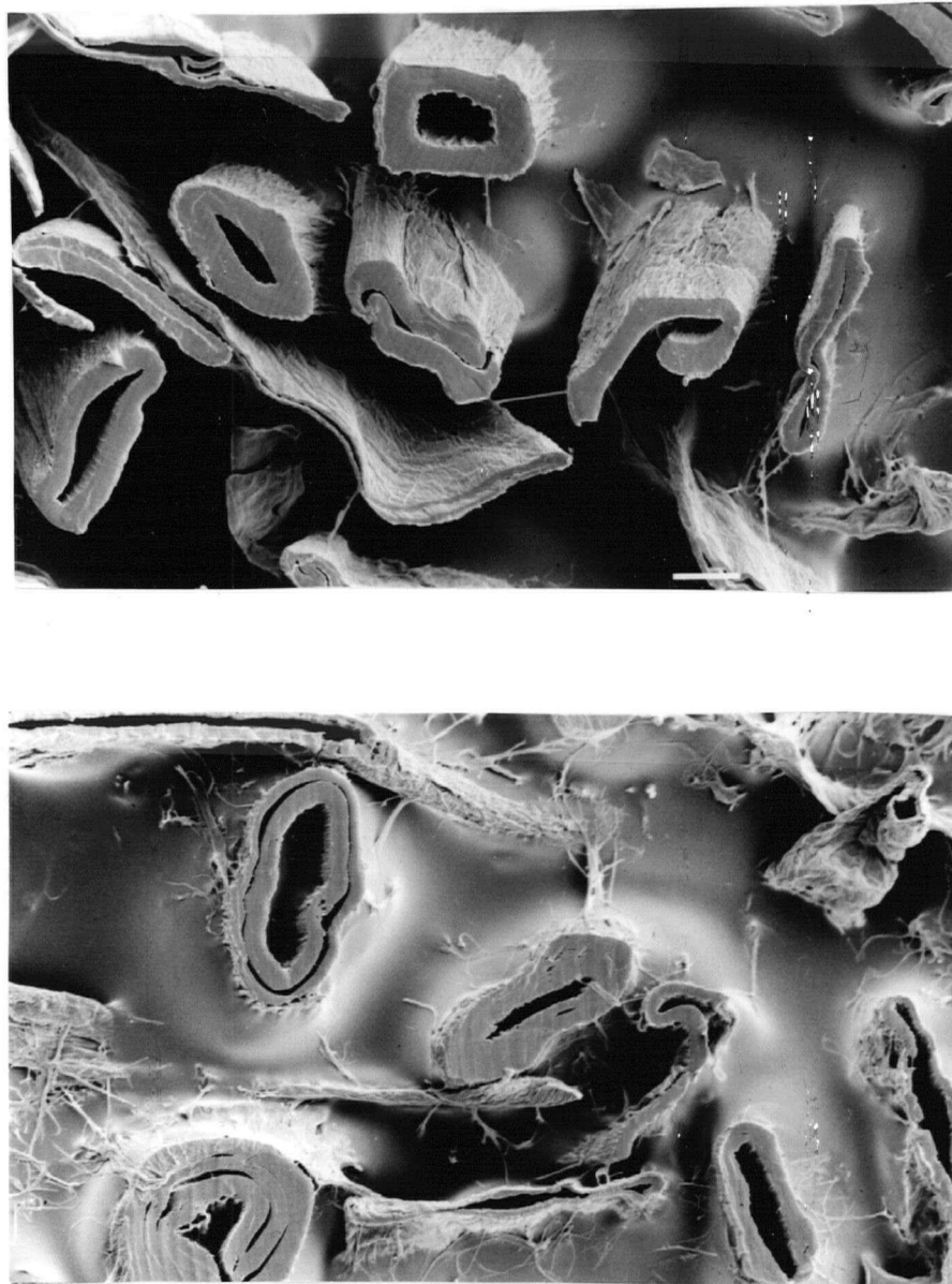
Figure 2.4: Internal fibrillation [Polan 1993] top - Unrefined chemical pulp 1 bottom - Chemical pulp after LC refining
