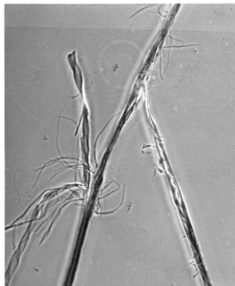
Figure 5.7: Examples of fibre damage (x100) a. Unraveled end b. Pulled back to a point
