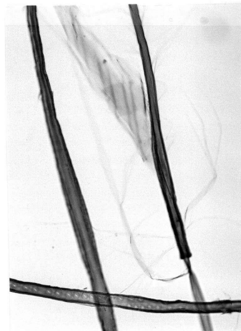
Figure 5.7: Examples of fibre damage (x100) a. Unraveled end b. Pulled back to a point
