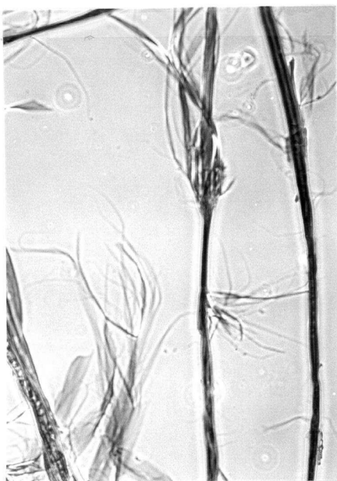
Figure 5.7: Examples of fibre damage (x100) c. Large fibre segments pulled back d. Sleeve condition
