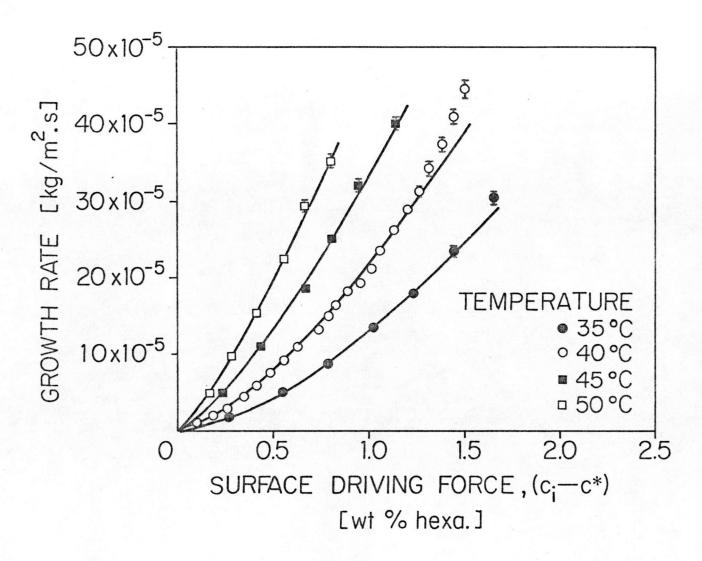
Figure 18 Apparent surface integration rates of 1.01 mm nickel sulfate  $\alpha$ -hexahydrate crystals at different temperatures. Bars show the 95% confidence limits when these extend beyond the point symbols
