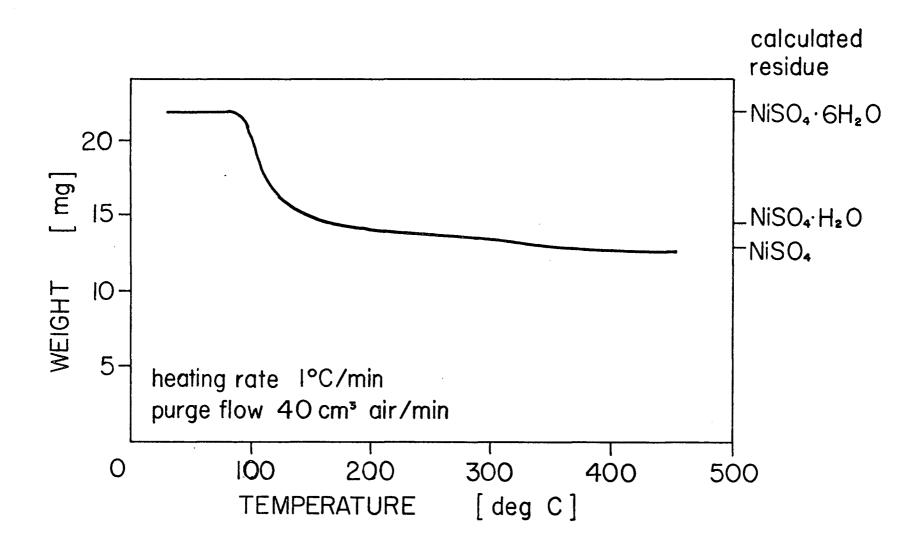
Figure 2 Thermogravimetric analysis of nickel sulfate  $\alpha$ -hexahydrate
