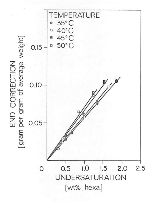
Figure L.4 Dissolution end corrections in the Batch Method for 1 mm crystals at different temperatures
