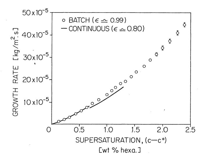
Figure 8 Growth rates of 1.01 mm nickel sulfate α-hexahydrate crystals at 40°C by the Batch and Continuous Methods. Bars show the 95% confidence limits when these extend beyond the point symbols
