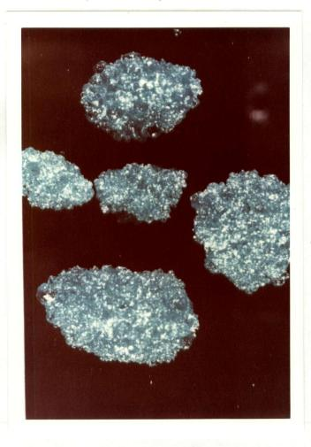
Figure G.1 Caked crystals, as received from the manufacturer
