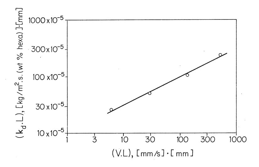
Figure 15 Mass transfer correlation of dissolution rate constant (k<sub>d</sub>) with solution velocity (V) and crystal size (L) at 40°C. The 95% confidence limits are all within the point symbols
