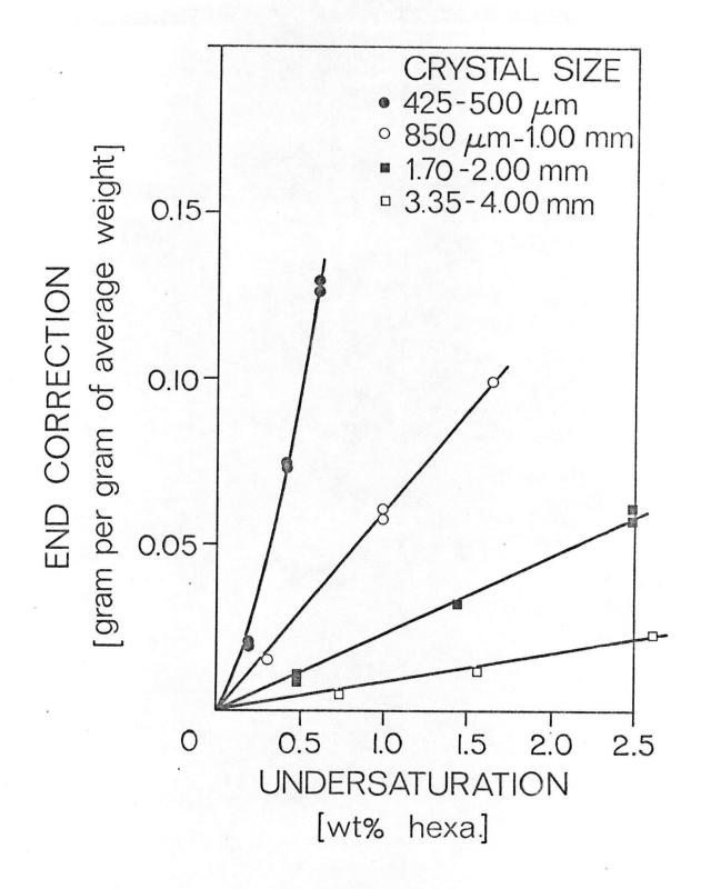
Figure L.3 Dissolution end corrections in the Batch Method for different sized crystals at 40°C
