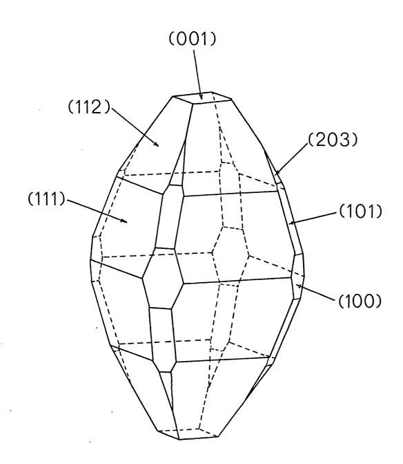
Figure J.1 Idealized shape of nickel sulfate  $\alpha$ -hexahydrate crystals
