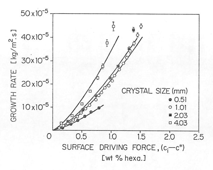
Figure 17 Apparent surface integration rates of different sized nickel sulfate α-hexahydrate crystals at 40°C. Bars show the 95% confidence limits when these extend beyond the point symbols
