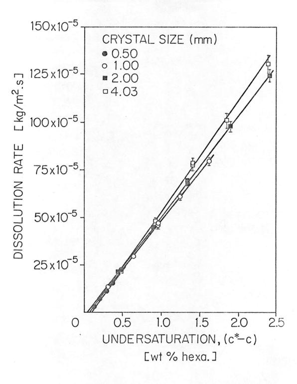
Figure 13 Dissolution rates by Batch Method of different sized nickel sulfate  $\alpha$ -hexahydrate crystals at 40°C. Bars show the 95% confidence limits when these extend beyond the point symbols
