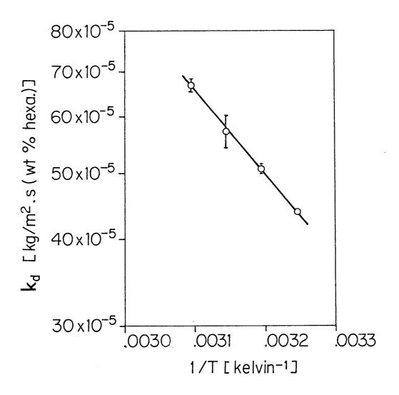
Figure 16 Arrhenius plot of dissolution rate constants for 1.00 mm crystals. Bars show the 95% confidence limits when these extend beyond the point symbols
