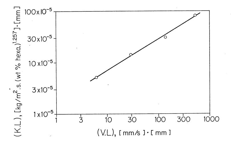
Figure 10 Pseudo-mass transfer correlation of overall growth rate constant (K) with interstitial solution velocity (V) and crystal size (L) at 40°C
