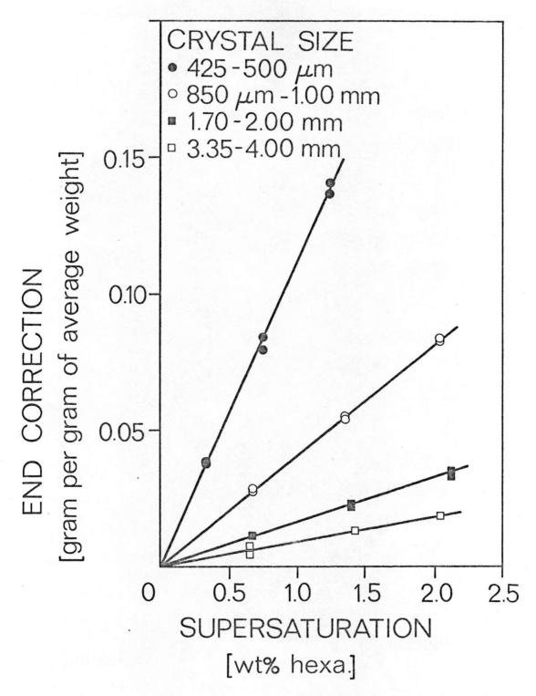
Figure L.1 Growth end corrections in the Batch Method for different sized crystals at  $40^{\circ}\mathrm{C}$
