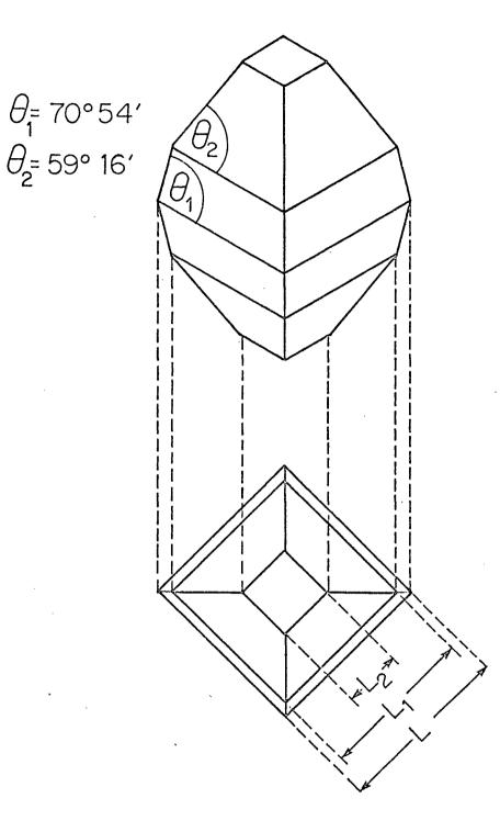
Figure J.2 Simplified shape of nickel sulfate  $\alpha$ -hexahydrate crystals
