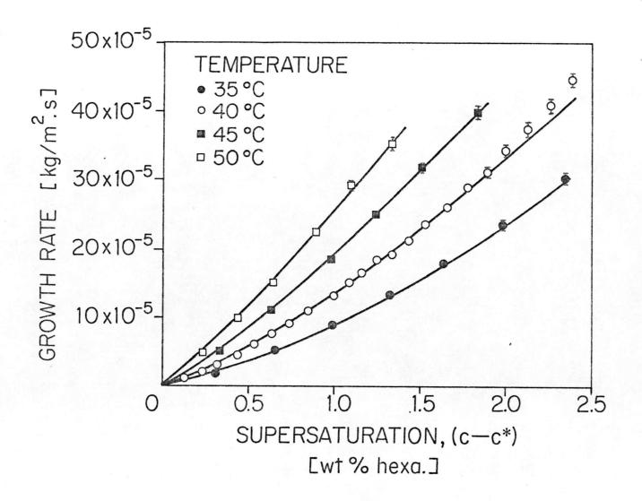
Figure 7 Growth rates by Batch Method of 1.01 mm nickel sulfate α-hexahydrate crystals at different temperatures. Bars show the 95% confidence limits when these extend beyond the point symbols
