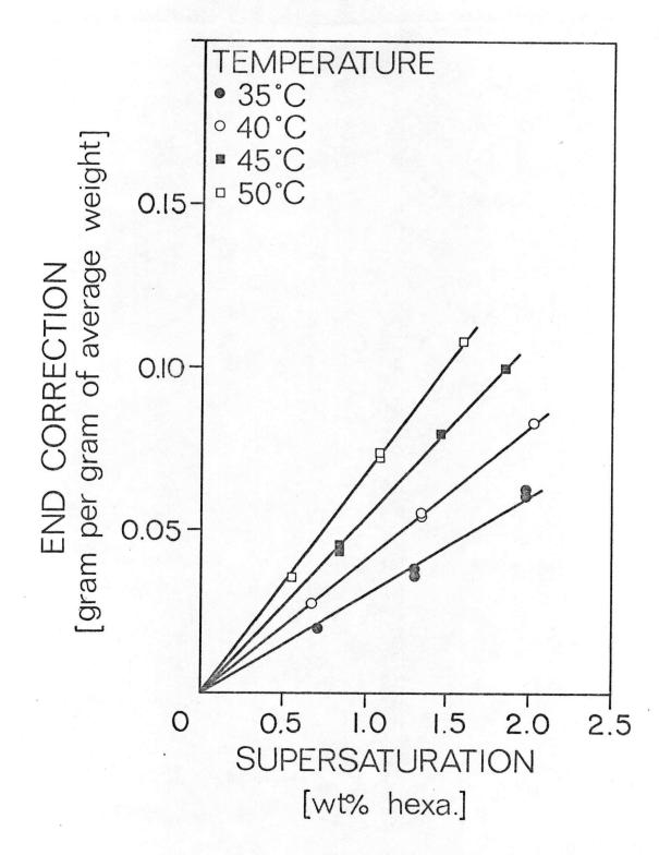
Figure L.2 Growth end corrections in the Batch Method for 1 mm crystals at different temperatures
