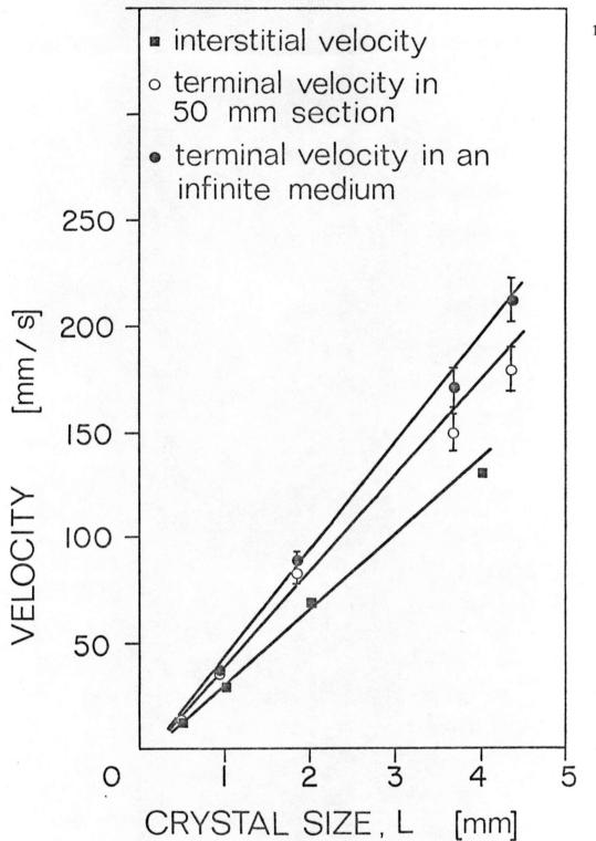
Figure D.1 Interstitial solution velocities during the Batch Method and single crystal terminal velocities, for different crystal sizes at 40°C. Bars show the 95% confidence limits when these extend beyond the point symbols
