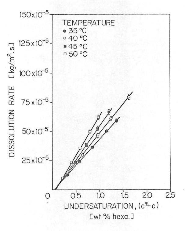
Figure 14 Dissolution rates by Batch Method of 1.00 mm nickel sulfate α-hexahydrate crystals at different temperatures. Bars show the 95% confidence limits when these extend beyond the point symbols
