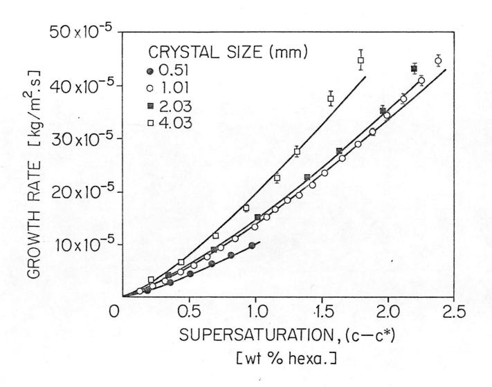
Figure 6 Growth rates by Batch Method of different sized nickel sulfate  $\alpha$ -hexahydrate crystals at 40°C. Bars show the 95% confidence limits when these extend beyond the point symbols
