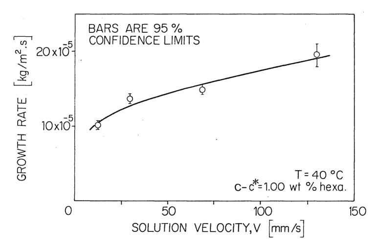
Figure 12 Apparent dependence of growth rate on crystal/solution relative velocity (interstitial solution velocity), V, in a fluidized bed
