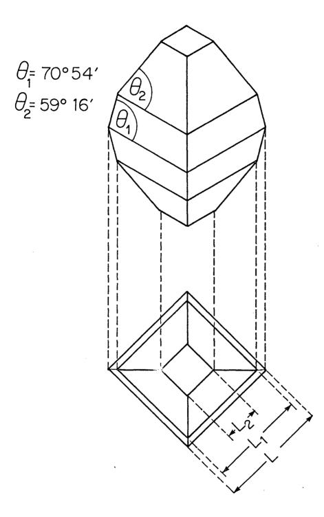
Figure 1 Simplified shape of nickel sulfate α-hexahydrate crystals
