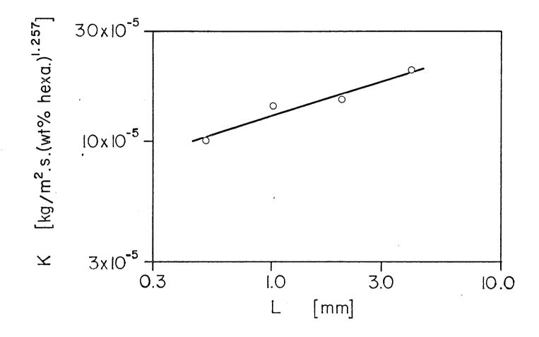
Figure 9 Logarithmic plot of overall growth rate constant (K) against crystal size (L) to find the exponent b'
