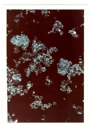
Figure G.2 Crystals from the manufacturer after partial decaking with a pestle
