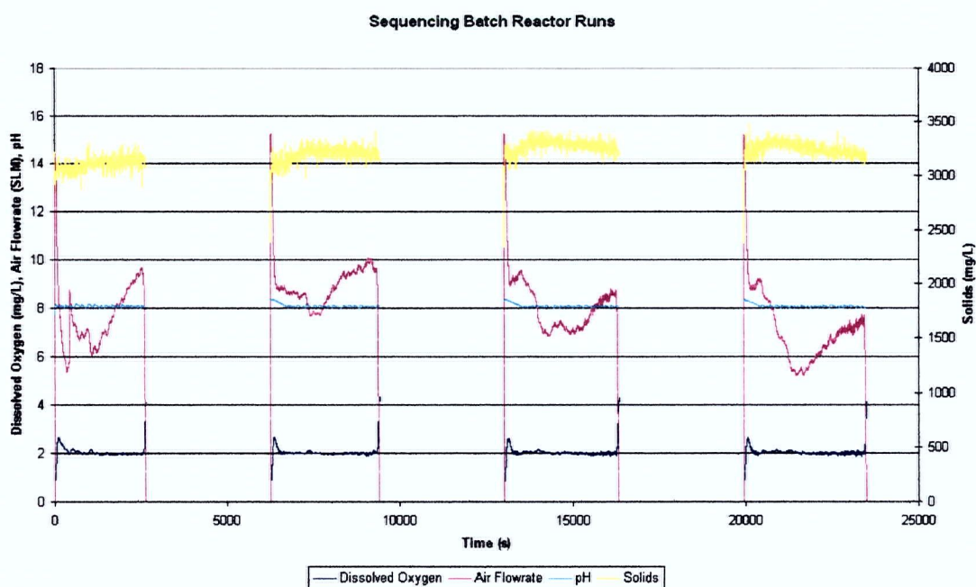
Figure 5.10 - A typical sequencing batch reactor run.
